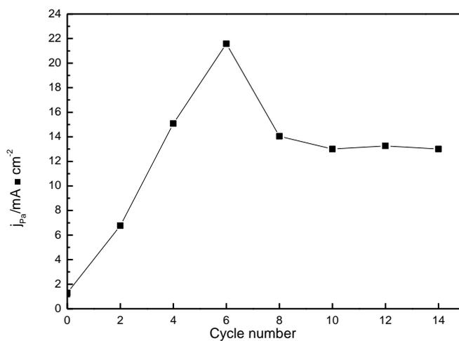
**Figure 4.** Effect of the thickness of the film on peak current density of methanol oxidation
