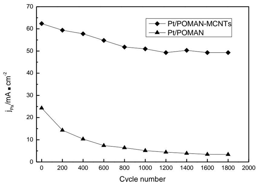
**Figure 7.** Long-term stability of the electrodes in 1mol/LHCHO and 0.5mol/LH<sub>2</sub>SO<sub>4</sub> (Scan rate: 10mV/s)
