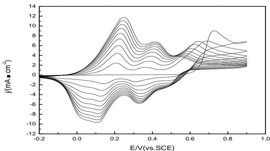
**Figure 1.** Cyclic voltammograms of 2-methoxyaniline (MCNTs) electrochemical polymerization on Pt electrode
