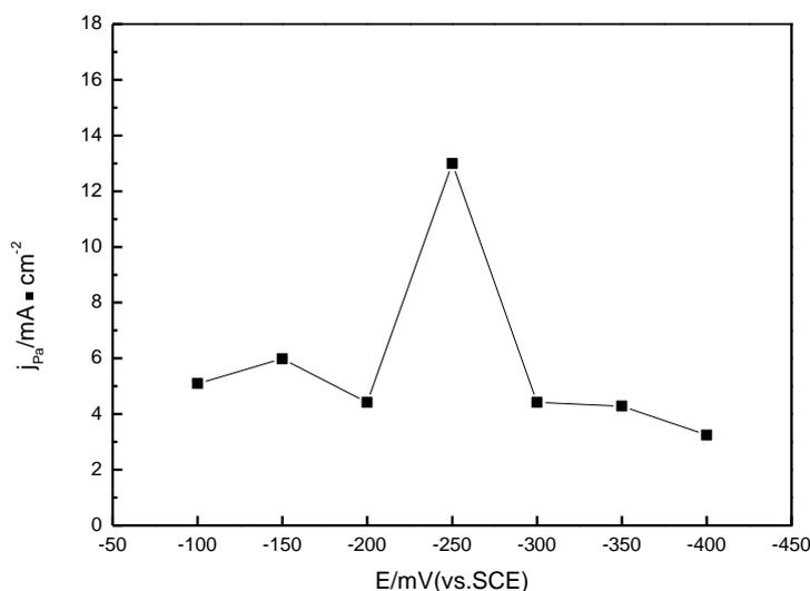
**Figure 5.** Effect of deposition potential on peak current density of methanol oxidation
