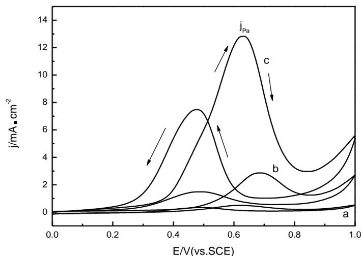
**Figure 3.** Cyclic voltammograms of methanol oxidation on POMAN(a), Pt/POMAN (b) and Pt/POMAN-MCNT (c) film electrodes
