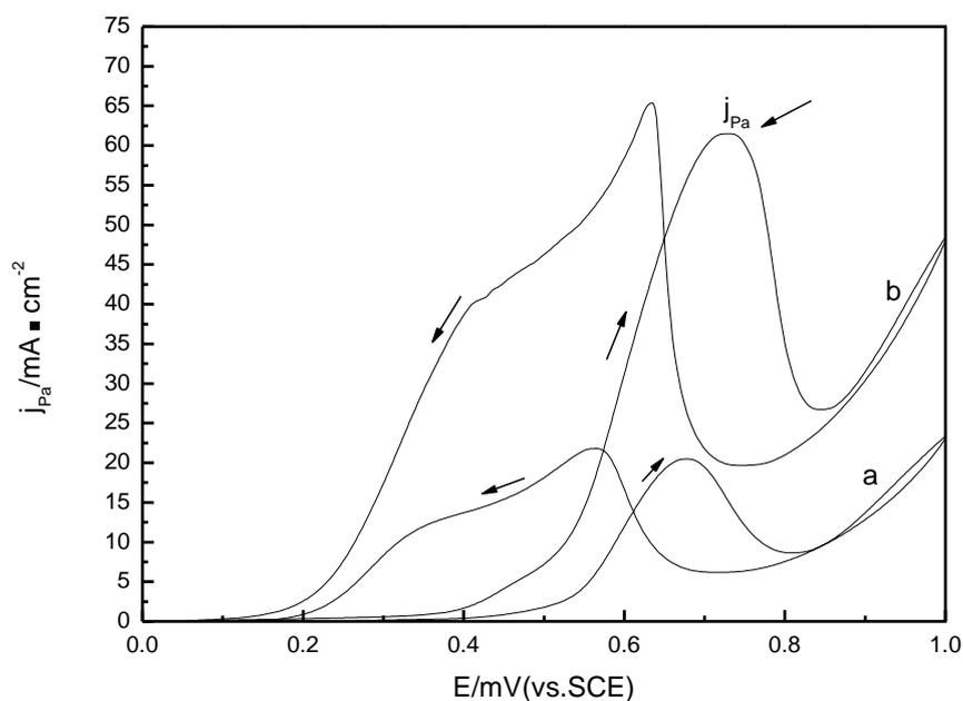
**Figure 6.** The potential cyclic voltammograms of electrooxidation of formaldehyde at (a) Pt-modified POMAN film electrode and (b) Pt-modified POMAN-MCNTs composite film electrode in 1 mol/L HCHO and 0.5 mol/L  $\text{H}_2\text{SO}_4$ (vs.SCE)
