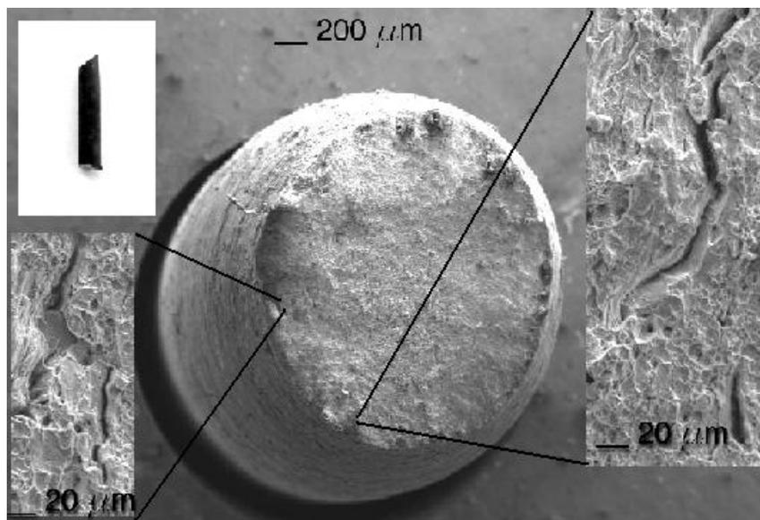
**Figure 8.** Steel SSRT longitudinal specimen fractured in NS-4 solution
