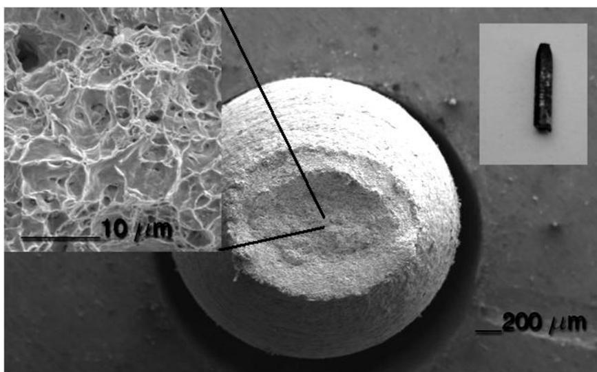
**Figure 6.** SSRT steel longitudinal specimens hydrogen precharged and fractured in air.
