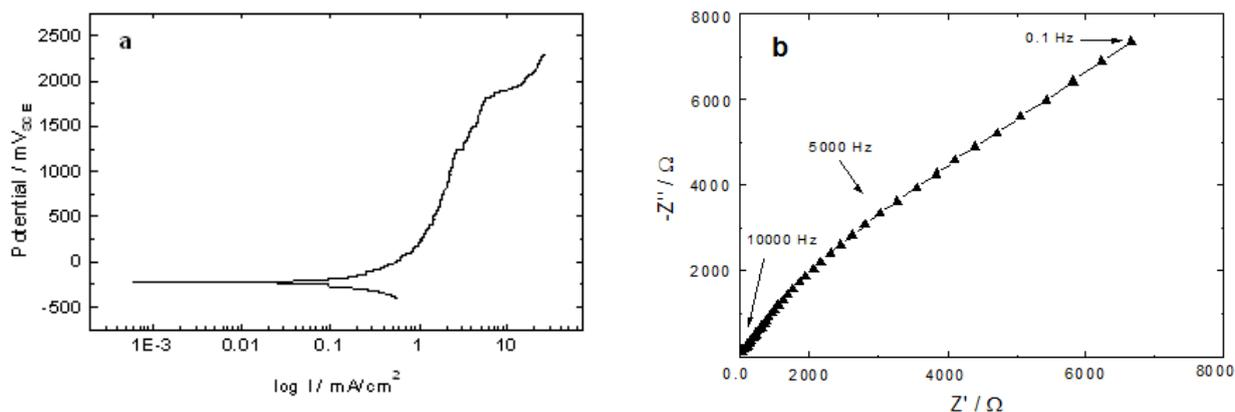
**Figure 2.** Electrochemical corrosion steel behavior in NS-4 test solution, (a)polarization curves and (b) EIS Nyquist plot.
