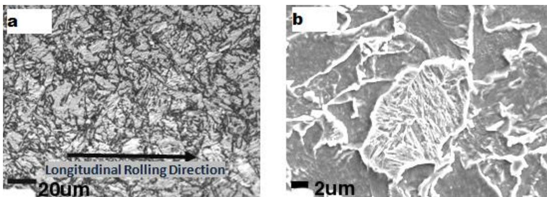
**Figure 1.** Microalloyed Pipeline Steel Plate Microstructure. a) Optical and b) SEM microphotographies.
