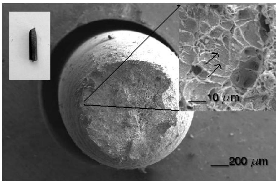
**Figure 7.** Steel SSRT transversal specimen fractured in NS-4 solution
