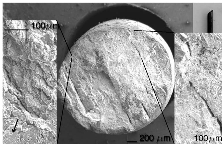
**Figure 10.** Fractography and steel sample test profile in the transversal direction at the NS4-H solution condition.
