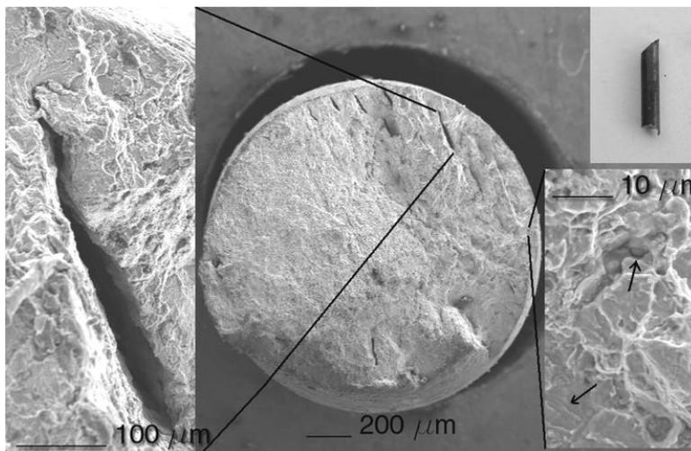
**Figure 9.** Fractography and steel sample test profile in the longitudinal direction at the NS4-H
