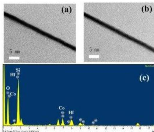
**Figure 2.** Cross-sectional TEM images of  $\text{Co}_x\text{Hf}_y\text{Si}_z\text{O}$  high- $\kappa$  thin film (a) before and (b) after  $\text{O}_2$  plasma treatment. (c) EDS spectrum of the plasma treated  $\text{Co}_x\text{Hf}_y\text{Si}_z\text{O}$  high- $\kappa$  thin film.
