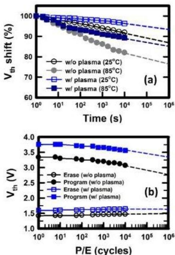
**Figure 6.** (a) Charge retention and (b) endurance characteristics of the high- $\kappa$  memories with and without  $\text{O}_2$  plasma treatment.
