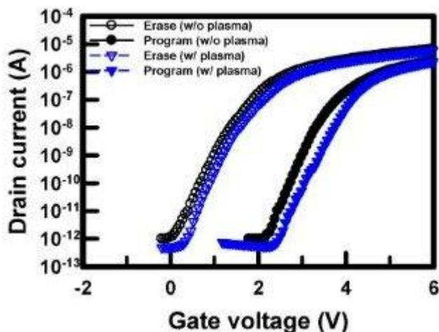
**Figure 4.** I<sub>d</sub>-V<sub>g</sub> characteristics of the high-κ memories with and without O<sub>2</sub> plasma treatment in fresh and program states, respectively.
