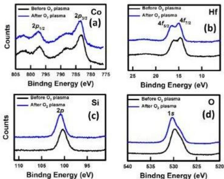
**Figure 3.** (a) Co  $2p$ , (b) Hf  $4f$ , (c) Si  $2p$ , and (d) O  $1s$  spectra of the sol-gel derived  $\text{Co}_x\text{Hf}_y\text{Si}_2\text{O}$  high- $\kappa$  film before and after  $\text{O}_2$  plasma treatment.
