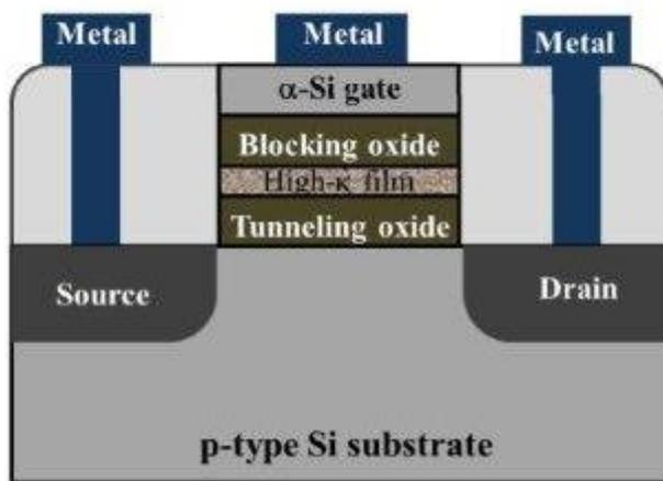
**Figure 1.** Schematic diagram of high- $\kappa$  flash memory.
