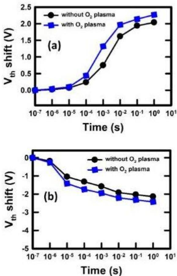
**Figure 5.** (a) Program and (b) erase speeds of the Co<sub>x</sub>Hf<sub>y</sub>Si<sub>z</sub>O high-κ memories.
