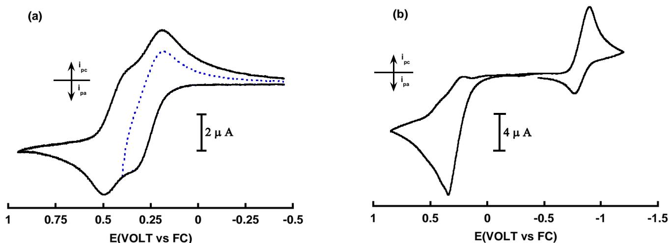
**Figure 4.** (a) Cyclic voltammograms of 2.25 mM **1** in  $\text{CH}_2\text{Cl}_2$ /0.05 M  $[\text{NBu}_4][\text{B(C}_6\text{F}_5)_4]$  at scan rate of 500 mV/s, 1 mm GC disk electrode. (b) Cyclic voltammograms recorded under same conditions as in (a) but after addition of 1 equiv  $\text{P(OMe)}_3$  ligand.
