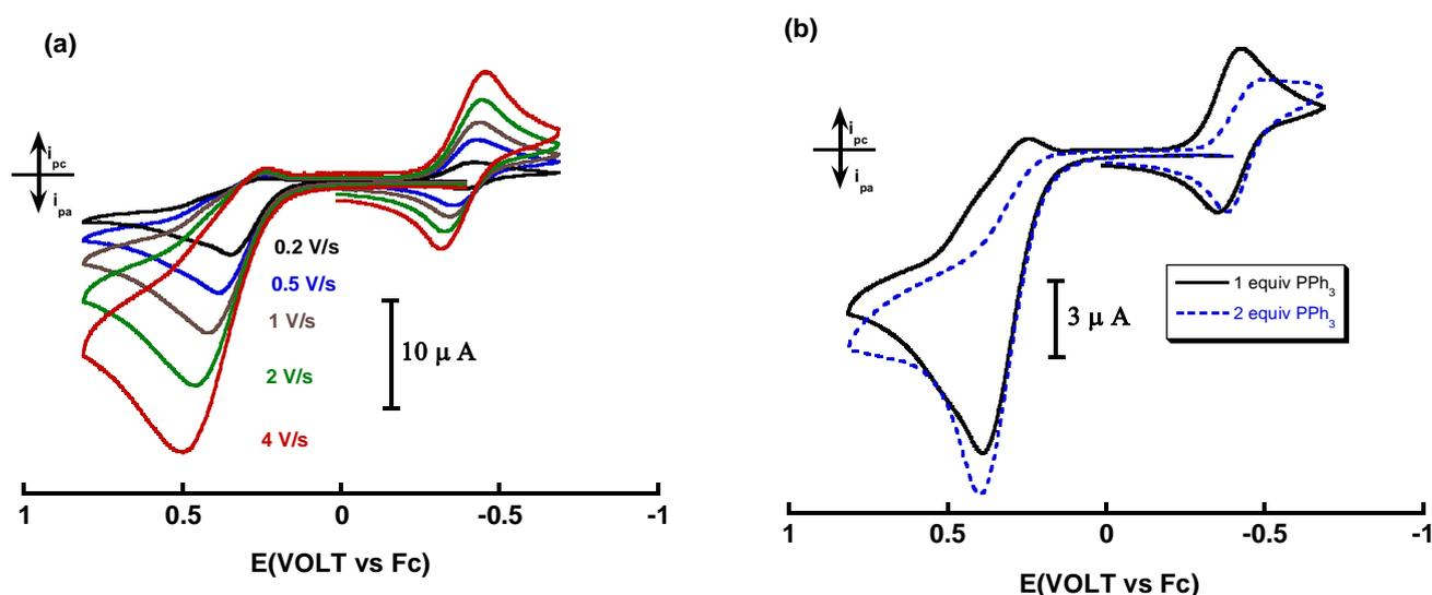
**Figure 2.** (a) Cyclic voltammograms obtained at different scan rates with 1 mm GC disk electrode for 1.55 mM **1** in CH<sub>2</sub>Cl<sub>2</sub>/0.05 M [NBu<sub>4</sub>][B(C<sub>6</sub>F<sub>5</sub>)<sub>4</sub>] in the presence of 1 equiv PPh<sub>3</sub> at 298K. (b) CVs of 1.55 mM **1** in CH<sub>2</sub>Cl<sub>2</sub>/0.05 M [NBu<sub>4</sub>][B(C<sub>6</sub>F<sub>5</sub>)<sub>4</sub>] in the presence of 1 and 2 equiv of PPh<sub>3</sub> at scan rate of 500 mV/s, 298K using 1 mm GC disk.
