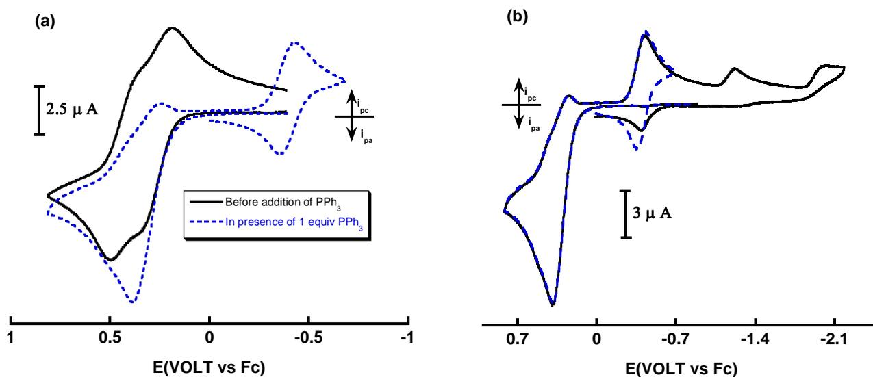
**Figure 1.** (a) Cyclic voltammograms of 1.55 mM **1** in  $\text{CH}_2\text{Cl}_2/0.05 \text{ M } [\text{NBu}_4][\text{B}(\text{C}_6\text{F}_5)_4]$  at scan rate of 500 mV/s, 298K and 1 mm GC disk electrode, before (black curve) and after (blue curve) addition of 1 equiv of  $\text{PPh}_3$ . (b) CVs under the same conditions but at different switching potentials.
