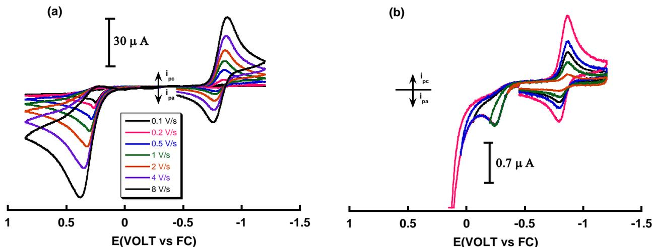
**Figure 5.** (a) Cyclic voltammograms of 2.25 mM **1** in  $\text{CH}_2\text{Cl}_2/0.05$  M  $[\text{NBu}_4][\text{B}(\text{C}_6\text{F}_5)_4]$  and 1 equiv  $\text{P}(\text{OMe})_3$  at different scan rates, 1 mm GC disk electrode. (b) Cyclic voltammograms obtained under same condition as in (a), but at different switching potentials and scan rate of 500 mV/s
