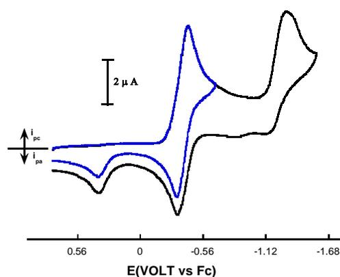
**Figure 3.** Cyclic voltammograms of the electrolysis products of 1.55 mM  $\mathbf{1}$  in the presence of 2 equiv  $\text{PPh}_3$  in  $\text{CH}_2\text{Cl}_2/0.05 \text{ M } [\text{NBu}_4][\text{B}(\text{C}_6\text{F}_5)_4]$  at scan rate of 100 mV/s, 273 K, using 1 mm GC disk electrode.
