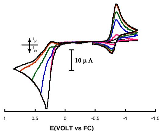
**Figure 6.** Cyclic voltammograms as at different switching potentials obtained for 2.25 mM **1** in  $\text{CH}_2\text{Cl}_2/0.05 \text{ M } [\text{NBu}_4][\text{B}(\text{C}_6\text{F}_5)_4]$  in the presence of 1 equiv of  $\text{P}(\text{OMe})_3$  at scan rate of 500 mV/s using 1 mm GC disk electrode.
