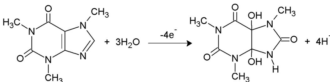
**Figure 1.** Mechanism of overall oxidation of CAF [34,54]
