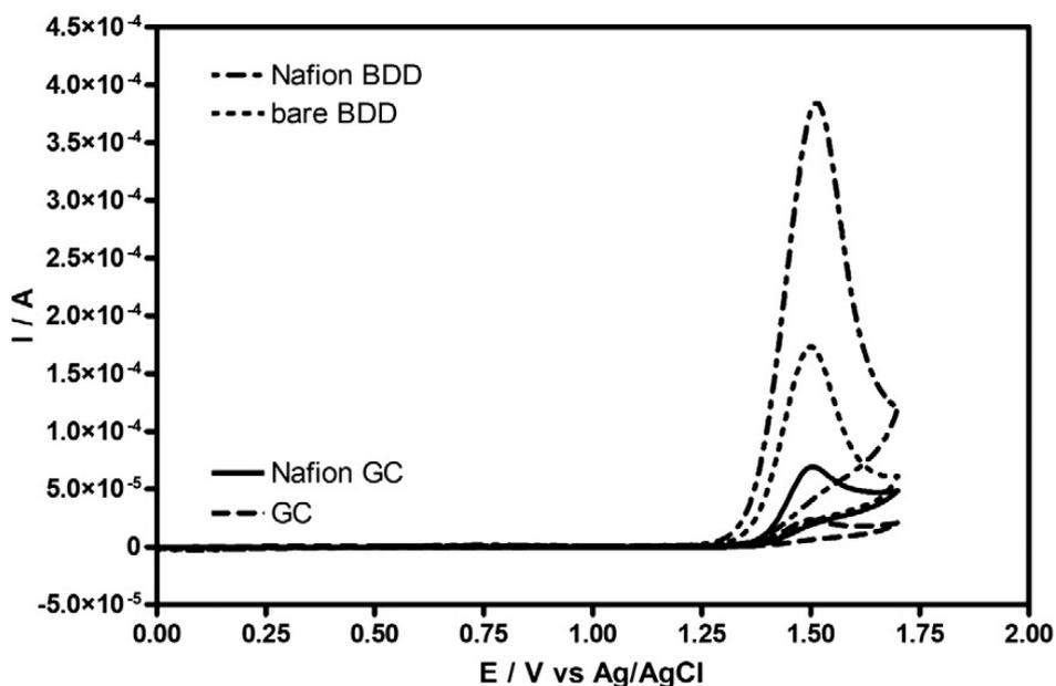
**Figure 3.** Cyclic voltammograms recorded on bare and Nafion-modified GCE and BDDE; 100  $\mu\text{L}$  of 0.1 M CAF in 30 mL of 0.2 M  $\text{H}_2\text{SO}_4$  solution (scan rate: 100  $\text{mV s}^{-1}$ ) [35].
