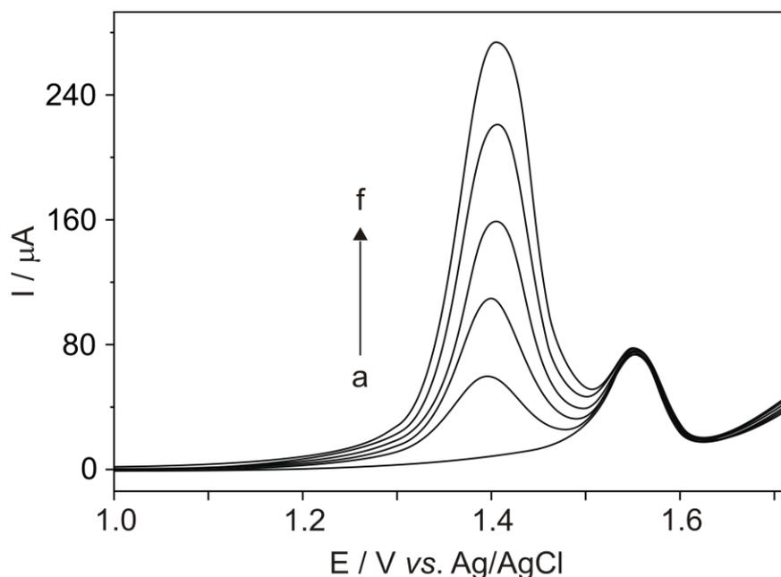
**Figure 2.** DP voltammograms of 10  $\mu\text{M}$  CAF (fixed concentration) and different THO concentrations: (a) 0, (b) 20, (c) 40, (d) 60, (e) 80 and (f) 100  $\mu\text{M}$  (supporting electrolyte 0.4 M  $\text{HClO}_4$ ) on bare BDDE at optimized DPV parameters: modulation amplitude of 0.05 V, modulation time 0.02 s and scan rate 0.05  $\text{V s}^{-1}$  [56].
