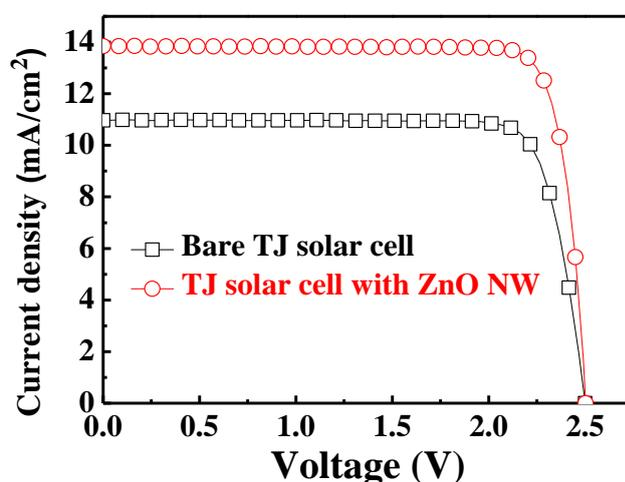
**Figure 2.** The illuminated (AM of 1.5 G) I-V characteristics of the bare TJ solar cell and TJ solar cell with a ZnO NW design under  $100 \text{ mW/cm}^2$  illumination.
