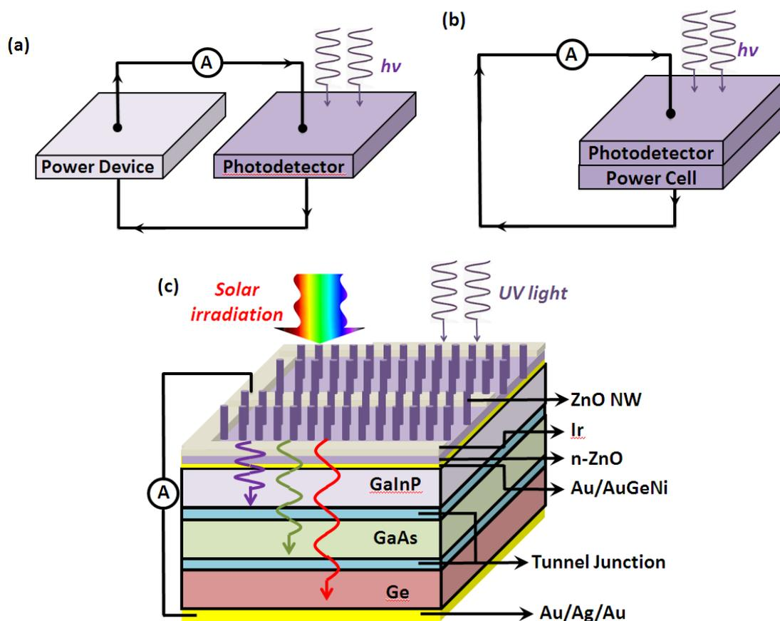
**Figure 1.** Schematic diagrams of (a) the planar and separated self-powered UV detection design, (b) the vertical and integrated self-powered UV detection design, and (c) the fabricated UV PD integrated with the triple-junction (TJ) solar cell.
