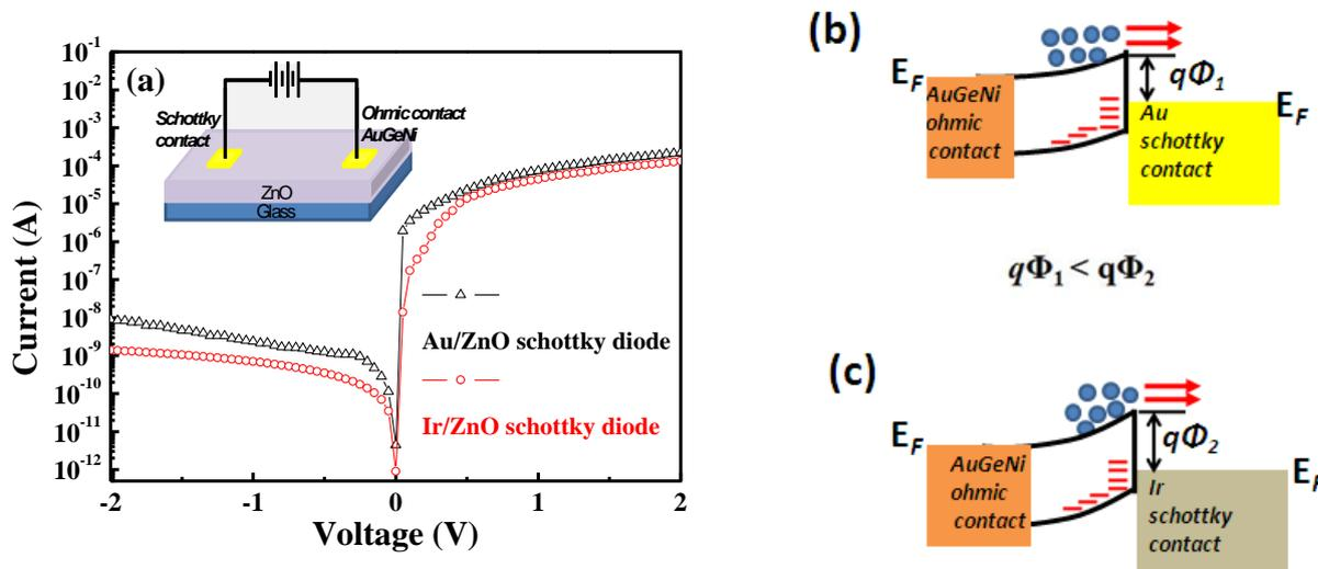
**Figure 3.** (a) Room-temperature I-V characteristics of the metal–semiconductor contact on the SiO<sub>2</sub> substrate and the schematic illustration of the Schottky diode behaviors of the (b) Ir/ZnO and (c) Au/ZnO structures.
