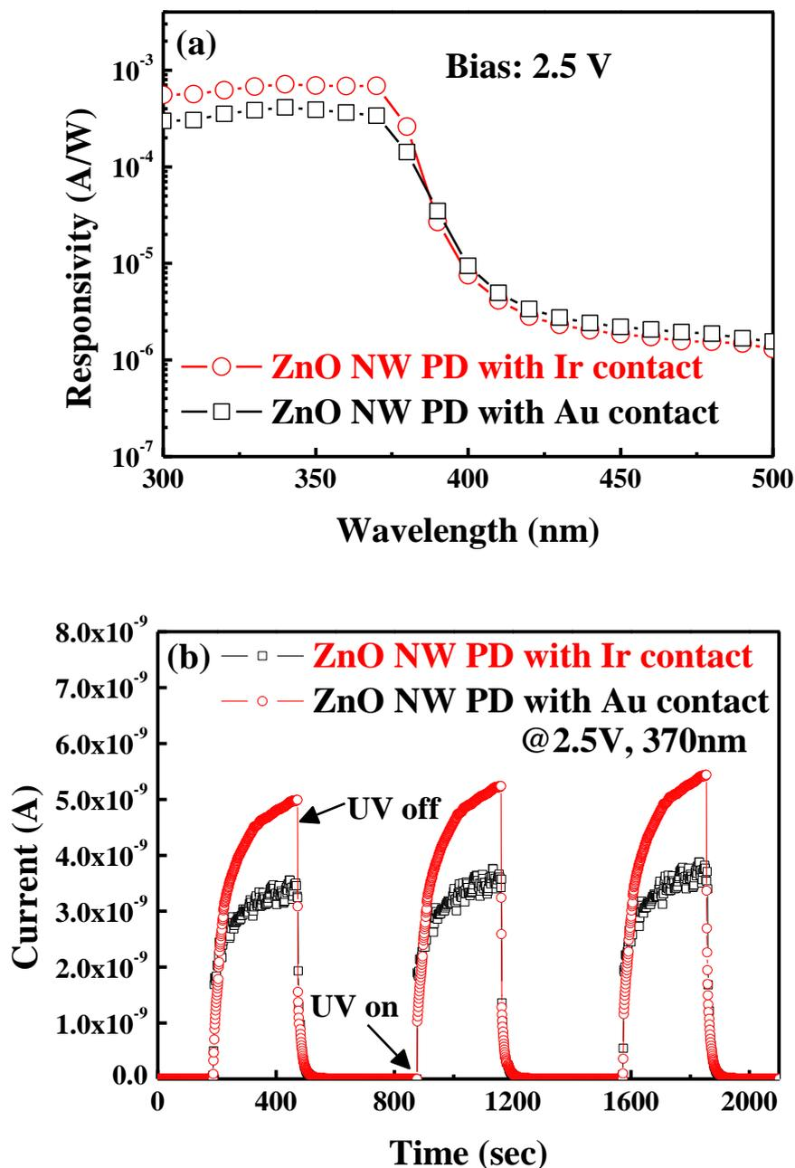
**Figure 4.** (a) Room-temperature spectral responses of the fabricated ZnO NW PDs with Ir and Au electrodes and (b) transient response of the fabricated ZnO NW PDs with Ir and Au electrodes as the UV excitation was switched on and off
