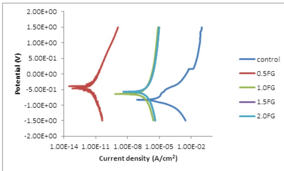
**Figure 4.** Linear polarization of mild steel in 3.5% NaCl solution /ferrous gluconate environment at 28<sup>o</sup>C.
