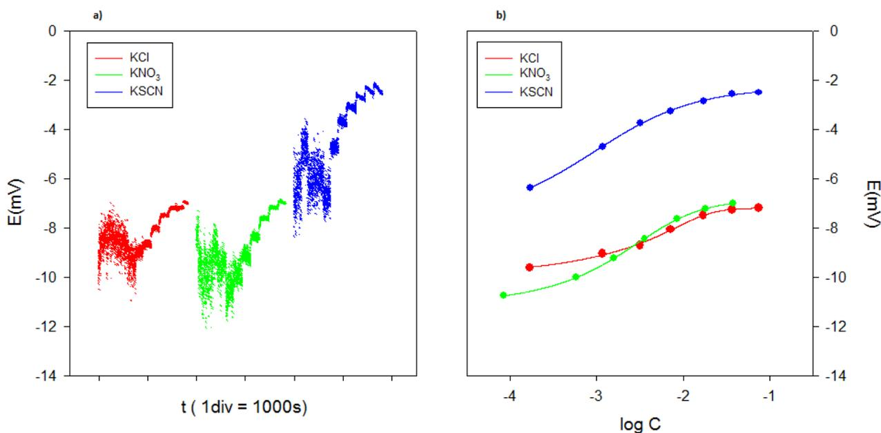
**Figure 4.** (a) Dynamic response of the  $[bmim^+][PF_6^-]$  (67 % wt.) membrane to increasing concentrations of  $Cl^-$ ,  $NO_3^-$  and  $SCN^-$  anions. (b) Corresponding calibration graphs for the electrode.
