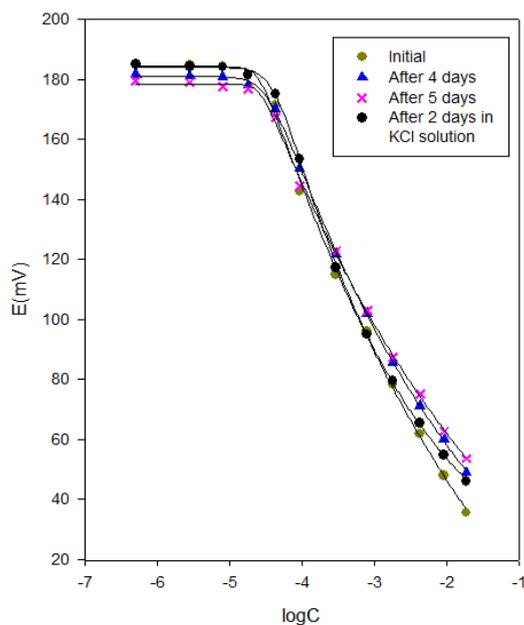
**Figure 8.** Calibration graphs for the ibuprofen anion response of the [thtdP<sup>+</sup>][Cl<sup>-</sup>] (20 % wt.) membrane after 1, 4 and 5 days in water and after 2 days in 0.1M KCl solution.
