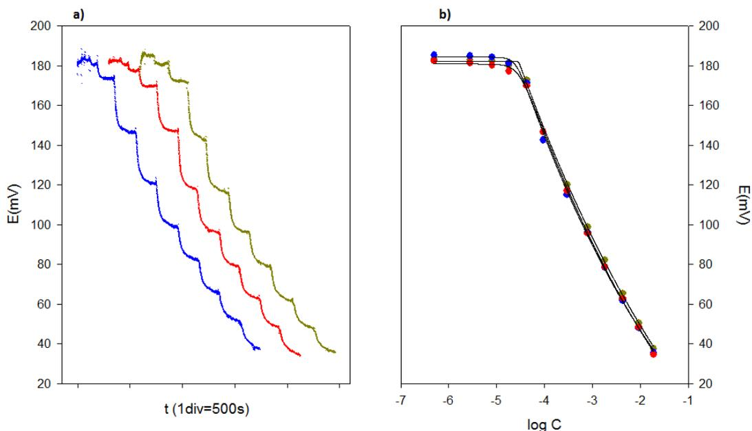
**Figure 7.** a) Dynamic response of the [thtdP<sup>+</sup>][Cl<sup>-</sup>] (20 % wt.) membrane to increasing concentrations of ibuprofen. (b) Corresponding calibration graphs for the electrode.
