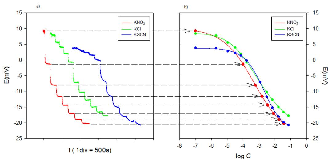
Figure 2. (a) Dynamic response of the [bmim<sup>+</sup>][PF<sub>6</sub><sup>-</sup>] (20 % wt.) membrane to increasing concentrations of NO<sub>3</sub><sup>-</sup>, Cl<sup>-</sup> and SCN<sup>-</sup> anions. (b) Corresponding calibration graphs for the electrode.
