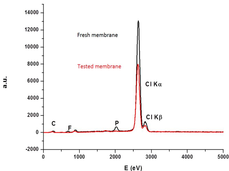
**Figure 3.** EDX spectra of [bmim<sup>+</sup>][PF<sub>6</sub><sup>-</sup>] (20 % wt.) membrane, fresh and after exposure to NO<sub>3</sub><sup>-</sup>, Cl<sup>-</sup> and SCN<sup>-</sup> anions.
