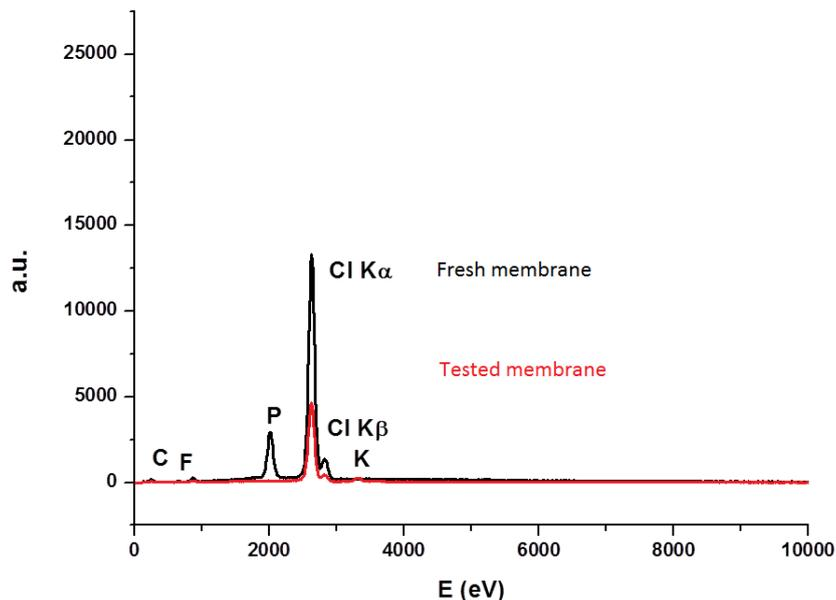
**Figure 5.** EDX spectra of  $[\text{bmim}^+][\text{PF}_6^-]$  (67 % wt.) membrane, fresh and after exposure to  $\text{Cl}^-$ ,  $\text{NO}_3^-$  and  $\text{SCN}^-$  anions.
