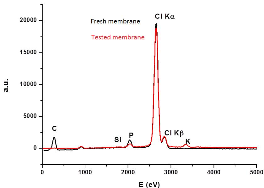
**Figure 10.** EDX spectra of [thtdP<sup>+</sup>][Cl<sup>-</sup>] (20 % wt.) membrane, fresh and after potentiometric responses to SCN<sup>-</sup>, NO<sub>3</sub><sup>-</sup>, and Cl<sup>-</sup> and ibuprofen anions, internal side.
