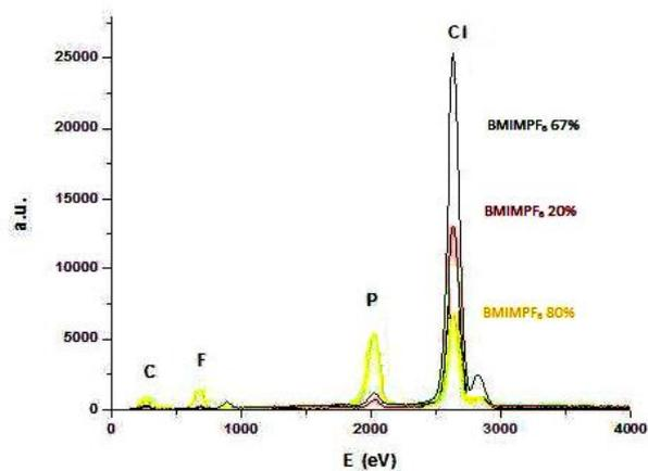
Figure 1. EDX spectra of fresh membranes with [bmim<sup>+</sup>][PF<sub>6</sub><sup>-</sup>] 67, 20 and 80 % wt.
