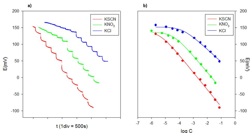
**Figure 6.** (a) Dynamic response of the  $[\text{thtdP}^+][\text{Cl}^-]$  (20 % wt.) membrane to increasing concentrations of  $\text{SCN}^-$ ,  $\text{NO}_3^-$ , and  $\text{Cl}^-$  anions. (b) Corresponding calibration graphs for the electrode.
