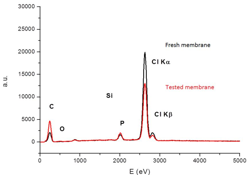
**Figure 9.** EDX spectra of [thtdP<sup>+</sup>][Cl<sup>-</sup>] (20 % wt.) membrane, fresh and after exposure to SCN<sup>-</sup>, NO<sub>3</sub><sup>-</sup>, and Cl<sup>-</sup> and ibuprofen anions, external side.
