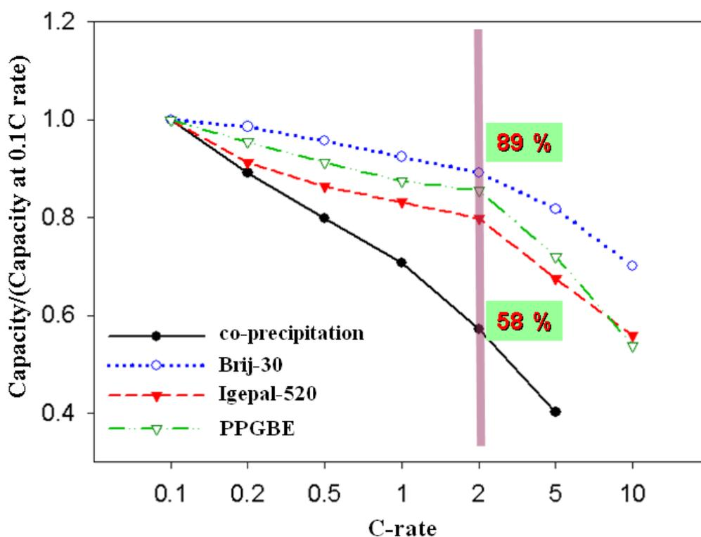
**Figure 10.** Relative specific capacity of LiFePO<sub>4</sub>/C with various surfactants at variable C-rate.
