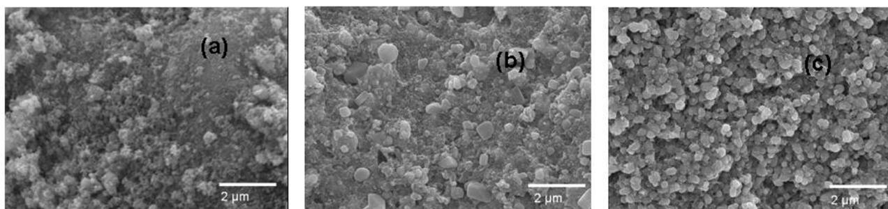
**Figure 5.** SEM images of  $\text{LiFePO}_4/\text{C}$  (a)Brij-30; (b) Igepal-520, (c) PPGBE.
