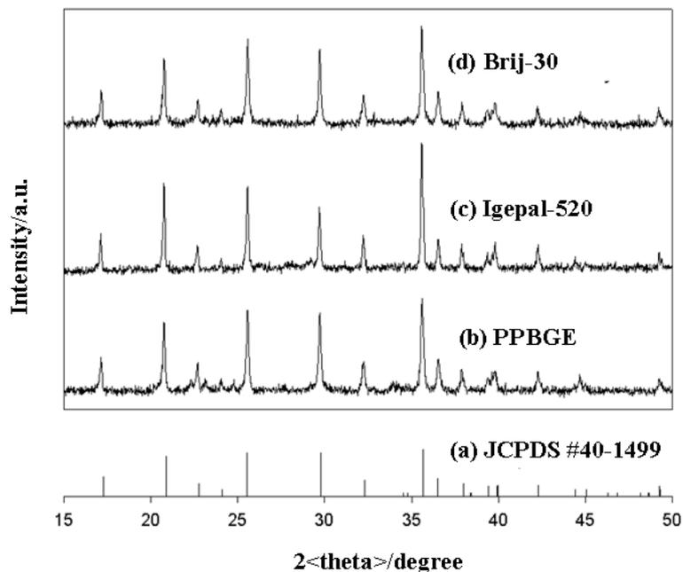
**Figure 3.** X-ray diffraction patterns of (a) theoretical  $\text{LiFePO}_4$  (JCPDS card no.40-1499)); (b) PPGBE; (c) Igepal-520; (d) Brij-30.
