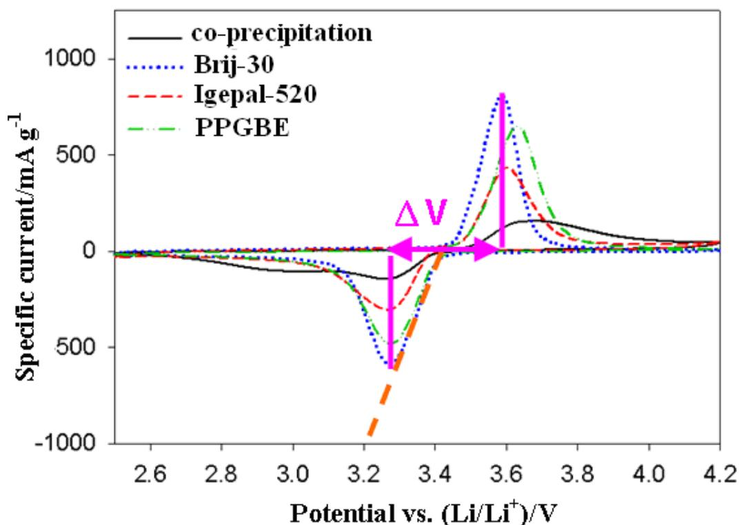
**Figure 6.** Cyclic voltammetry profile of the third cycle for LiFePO<sub>4</sub>/C prepared with various surfactants
