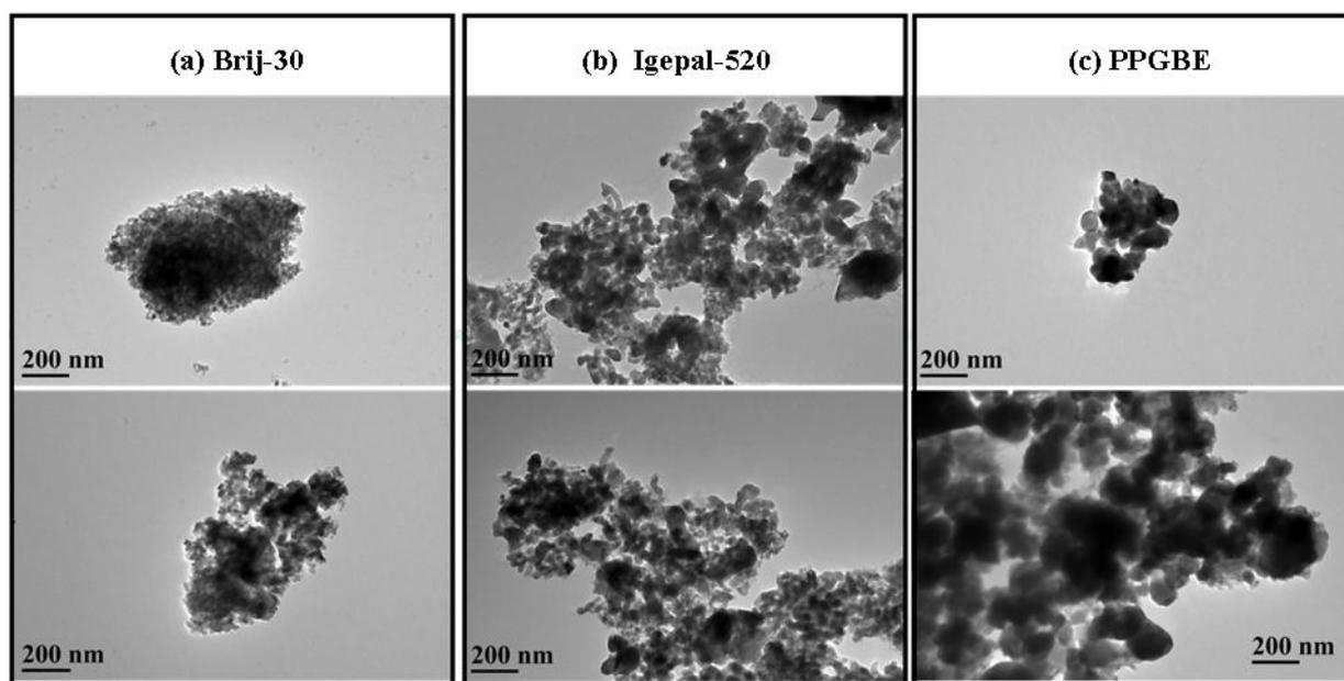
**Figure 4.** TEM images of  $\text{LiFePO}_4/\text{C}$  (a)Brij-30; (b) Igepal-520, (c) PPGBE.
