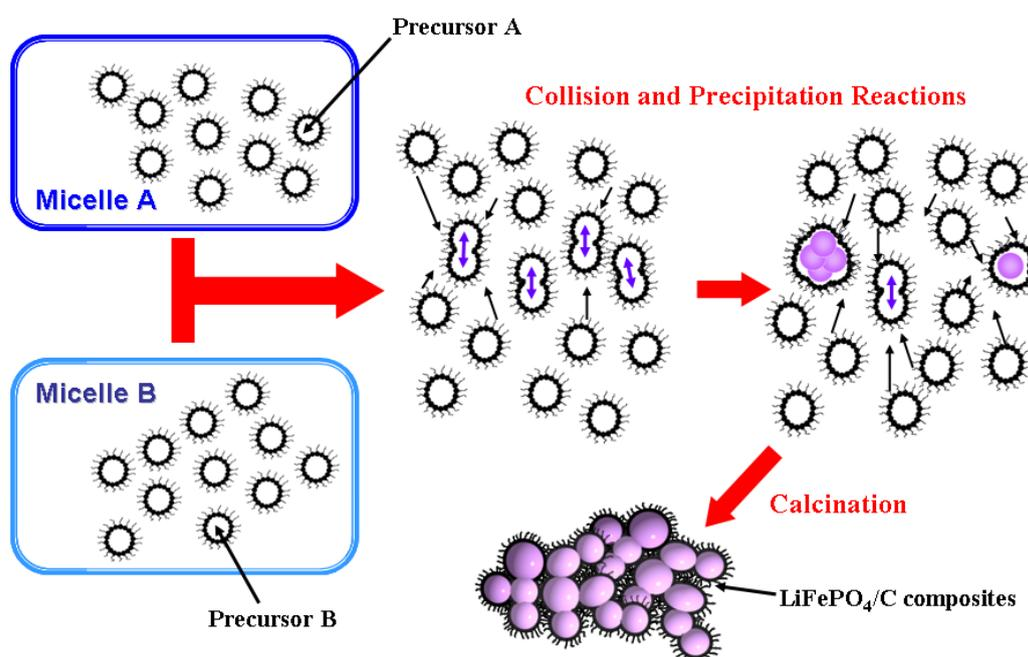
**Figure 1.** Schematic illustration of the precipitation method between two reverse-emulsion solutions.
