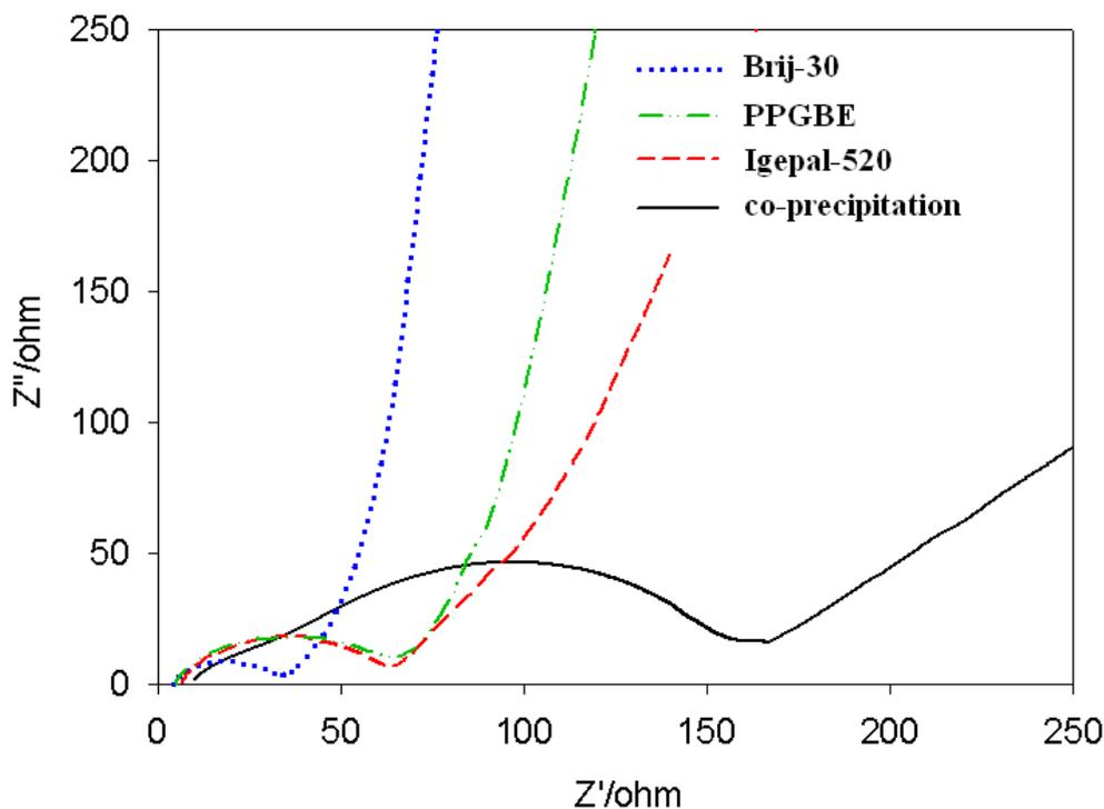
**Figure 7.** AC impedance spectroscopy for  $\text{LiFePO}_4/\text{C}$  prepared with various surfactants.
