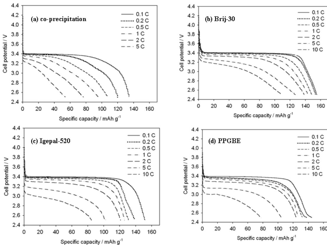
**Figure 9.** Discharge curves of LiFePO<sub>4</sub>/C prepared with various surfactants at variable C-rate.
