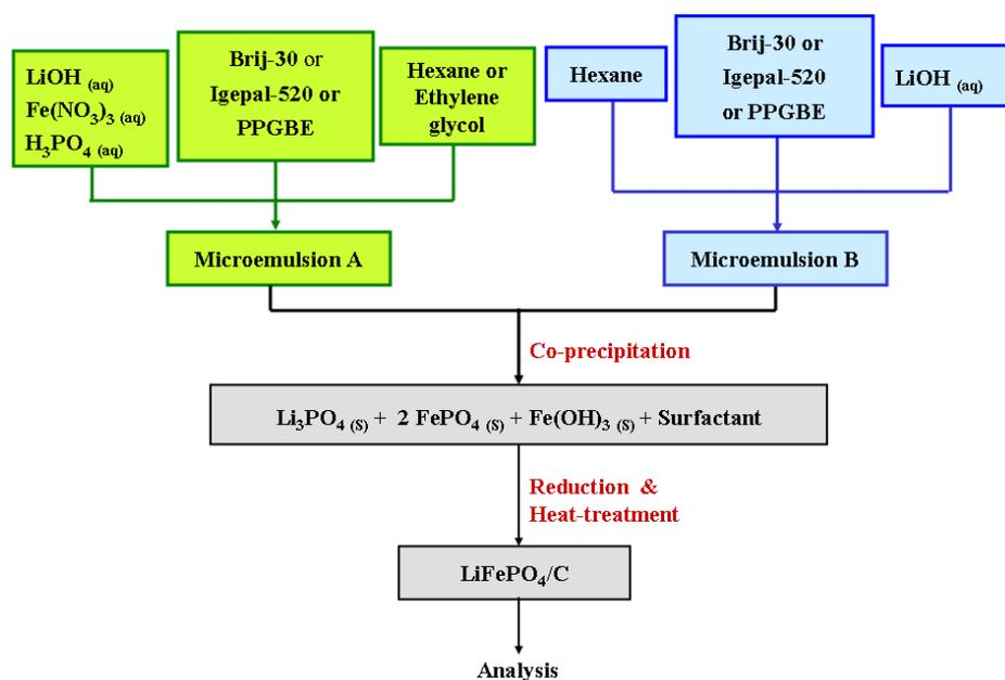
**Figure 2.** Flowchart for preparing  $\text{LiFePO}_4/\text{C}$  powder by the precipitation method between two microemulsion solutions.
