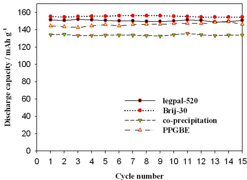
**Figure 8.** Discharge capacities vs. cycle number at 0.1C rate between 2.5 and 4.2 V for LiFePO<sub>4</sub>/C prepared with various surfactants.
