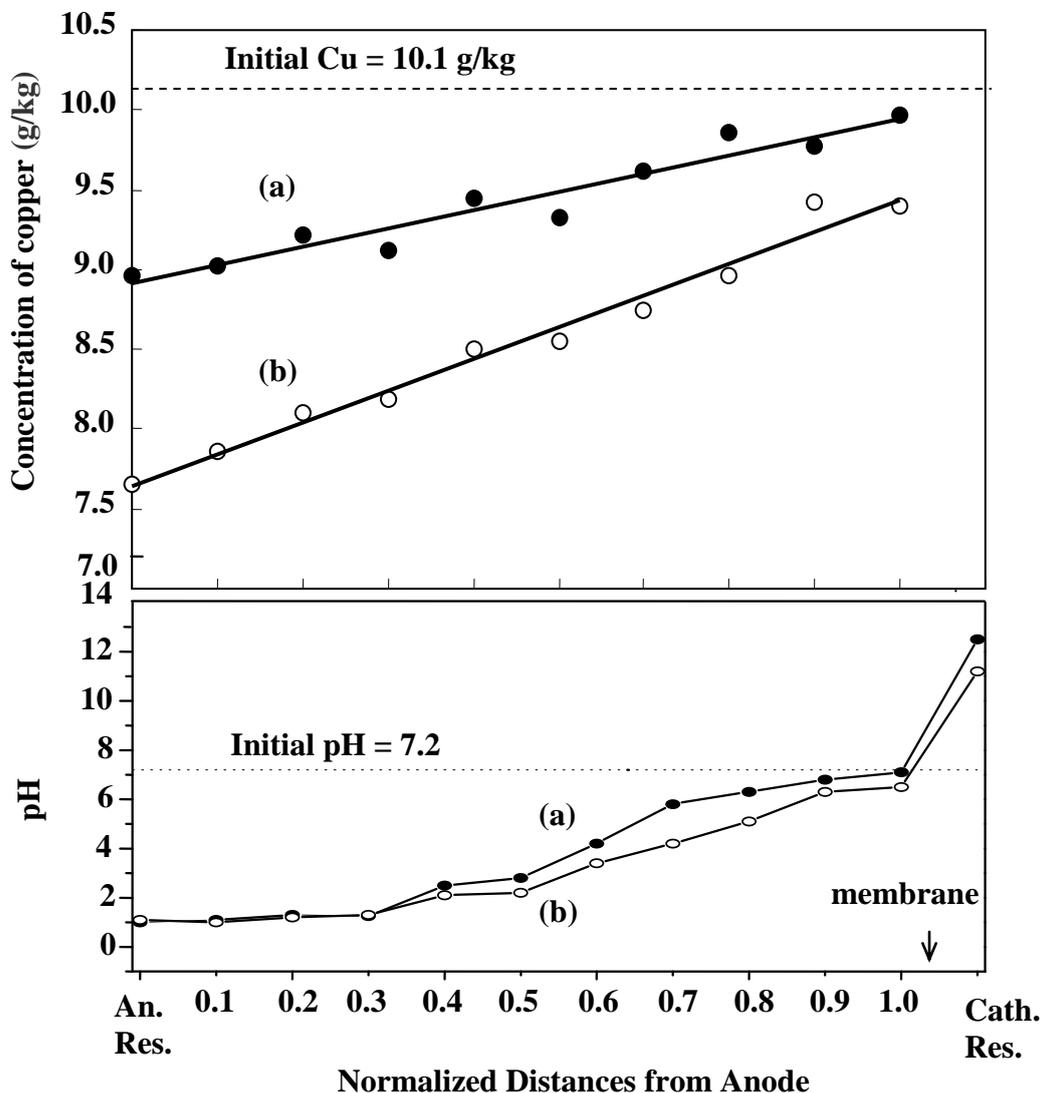
**Figure 1.** Concentrations of copper in the contaminated soil and pH values in the electrolyte between electrodes after 180 min of the electro-treatments (a) without and (b) with EDTA (0.05 M).
