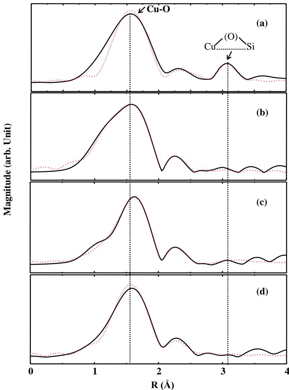
**Figure 5.** In-situ Fourier transformed Cu K edge EXAFS of Cu-contaminated soils (a) without and (b) with EDTA (0.05 M) for the electro-treatments of (c) 90 and (d) 180 min. The dotted curves denote the best fitting of the EXAFS spectra.
