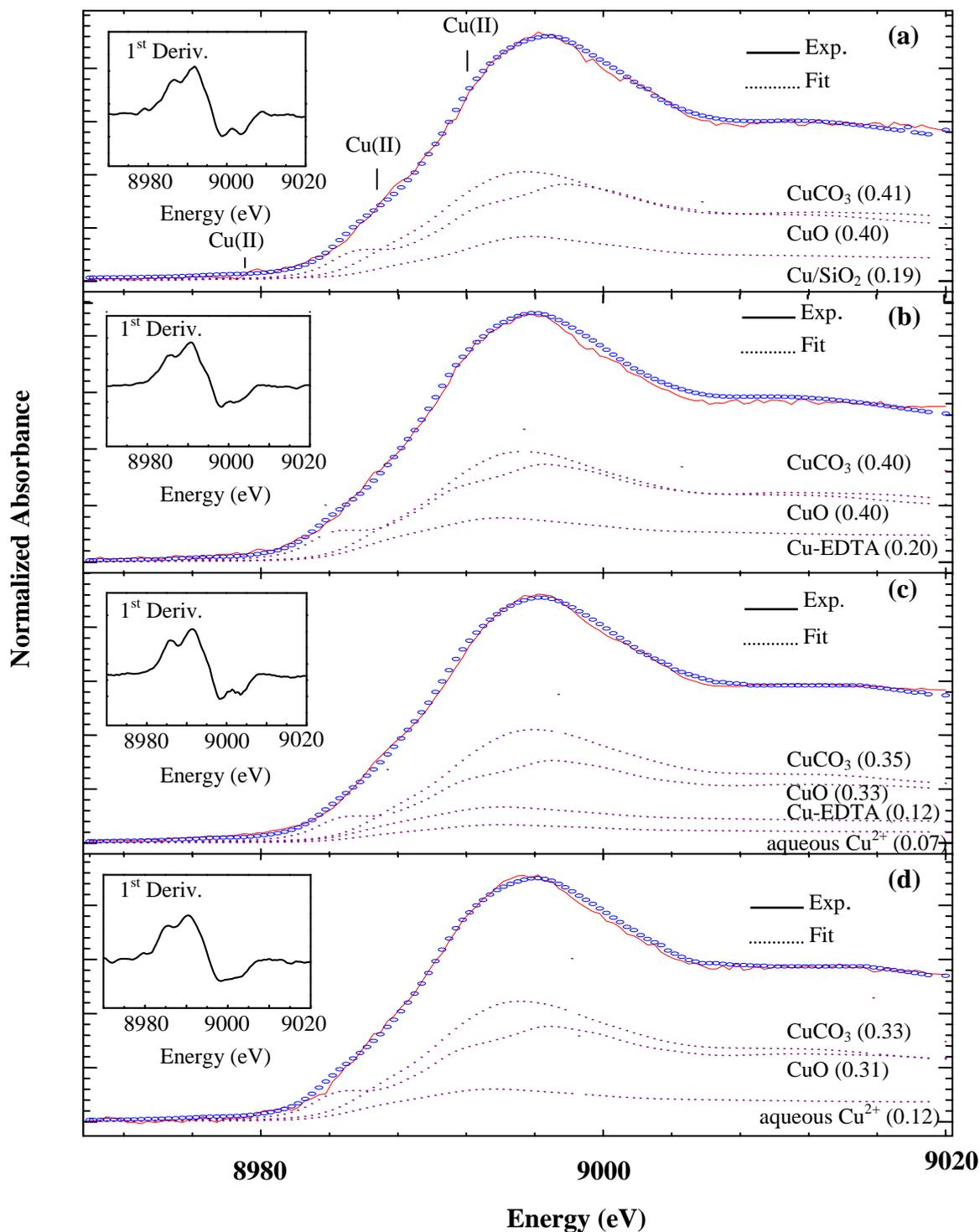
**Figure 3.** In-situ XANES spectra and their first derivative of the Cu-contaminated soil (a) without and (b) with EDTA (0.05 M) for the electro-treatments of (c) 90 and (d) 180 minutes. Solid lines and circles represent experimental data and the least-square fits, respectively. Dotted lines denote fractional contributions of the four main components (Cu(OH)<sub>2</sub>, CuCl<sub>2</sub>, Cu-EDTA and aqueous Cu<sup>2+</sup>) making up the fitted spectra.
