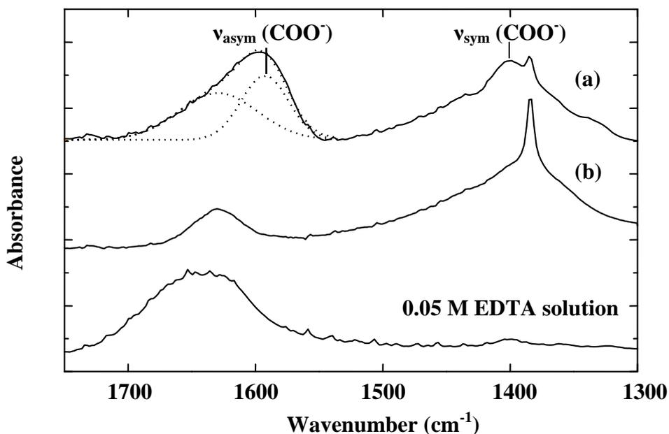
**Figure 2.** FTIR spectra of the Cu-contaminated soil in the presence of EDTA (0.05 M) (a) before and (b) after (180 min) the electro-treatments.
