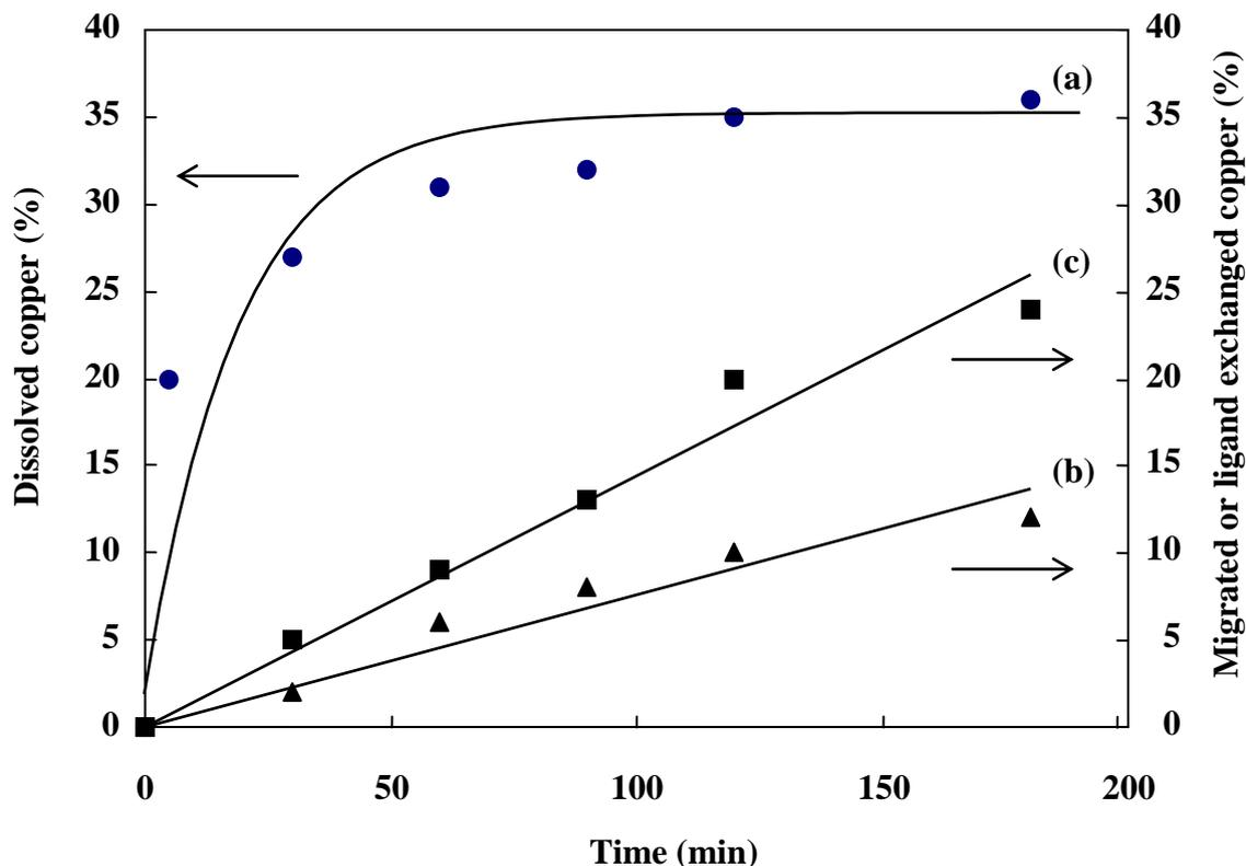
**Figure 4.** Time dependence for (a) dissolution, (b) ligand exchange and (c) electromigration of copper during the electrotreatments.
