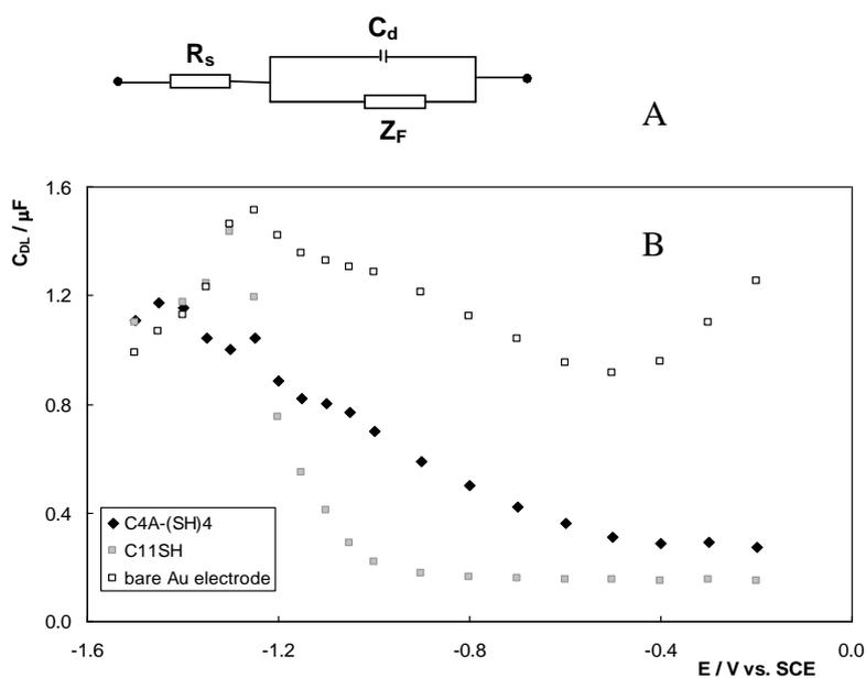
**Figure 5.** Electric equivalent circuits used to fit the impedance spectra (A) and the changes in the double-layer capacitance during the desorption processes of  $C_4A-(SH)_4$  and  $C_{11}SH$ , compared to the bare gold electrode (B). Modified electrode: Self-assembly modification (thiols concentration:  $c_{ADS} 5 \cdot 10^{-5}$  M in DMF solution; adsorption time:  $t_{ADS}$  10 min for both compounds).
