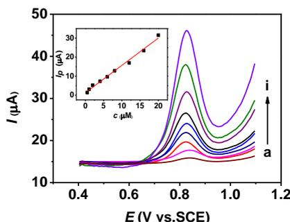
**Figure 6.** DPV of different PHE concentrations. PHE concentrations (from a to i): 0.5, 1.0, 2.0, 4.0, 6.0, 8.0, 12.0, 16.0,  $20.0 \times 10^{-6} \text{ mol L}^{-1}$ . The insert is linear dependence of the peak current on PHE concentration.
