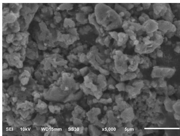
**Figure 2.** SEM image of GR/TiO<sub>2</sub>.
