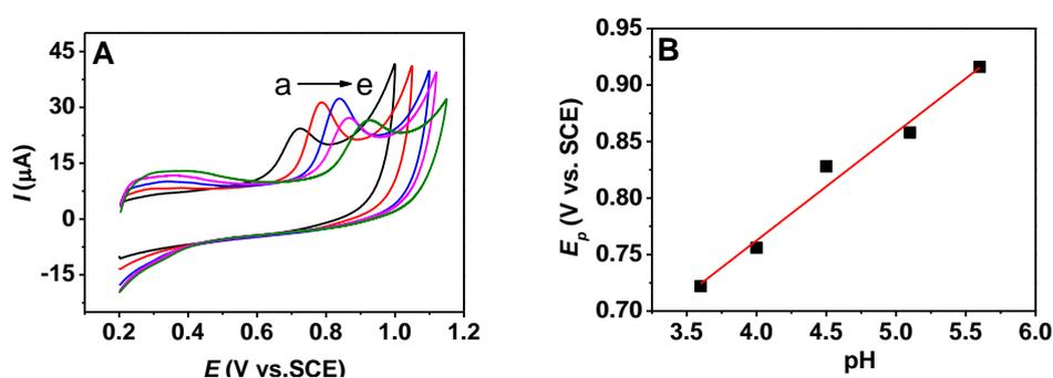
**Figure 5.** (A) Cyclic voltammograms of PHE at different pH, curve a-e: 3.6, 4.0, 4.6, 5.1, 5.6. (B) A linear relationship between the peak potential and the pH.
