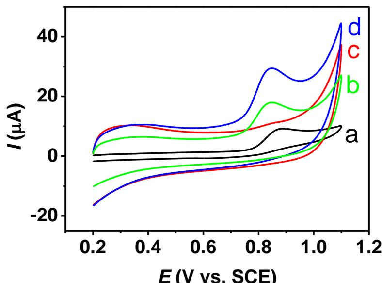
**Figure 3.** Cyclic voltammograms of  $1.0 \times 10^{-5} \text{ mol L}^{-1}$  PHE at GCE (a), GR/GCE (b), GR/TiO<sub>2</sub>/GCE (c), GR/TiO<sub>2</sub>/GCE (d) in  $0.1 \text{ mol L}^{-1}$  HAc-NaAc (pH 4.6). Scan rate:  $50 \text{ mV s}^{-1}$ .
