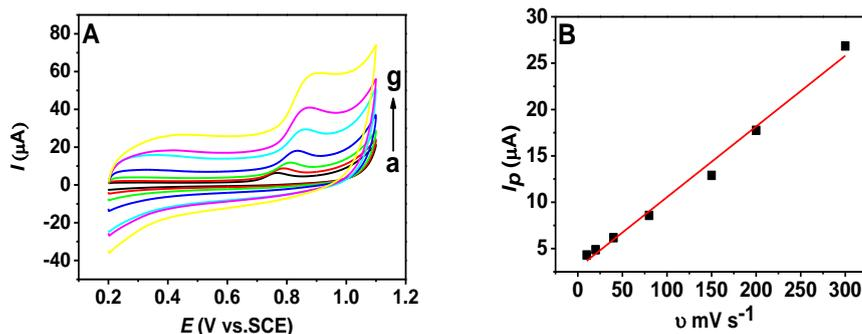
**Figure 4.** (A) Cyclic voltammograms of PHE at different scan rates. Scan rates (curve a-g): 10, 20, 40, 80, 150, 200, 300  $\text{mV s}^{-1}$ . (B) A linear relationship between the peak current and the square root of scan rate.
