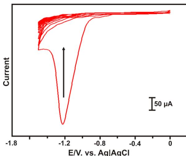
**Figure 2.** 30 successive cyclic voltammograms were performed in GO modified GCE at 0 to -1.5 V in pH 5 solution at the scan rate 50 mVs<sup>-1</sup>.
