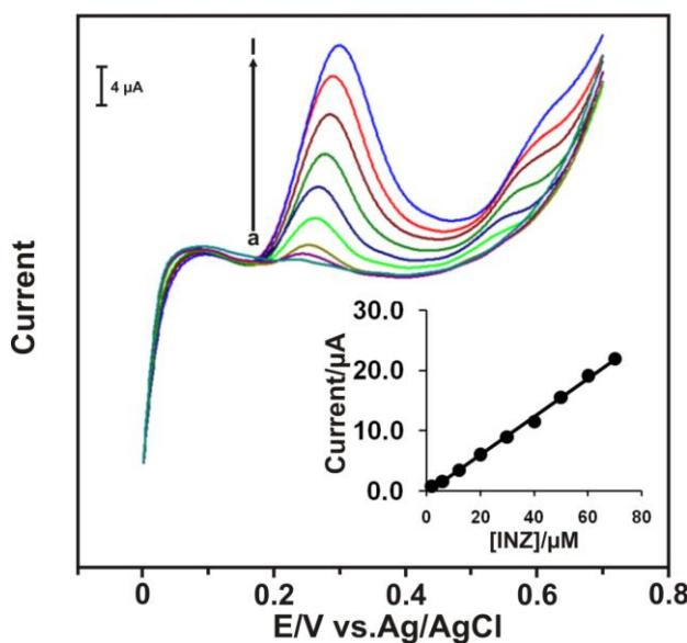
**Figure 8.** LSV of ERGO modified GCE in different concentration of INZ (a-i) in PBS at the scan rate of 100  $\text{mV s}^{-1}$ . Inset plot shows the linear dependence of  $I_{pa}$  vs. [INZ]
