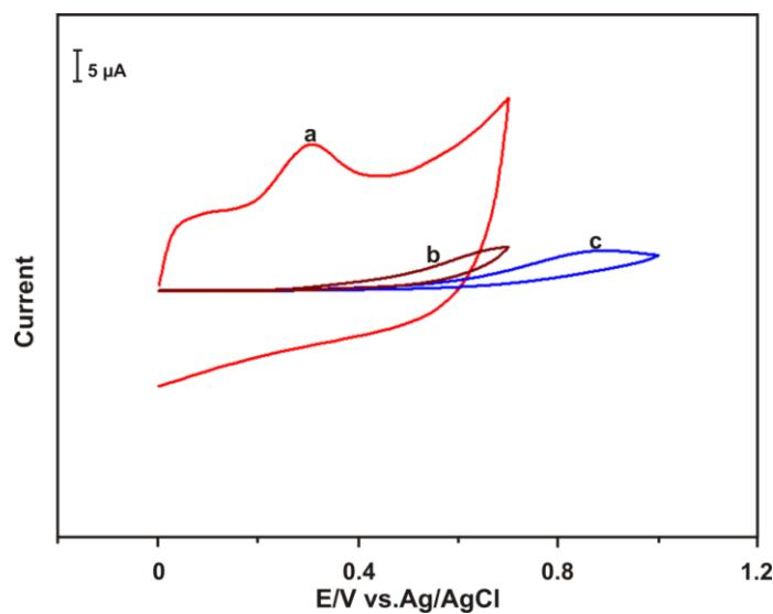
**Figure 5.** Cyclic voltammograms of ERGO/GCE (a), GO/GCE (b), and bare GCE (c) modified electrodes in the presence of  $60 \mu\text{M}$  INZ in deoxygenated PBS at  $100 \text{ mV s}^{-1}$  scan rate.
