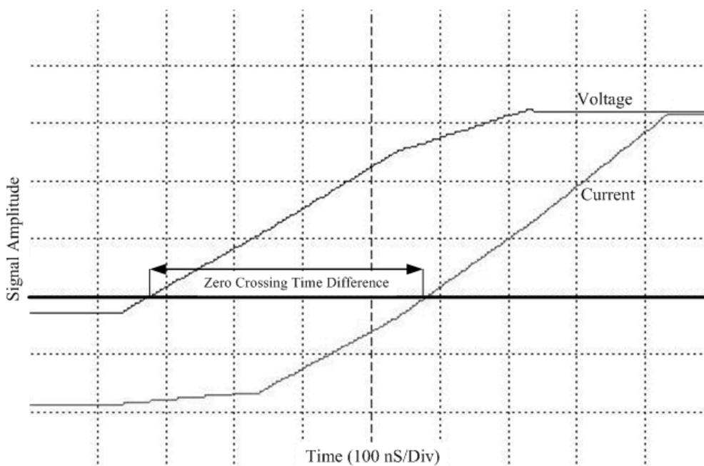
**Figure 5.** Reading the time difference between waveforms zero crossing in AC coupling
