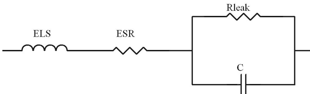
**Figure 7.** Simplified second order electrical equivalent circuit
