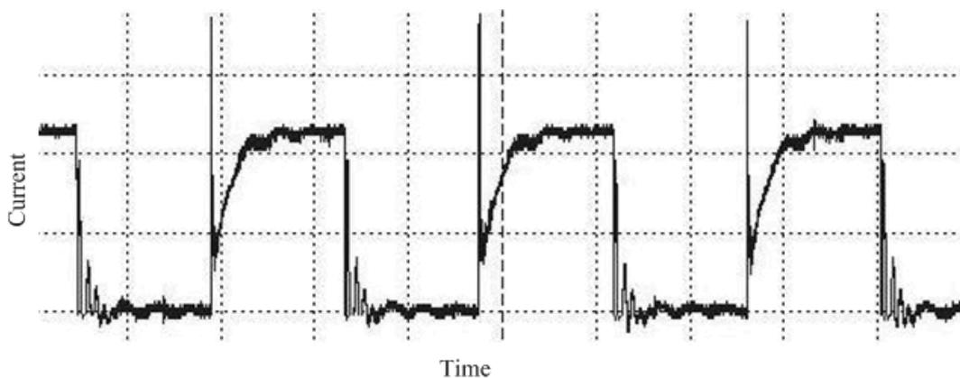
**Figure 1.** Sample PWM electrolyzer current waveform
