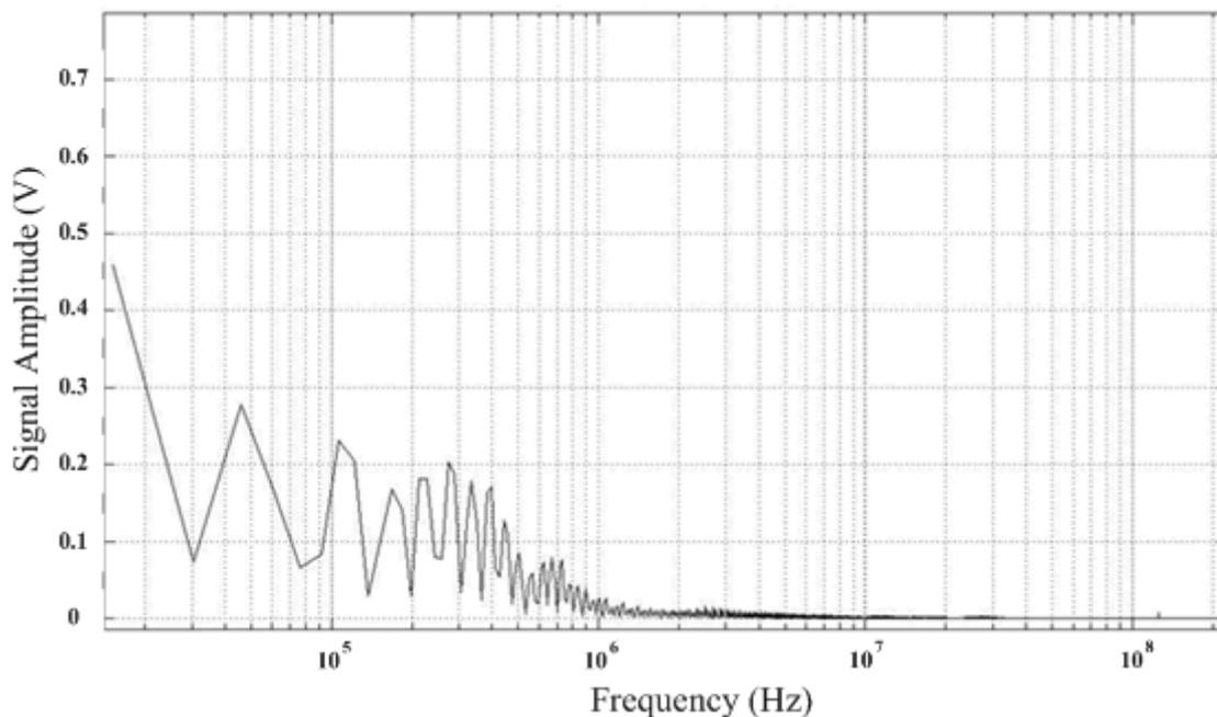
**Figure 2.** Fast Fourier Transform of the current waveform of figure 1
