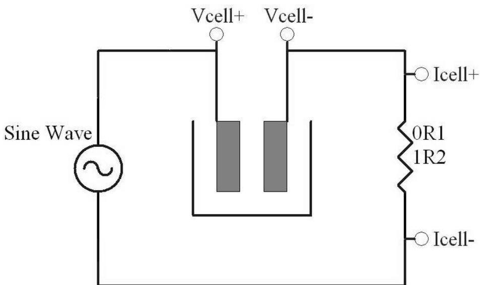
Figure 3. Electrical schematic of the experimental setup
