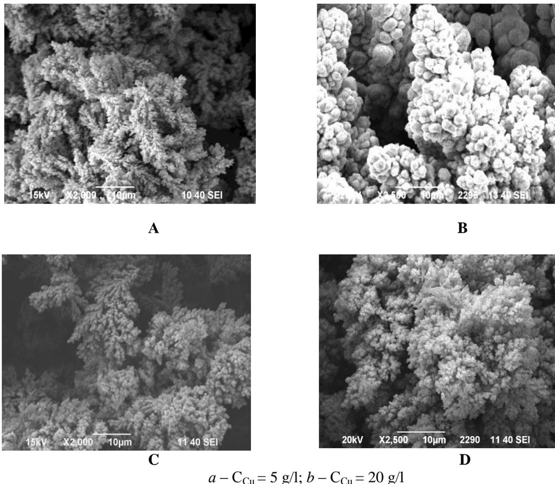
**Figure 4.** Micrographs of copper powders obtained by adding a solution of glycerin (50 ml), and from electrolyte ( $C_{Cu} = 5 \text{ g/l}$ ) without the addition of an organic compound (c) and when added 20 ml ethylene glycol to a solution (d).
