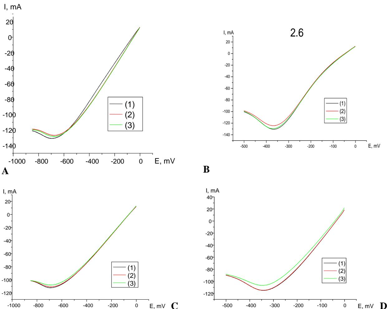
*a* –  $\text{CH}_2\text{SO}_4 = 10 \text{ g/l}$ ; glycerol amount = 10 ml; *b* –  $\text{CH}_2\text{SO}_4 = 50 \text{ g/l}$ ; glycerol amount = 10 ml; *c* –  $\text{CH}_2\text{SO}_4 = 10 \text{ g/l}$ ; glycerol amount = 50 ml; *d* –  $\text{CH}_2\text{SO}_4 = 50 \text{ g/l}$ ; glycerol amount = 50 ml
