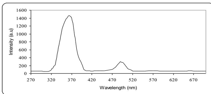
**Figure 3.** PL spectra of the ZnS nanoparticles prepared at pH =3
