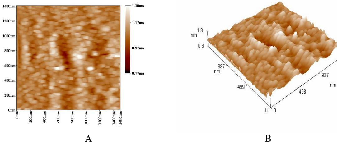
**Figure 5.** AFM images of ZnS powder placing on glass. (a) Two-dimensional and (b) three – dimensional.
