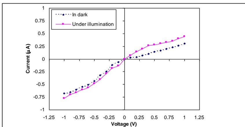
**Figure 4.** Current vs. voltage plots in dark and under illumination for a ZnS nanoparticle
