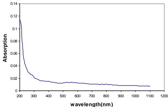
/ **Figure 2.** UV-Vis absorption spectra of ZnS nano-particles.
