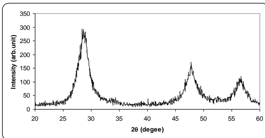
Figure 1. XRD of ZnS nanoparticle.
