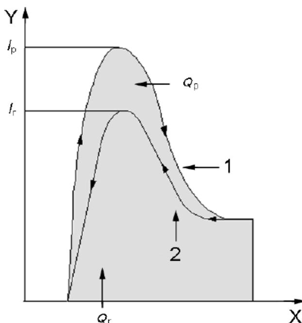
**Figure 1.** The sketch of polarization curve in double-loop EPR test method X-electric potential, Y-log current density, 1-anode scanning, 2-reactivation scanning.
