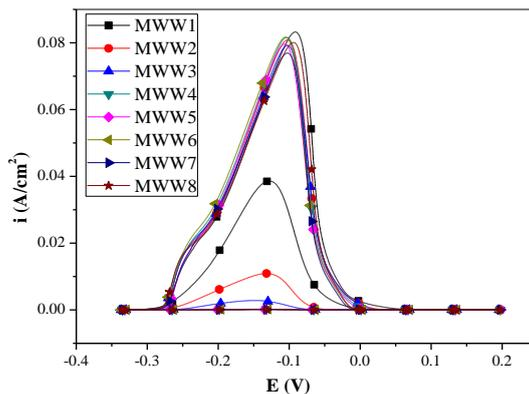
Figure 2. The DL-EPR test curves of alloy 690 with different thermal treatments.
