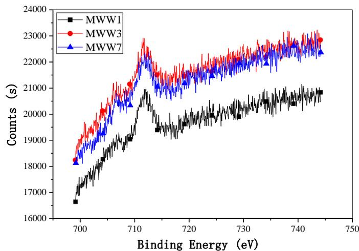
Figure 5. The photoelectron binding energy spectrogram of Fe in the specimen surface.
