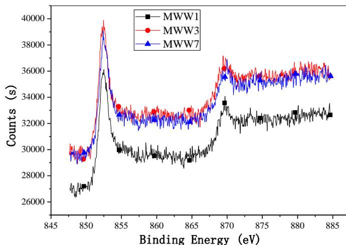
Figure 6. The photoelectron binding energy spectrogram of Ni in the specimen surface.
