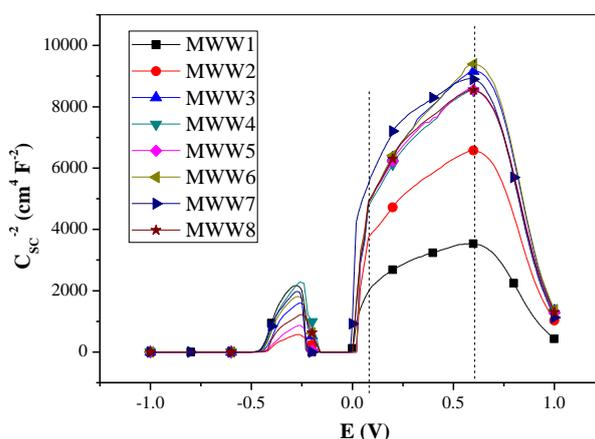
**Figure 7.** The Mott–Schottky plots of alloy 690 with different thermal treatments.
