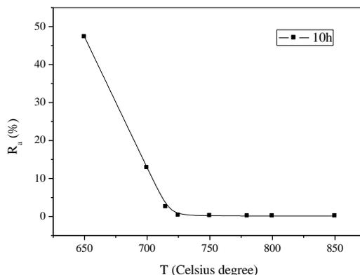
**Figure 3.** The relationship between R<sub>a</sub> value and the TT temperature for alloy 690.
