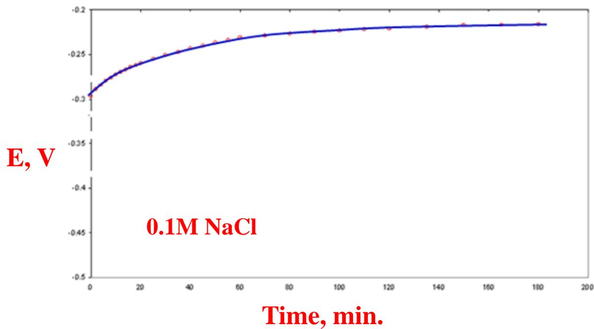
**Figure 1.** Variation of potential with immersion time for maraging steel immersed in 0.1M NaCl solution.
