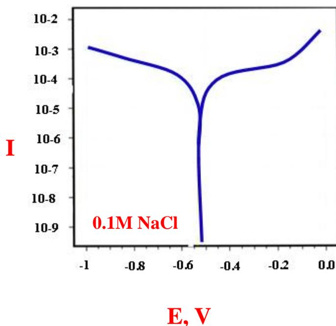
**Figure 5.** Polarization curve for the corrosion of maraging steel in 0.1M NaCl solution.
