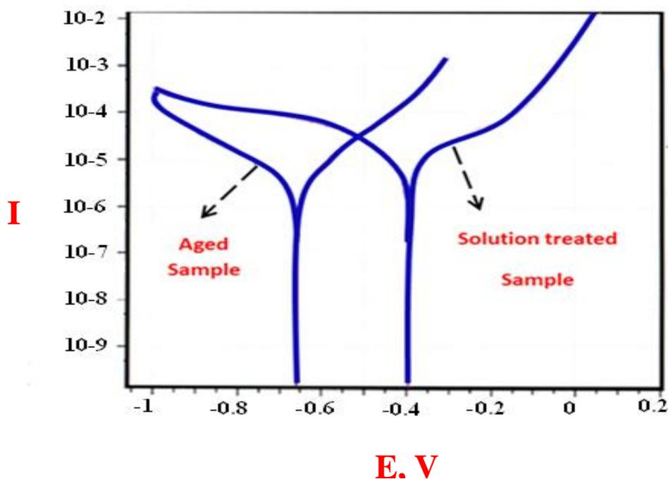
**Figure 8.** Polarization curves for the corrosion of aged and solution treated maraging steel in 0.6M NaCl solution.
