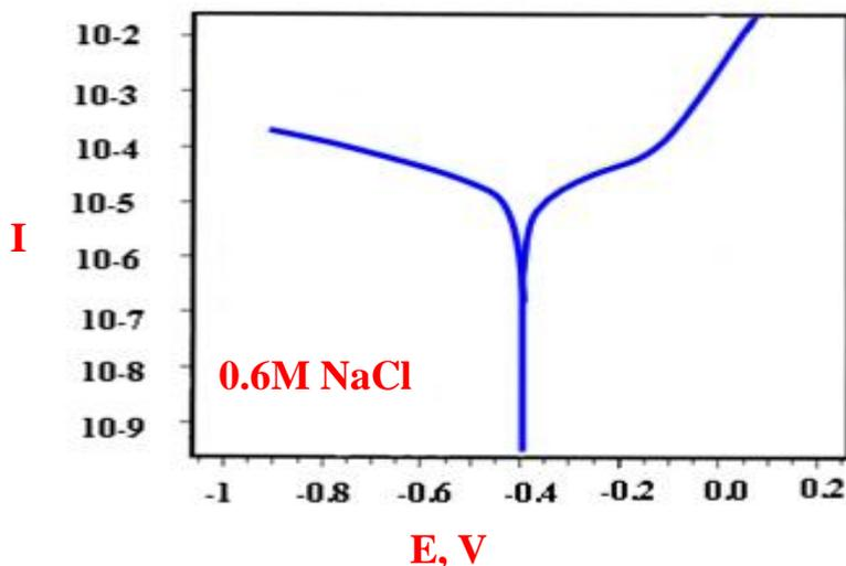
Figure 6. Polarization curve for the corrosion of maraging steel in 0.6M NaCl solution.
