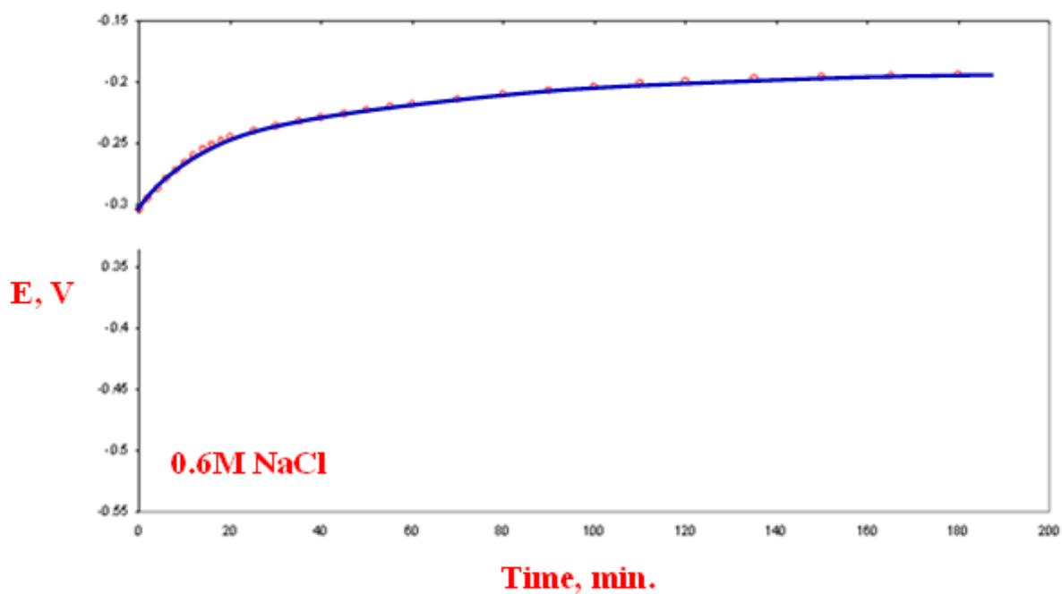
**Figure 2.** Variation of potential with immersion time for maraging steel immersed in 0.6M NaCl solution.
