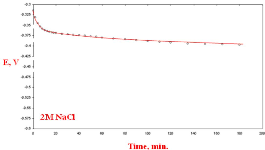
**Figure 3.** Variation of potential with immersion time for maraging steel immersed in 2M NaCl solution.
