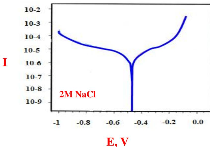
Figure 7. Polarization curve for the corrosion of maraging steel in 2M NaCl solution.
