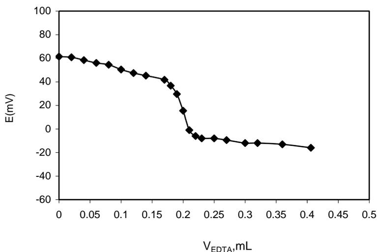
**Figure 5.** Potential titration curves of 20.0 mL  $1.0 \times 10^{-4}$  mol L<sup>-1</sup> Tm<sup>3+</sup> solution with  $1.0 \times 10^{-2}$  mol L<sup>-1</sup> of EDTA.
