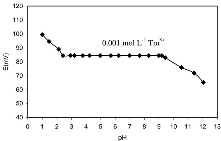
**Figure 3.** pH effect of the test solution ( $1.0 \times 10^{-3}$  mol L<sup>-1</sup> of Tm<sup>3+</sup>) of the Tm<sup>3+</sup> sensor based on PTP.
