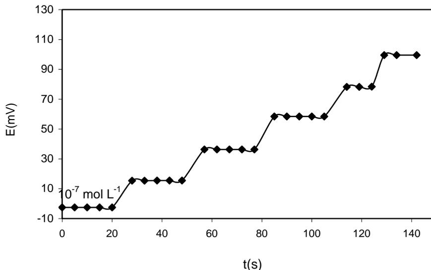
**Figure 4.** Dynamic response time of  $Tm^{3+}$  sensor based on PTP.
