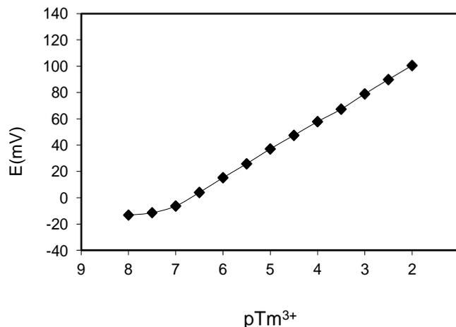
**Figure 2.** Calibration curves of the PTP-based Tm<sup>3+</sup> sensor.
