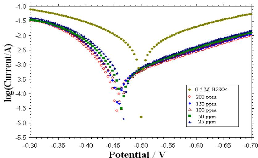
**Figure 10.** Tafel plots showing effect of increasing concentration of *Ipomoea triloba* leaves extracts on corrosion of MS in H<sub>2</sub>SO<sub>4</sub> solutions
