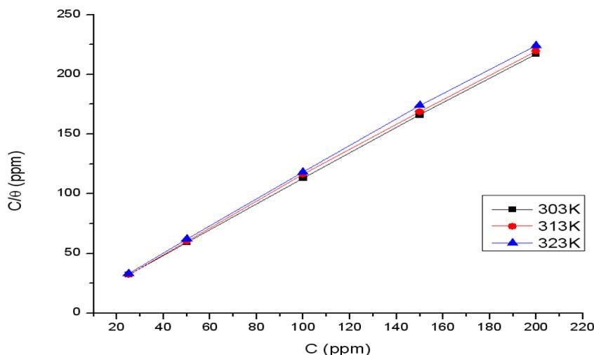
**Figure 1.** Langmuir adsorption plots for MS in 0.5 M H<sub>2</sub>SO<sub>4</sub> at different temperatures in presence of various concentration of Wrightia Tinctoria leaves extract
