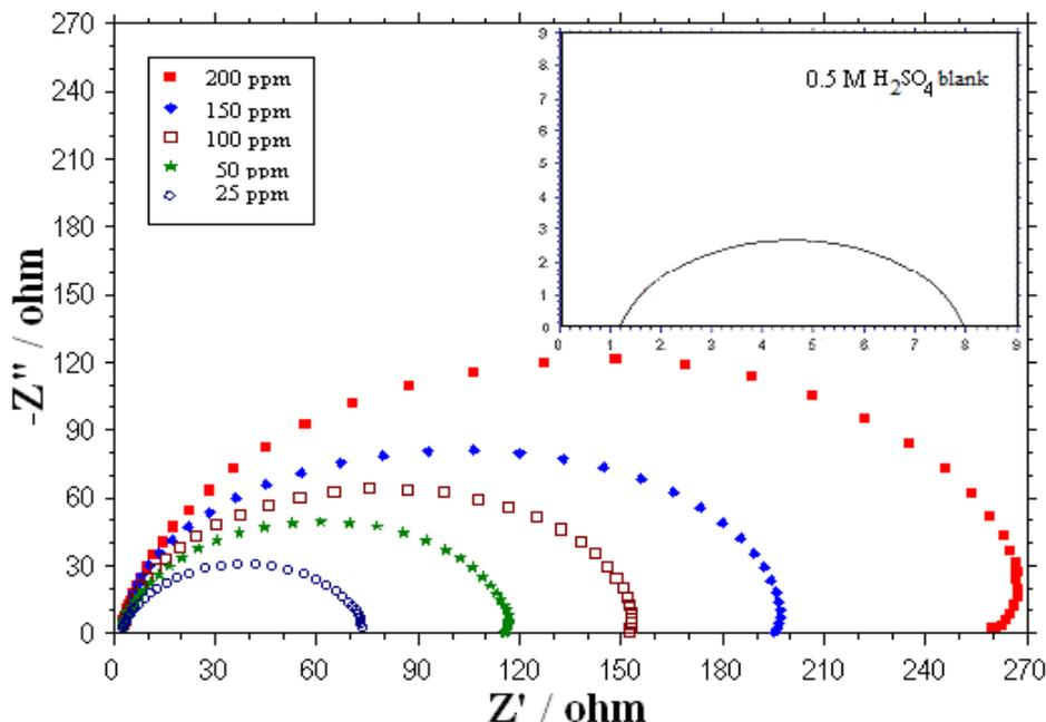
**Figure 3.** Nyquist plots showing effect of increasing concentration of Wrightia Tinctoria leaves extract on corrosion of MS in H<sub>2</sub>SO<sub>4</sub> solutions
