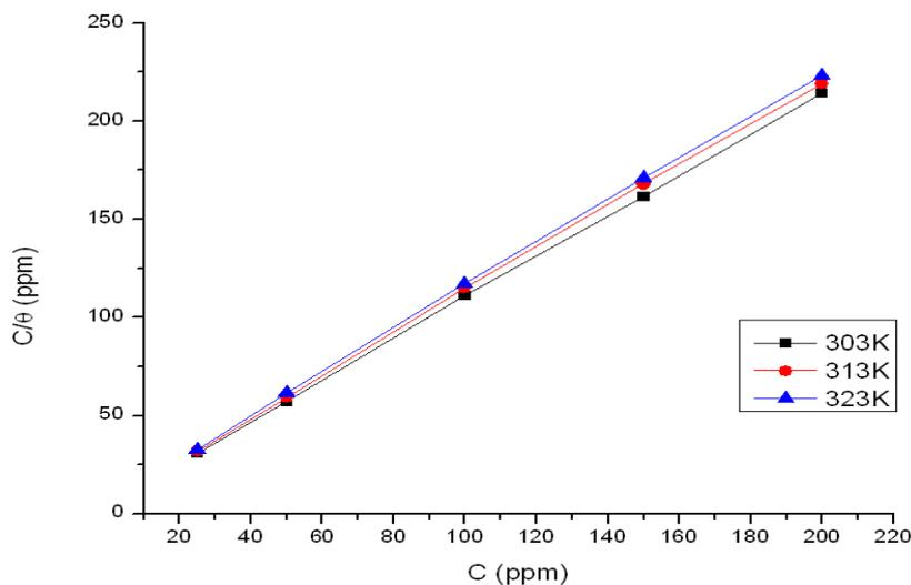
**Figure 5.** Langmuir adsorption plots for MS in 0.5 M  $H_2SO_4$  at different temperatures in the presence various concentration of Clerodendrum phlomidis leaves extract
