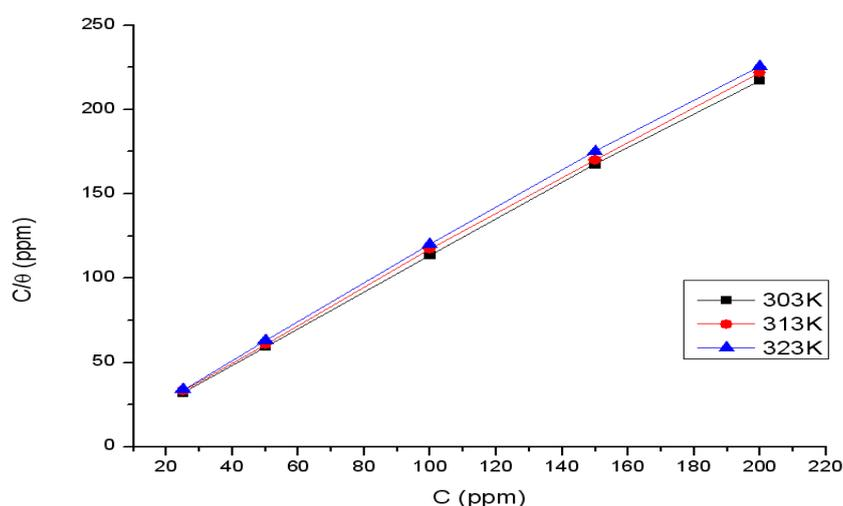
**Figure 9.** Langmuir adsorption plots for MS in 0.5 M  $H_2SO_4$  at different temperatures in presence various concentration of Ipomoea triloba leaves extract
