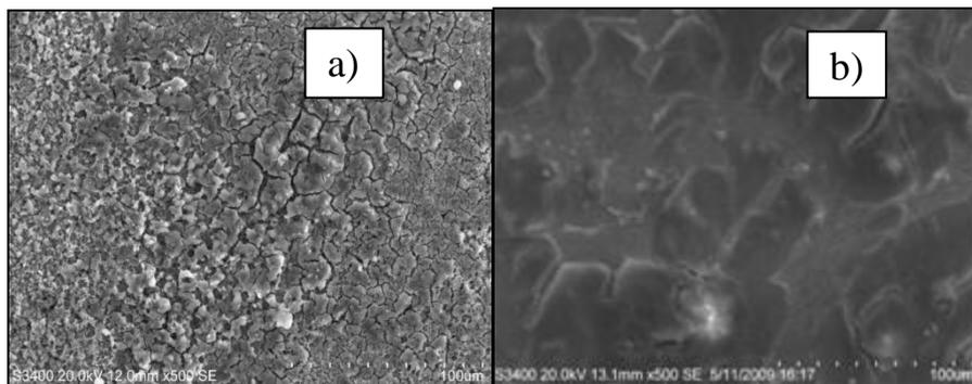
**Figure 4.** SEM image of MS surface, a) in 0.5 M H<sub>2</sub>SO<sub>4</sub> solution, and that of b) with 200 ppm of Wrightia Tinctoria leaves extract
