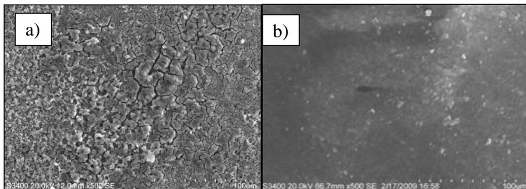
**Figure 12.** SEM image of MS surface, a) in 0.5 M H<sub>2</sub>SO<sub>4</sub> solution, and that of b) with 200 ppm of *Ipomoea triloba* leaves extract
