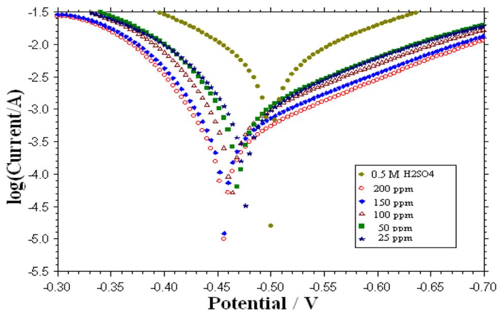
**Figure 2.** Tafel plots showing effect of increasing concentrations of *Wrightia Tinctoria* leaves extracts on corrosion of MS in  $H_2SO_4$  solutions
