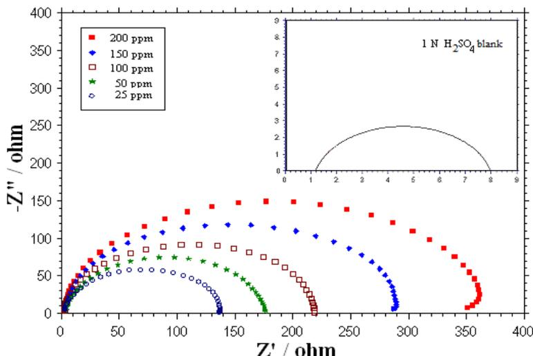
**Figure 11.** Nyquist plots showing effect of increase in concentration of Ipomoea triloba leaves extract on corrosion of MS in H<sub>2</sub>SO<sub>4</sub> solutions
