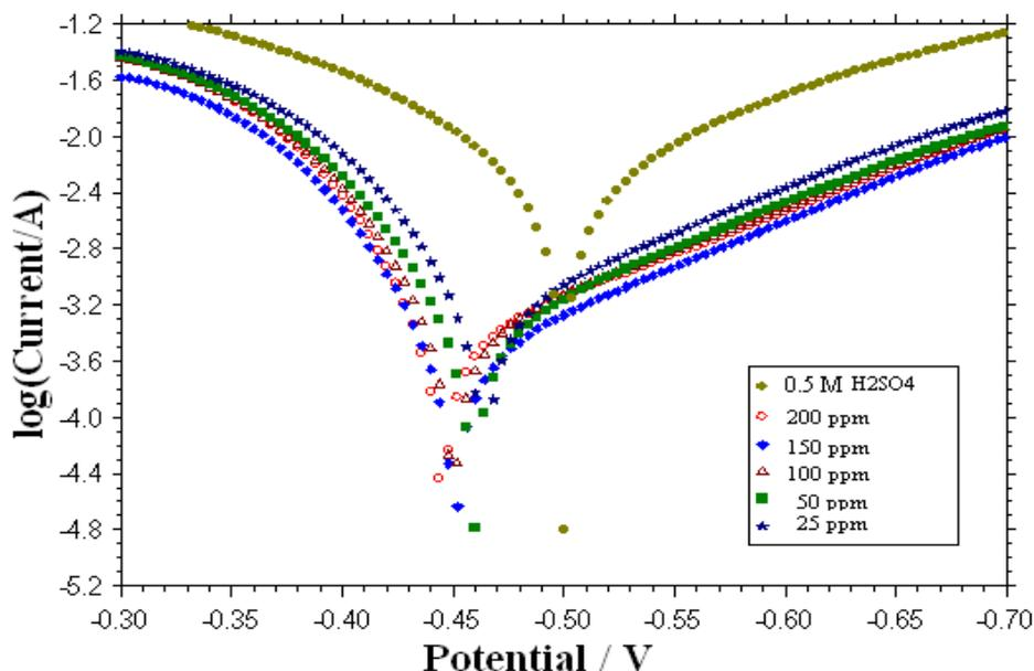
**Figure 6.** Tafel plots showing effect of Clerodendrum phlomidis leaves extracts on corrosion of MS in H<sub>2</sub>SO<sub>4</sub> medium
