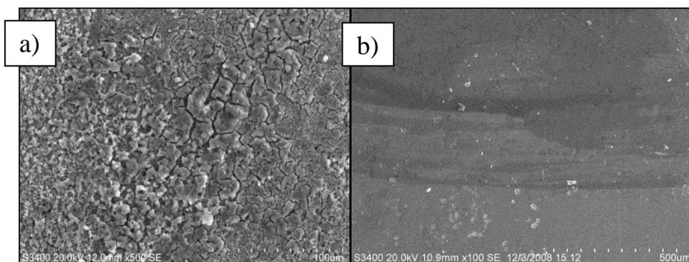
**Figure 8.** SEM image of MS surface, a) in 0.5 M H<sub>2</sub>SO<sub>4</sub> solution, and that of b) with 200 ppm of Clerodendrum phlomidis leaves extract
