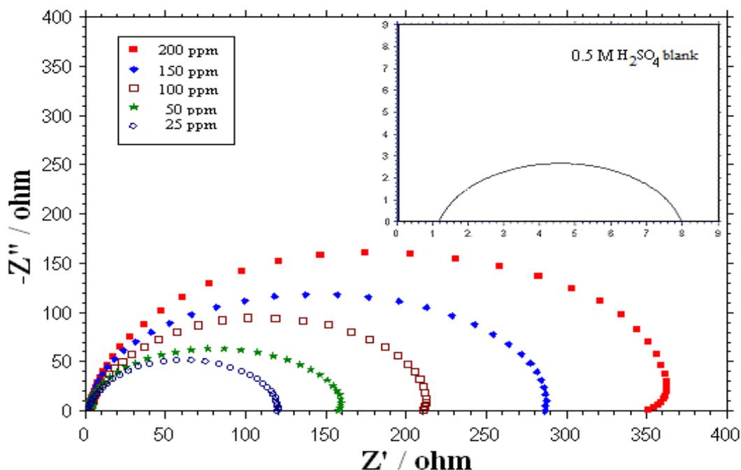
**Figure 7.** Nyquist plots showing effect of Clerodendrum phlomidis leaves extracts on corrosion of MS in 0.5 M H<sub>2</sub>SO<sub>4</sub> solutions
