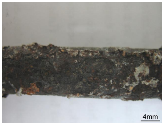
Figure 6. Corrosion morphology of the rebar after 14 cycles corrosion.
