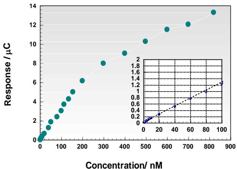
**Figure 9.** Response of the Chi- $ZrO_2$ /GNS-IL/GC electrode to Alfuzosin upon the following concentrations: A) 2 to 800 nM n PB solution, pH 5.0 B) The calibration curve for Alfuzosin determination
