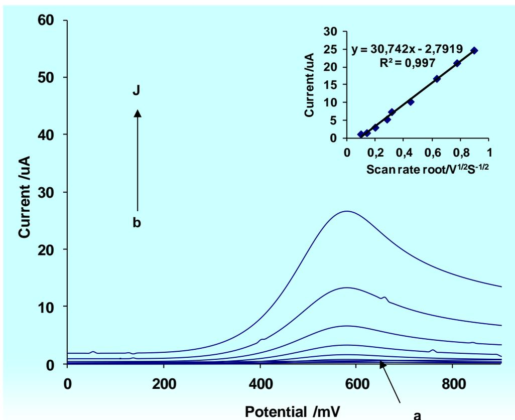
**Figure 4.** Typical Linear sweep voltammograms of 2  $\mu$ M Alfuzosin in 0.05 M PBS pH 5.0 at the bare GCE, Chi-ZrO<sub>2</sub>/GNS-IL/GCE; scan rates 10 to 800 mV/s
