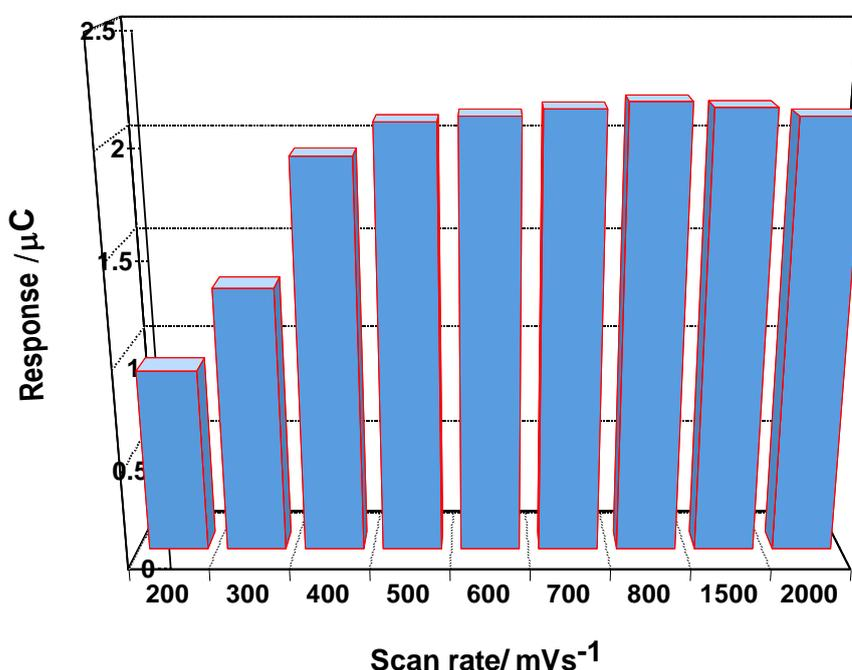
**Figure 6.** The effect of the scan rate on the response of the Chi-ZrO<sub>2</sub>/GNS-IL/GCE in  $2.0 \times 10^{-7}$  M Alfuzosin in 0.05 M PB solution in the potential range of 0 to 900 mV.
