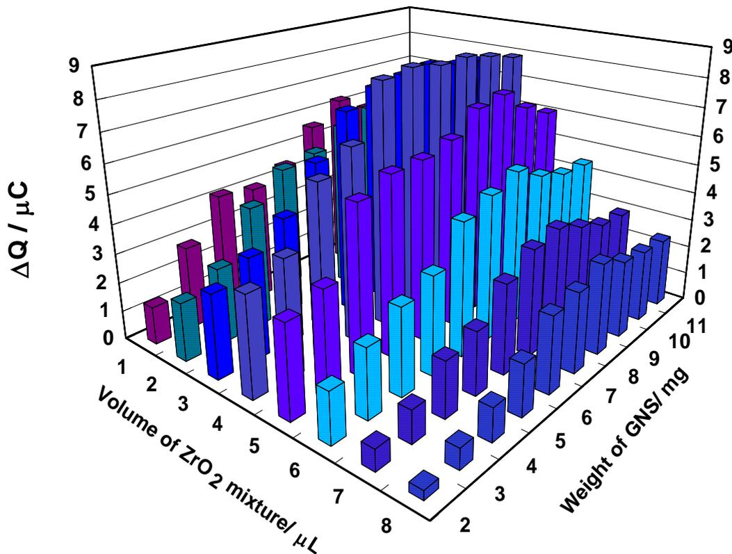
**Figure 8.** The effect of amount of ZrO<sub>2</sub> and GNS on the sensor response to  $5.0 \times 10^{-7}$  M of Alfuzosin in 0.05 M PBS at pH=5.0
