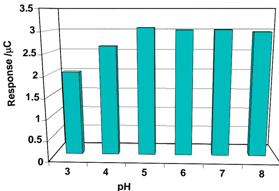
**Figure 7.** The effect of pH concentration on the sensor response to  $2.5 \times 10^{-7}$  M Alfuzosin in 0.05 M PB solution in the potential range of 0 to 900 mV at potential scan rate 800 mV/s
