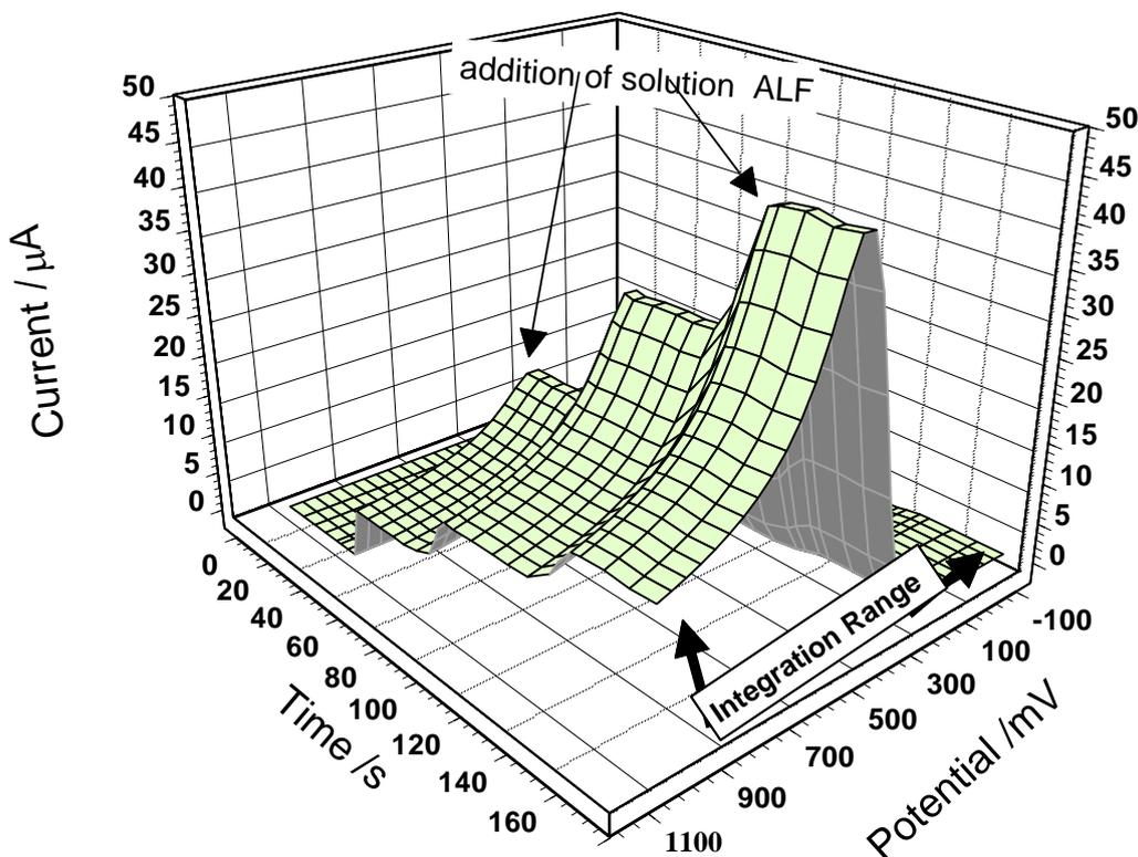
**Figure 5.** a) CFFTL SV voltammograms of the Chi-ZrO<sub>2</sub>/GNS-IL/GCE sensor in absent and present of 1.0, 2.0., and 3.0 × 10<sup>-6</sup> M Alfuzosin in PB solution at pH 5.0 in the potential range of 0 to 900 mV at potential scan rate 800 mV/s.
