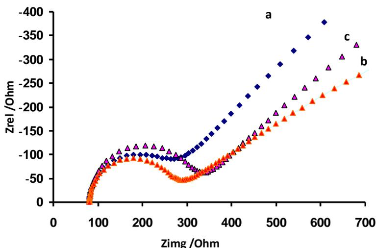
**Figure 3.** A) SEM images of Chi- $\text{ZrO}_2$ /GNS-IL. B) EIS plots of modified electrode in 3 mM  $\text{K}_3\text{Fe}(\text{CN})_6$  with 0.05 M KCl: (a) bare GCE (b) GNS-IL/GCE and (c) Chi- $\text{ZrO}_2$ /GNS-IL/GCE.
