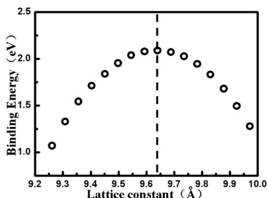
**Figure 2.** Binding energies of a single Li atom as the function of lattice constant, the dashed line denotes the equilibrium lattice constant.
