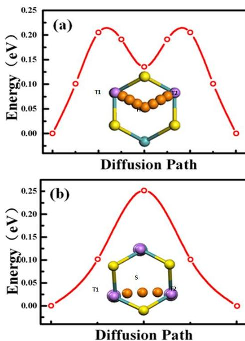
**Figure 5.** Lowest energy diffusion paths of a single lithium atom and calculated energy profiles along the paths for (a) one Li atom adsorbed on the MoS<sub>2</sub> monolayer, (b) seventeen Li atoms adsorbed on the MoS<sub>2</sub> monolayer.
