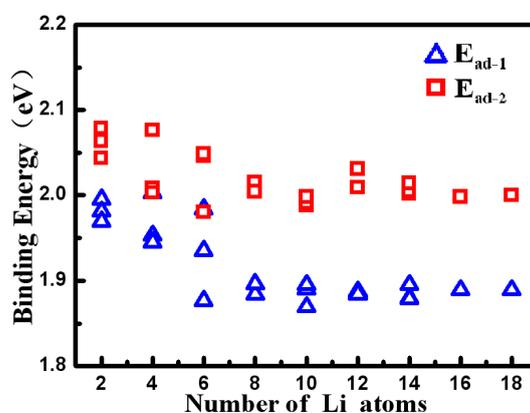
**Figure 4.** Binding energies as a function of the number of lithium atoms.  $E_{ad-1}$  (blue triangle) and  $E_{ad-2}$  (red square) denote the binding energies of lithium atom without and with lattice relaxation, respectively.
