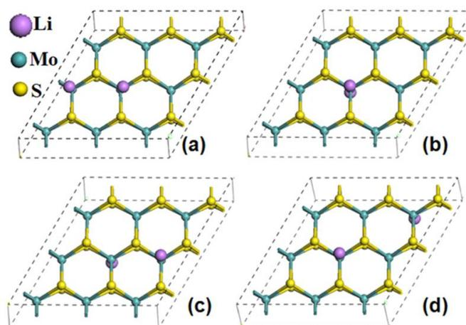
**Figure 3.** Optimized structures of two lithium atoms adsorbed on the MoS<sub>2</sub> monolayer. (a) On one side, (b), (c) and (d) on two sides. (b) On the opposite sides of a Mo atom, (c) on the nearest neighboring Mo atoms, and (d) on the next nearest neighboring Mo atoms.
