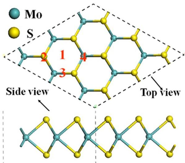
**Figure 1.** Optimized structures of MoS<sub>2</sub> monolayer with four adsorption sites (1) hollow site, (2) top site of the S atom, (3) Mo-S bridge site, and (4) top site of the Mo atom.
