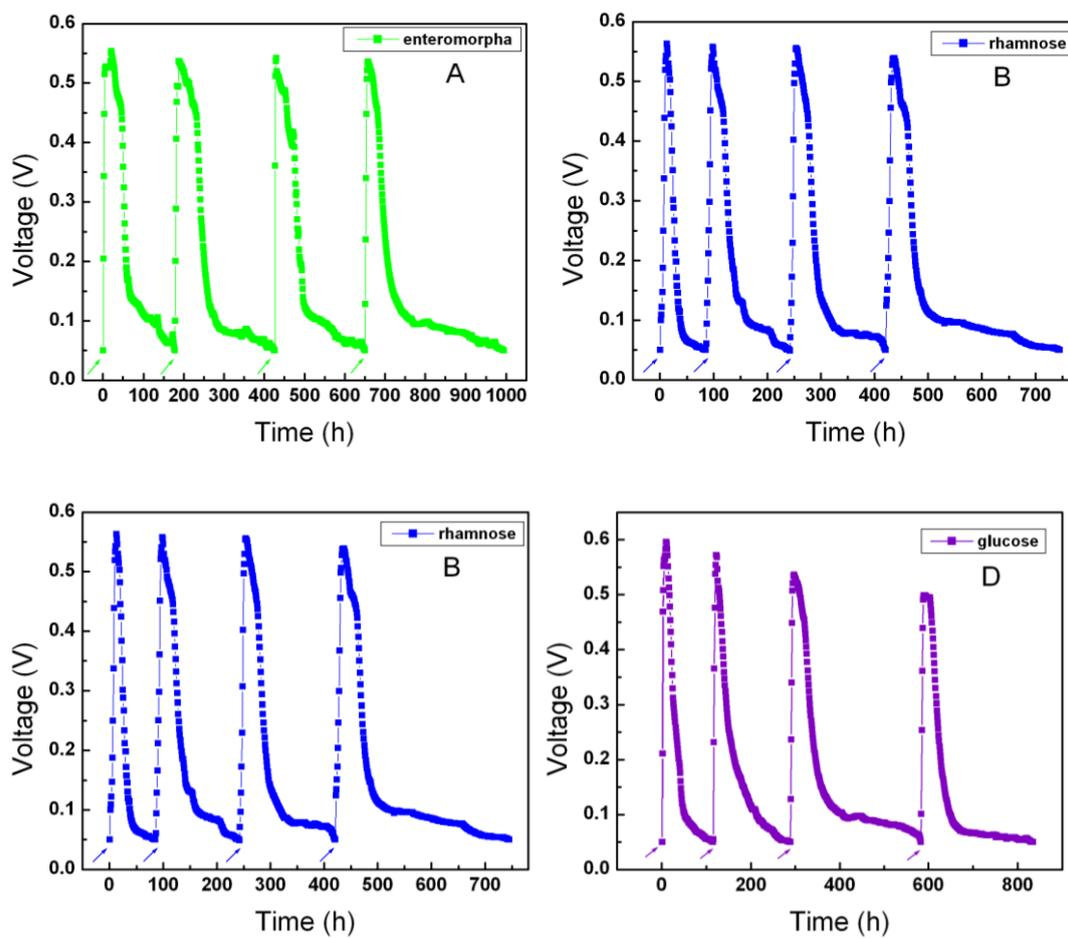
**Figure 1.** Voltage output over time of the MFC with external resistance of 1000 Ω. (A) the substrate was *E. proliferata* hydrolysate, (B) rhamnose, (C) xylose, (D) glucose. The concentration for each substrate was 1g-COD/L. The arrows indicate when MFC were fed with fresh medium.
