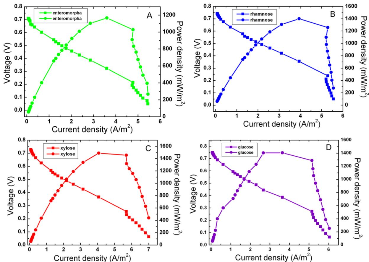
**Figure 2.** Power density curves and polarization curves of the MFC. (A) the substrate was *E. proliferans* hydrolysate. (B) the substrate was rhamnose. (C) the substrate was xylose. (D) the substrate was glucose. The concentration for each substrate was 1 g-COD/L.
