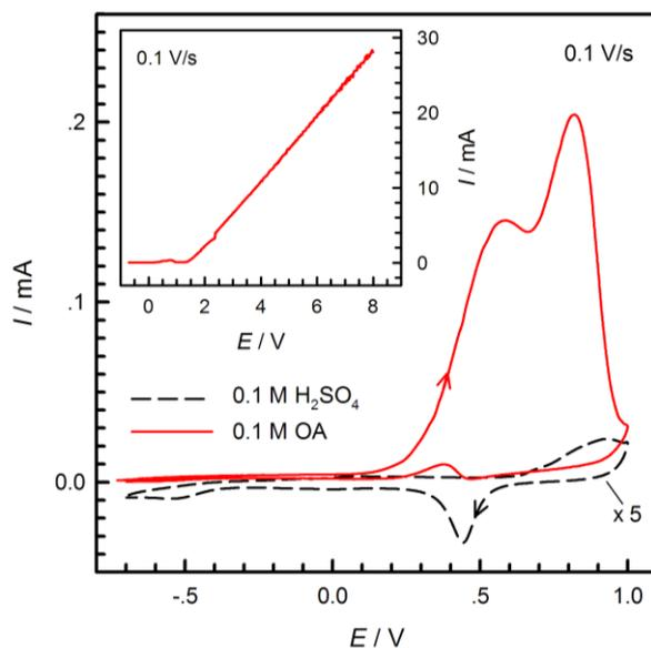
**Figure 1.** CVs with an upper potential limit of 1 V on the smooth gold electrode in 0.1 M  $\text{H}_2\text{SO}_4$  (the dashed line) and 0.1 M OA (the solid line) respectively. Note that the data of dashed line have been magnified by 5 times. The inset shows the linear sweep voltammetry with an upper potential limit of 8 V.
