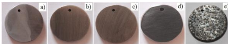
Figure 7. Macroscopical surface morphology of carbon steel samples after 6 days immersion in distilled water medium with the presence of (a) 5 ppm, (b) 10 ppm, (c) 15 ppm, (d) 20 ppm and (e) absence nanosilicate.
