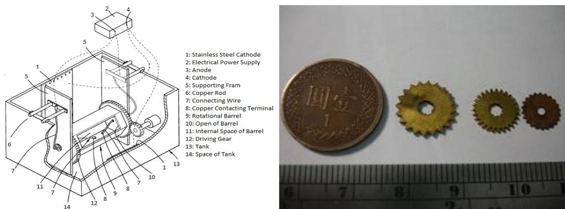
**Figure 1.** (a) Schematic of the electrochemical system of rotational barrel; (b) the pressed brass gears for experiment.
