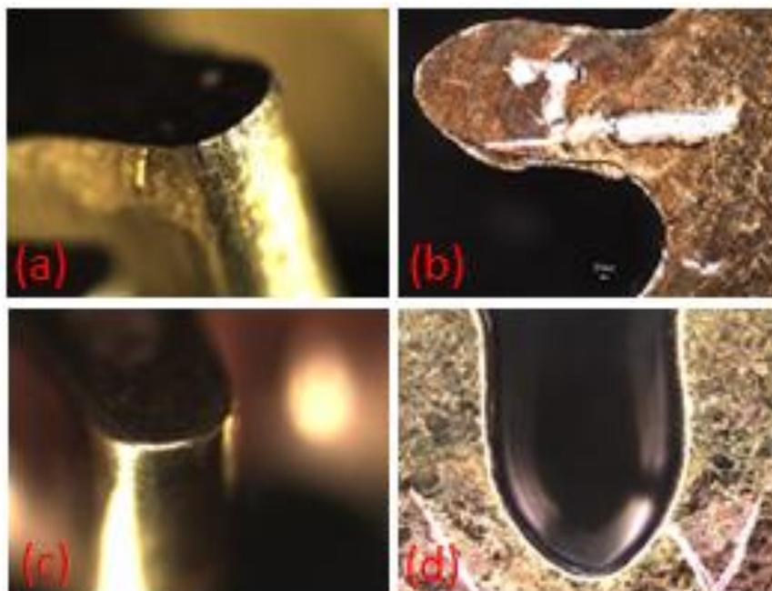
**Figure 5.** (a) and (b) gear tooth before deburring; (c) and (d) gear tooth after deburring. (Magnification : 10x10)
