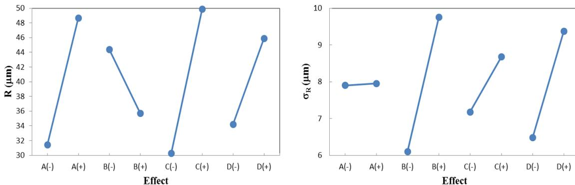
**Figure 3.** (a) Effects to average R; (b) effects to  $\sigma_R$  . ((A) applied voltage; (B) rotational speed of barrel; (C) temperature of electrolyte; and (D) process time)
