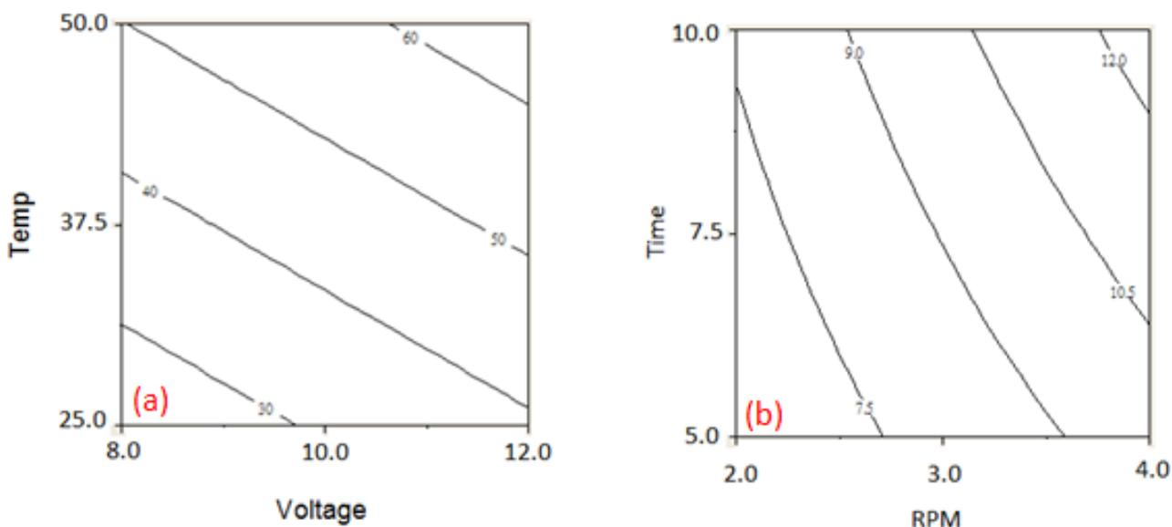
**Figure 4.** (a) Contour plot for constant average R w.r.t. applied voltage vs. temperature of electrolyte. (b) contour plot for constant  $\sigma_R$  w.r.t. rotational speed of the barrel vs. process time.
