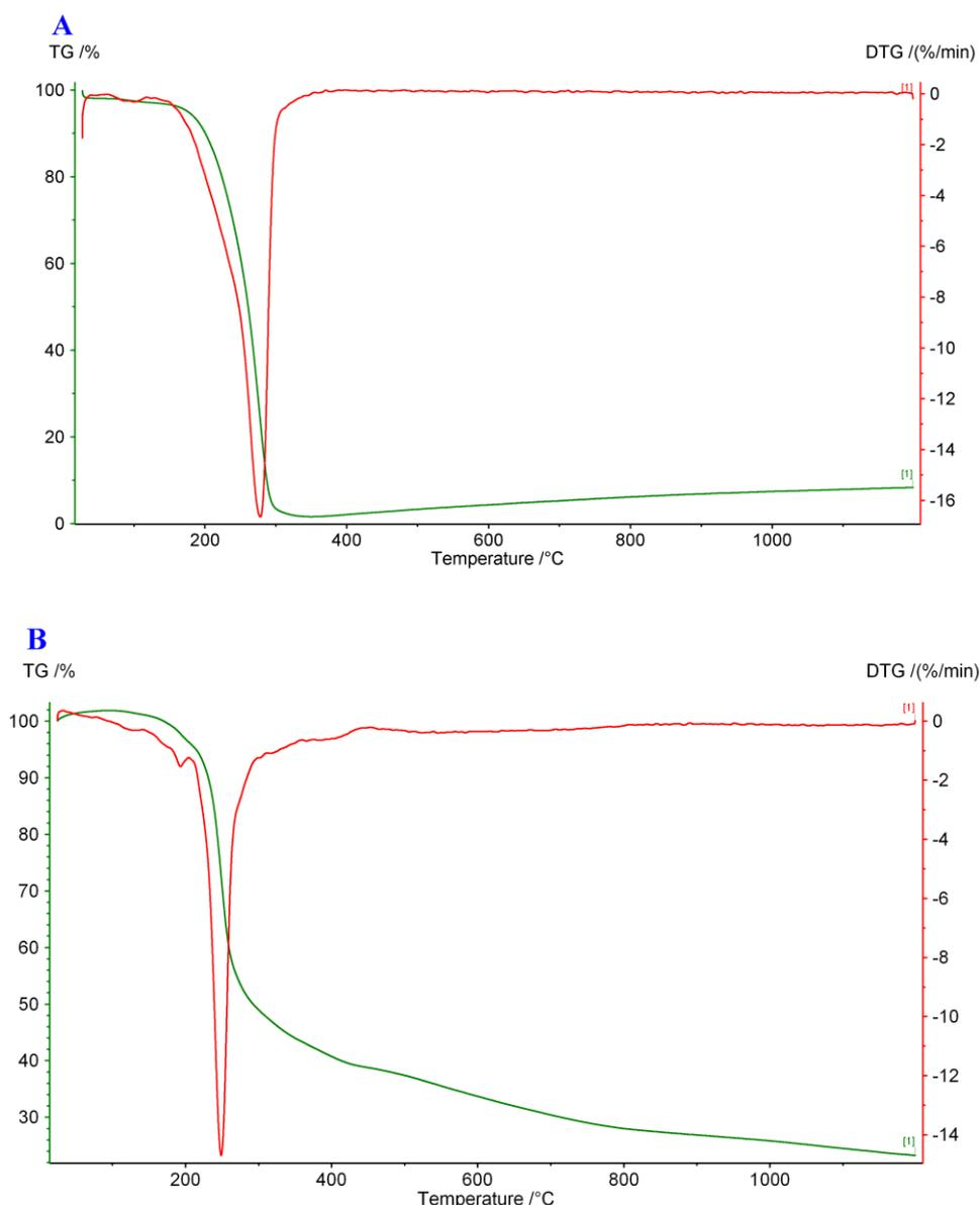
**Figure 6.** TG/DTG curves of (A) [(Eph)(QL)] and (B) [(Eph)(Pi)<sub>2</sub>] CT complexes.
