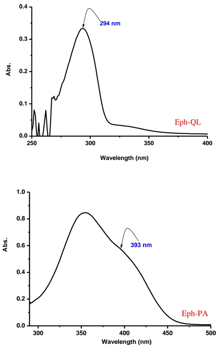
**Figure 1.** Electronic absorption spectra of Eph-QL (294 nm) and Eph-Pi (393 nm) CT complexes.
