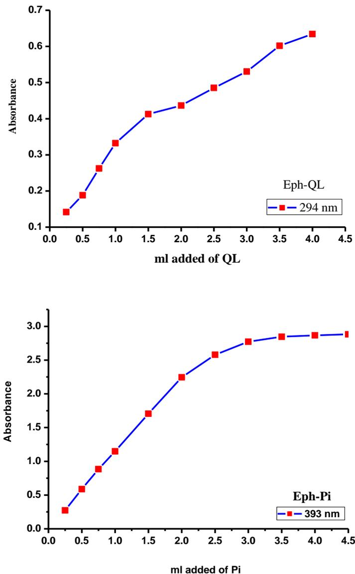
**Figure 2.** Photometric titration curves for Eph-QL and Eph-Pi CT complexes.
