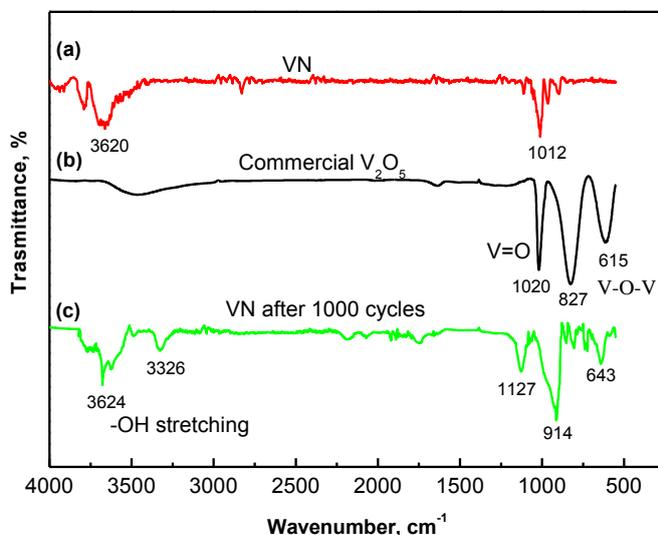
**Figure 8.** FTIR spectra of (a) nanocrystalline VN; (b)  $V_2O_5$  ; (c) VN after 1000 cycles at  $1 \text{ A g}^{-1}$ .
