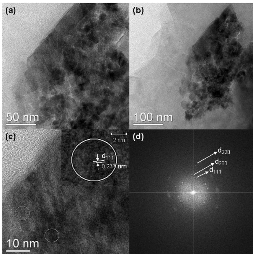
**Figure 2.** (a and b)TEM images of VN sample; (c) HRTEM image of VN sample, inset shows VN nanocrystals; (d) the corresponding powder spectrum of VN sample.
