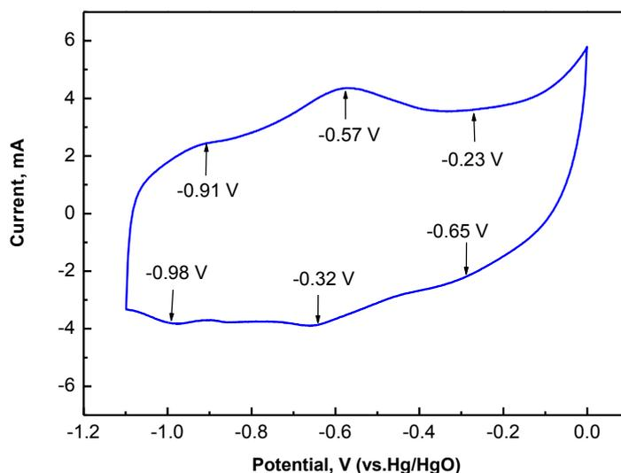
**Figure 5.** CV curve of nanocrystalline VN at the scan rate of  $10 \text{ mV s}^{-1}$  in  $1 \text{ M KOH}$ .
