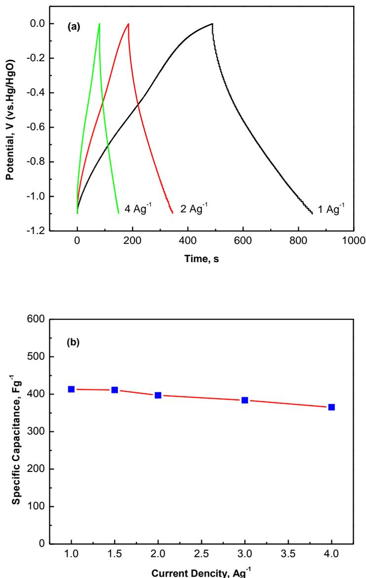
**Figure 6.** (a) The charge-discharge curves of nanocrystalline VN for varying current densities; (b) specific capacitance versus current density.
