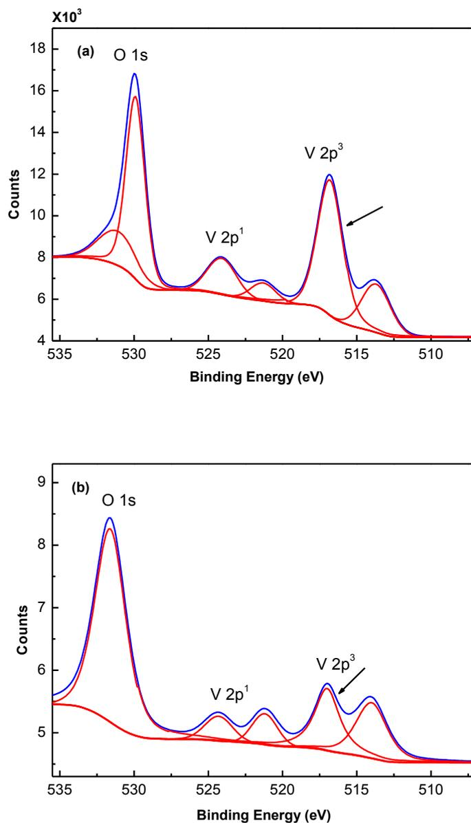
**Figure 9.** XPS spectra of nanocrystalline VN (a) before first cycle and (b) after 1000th cycle at  $1 \text{ A g}^{-1}$  in  $1 \text{ M KOH}$ .
