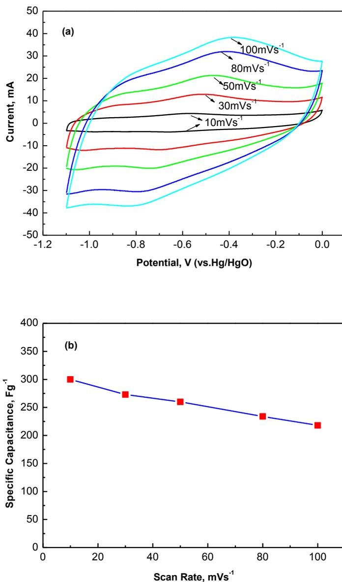
**Figure 4.** (a) CV curves of nanocrystalline VN at different scan rates in 1 M KOH; (b) the specific capacitance versus scan rate.
