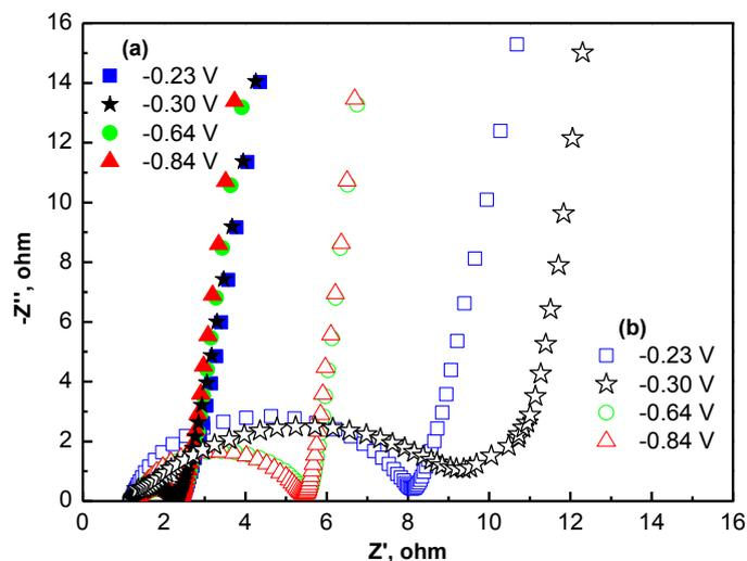
**Figure 10.** Nyquist plots of the nanocrystalline VN electrode between  $10^{-2}$  and  $10^5$  Hz: (a) before first cycle; (b) after 1000th cycle at  $1 \text{ A g}^{-1}$  in  $1 \text{ M KOH}$ .
