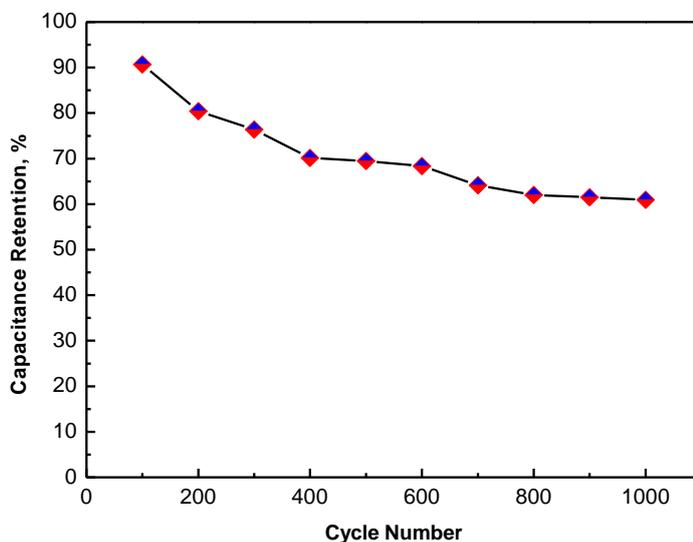
**Figure 7.** Cyclic behavior of VN nanocrystals scanned at current density of  $1 \text{ A g}^{-1}$  up to 1000 cycles in 1M KOH.
