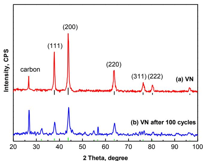
**Figure 1.** The XRD patterns of VN sample (a) before first cycle; (b) after 100th cycle.
