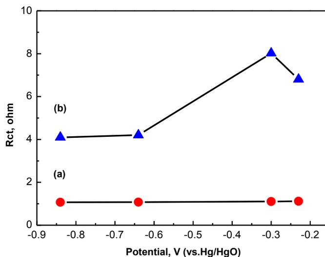
**Figure 11.** The variation of charge-transfer resistance ( $R_{ct}$ ) with potential (a) before first cycle and (b) after 1000th cycle at  $1 \text{ A g}^{-1}$  in  $1 \text{ M KOH}$ .
