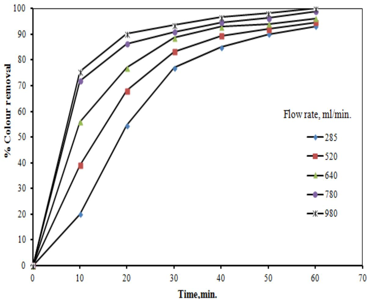
**Figure 6.** Effect of solution flow rate on % Colour removal ( $C_0=50$  mg/l, NaCl=1g/l, pH=7, c.d=  $13.27\text{mA/cm}^2$ , Temperature= $23\pm 2$  °C)
