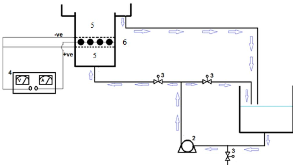
**Figure 1.** Electrochemical oxidation unit (1. Storage tank; 2. Centrifugal pump; 3. Valve; 4. D.C power supply; 5. Stainless steel screen cathode; 6. An array of lead cylinders ( anode))
