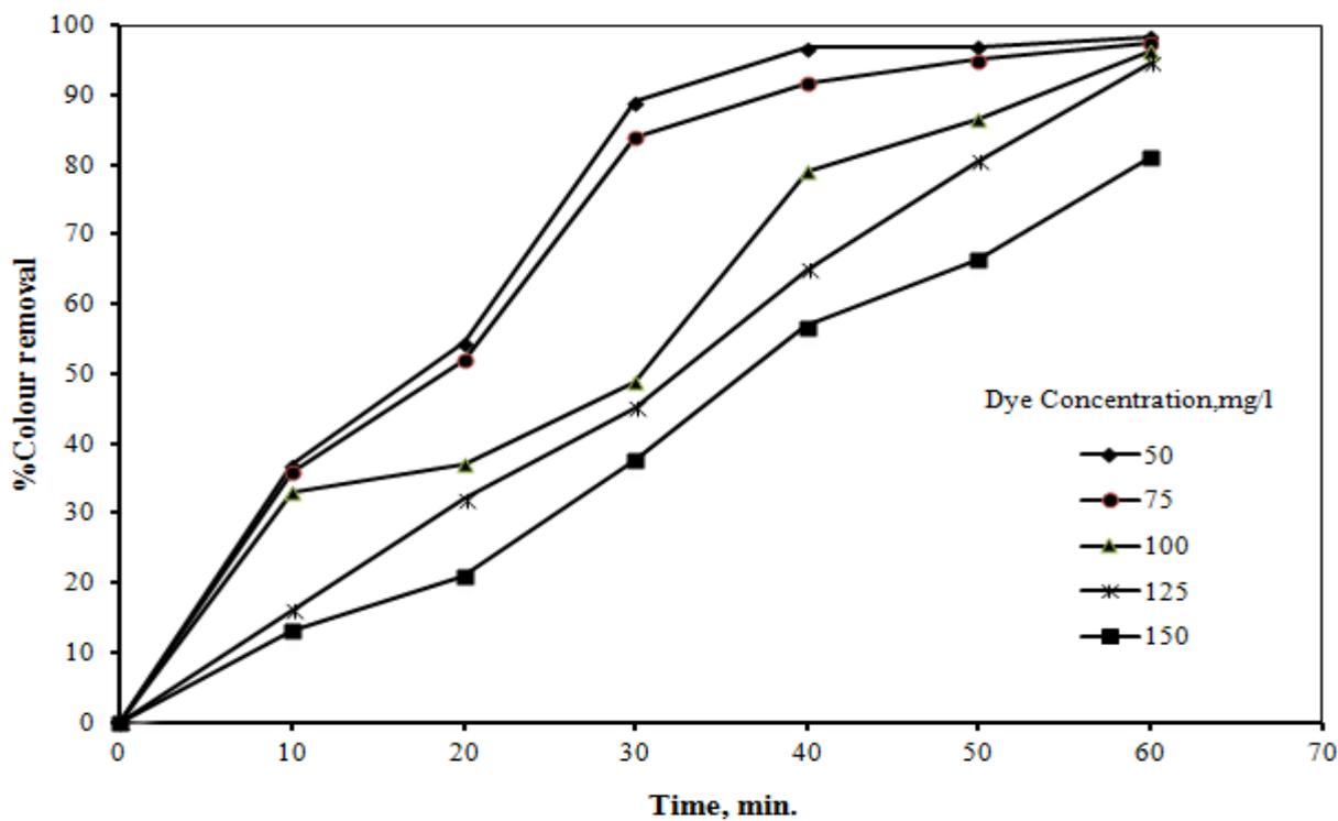
**Figure 3.** Effect of Initial dye concentration on % Colour removal
