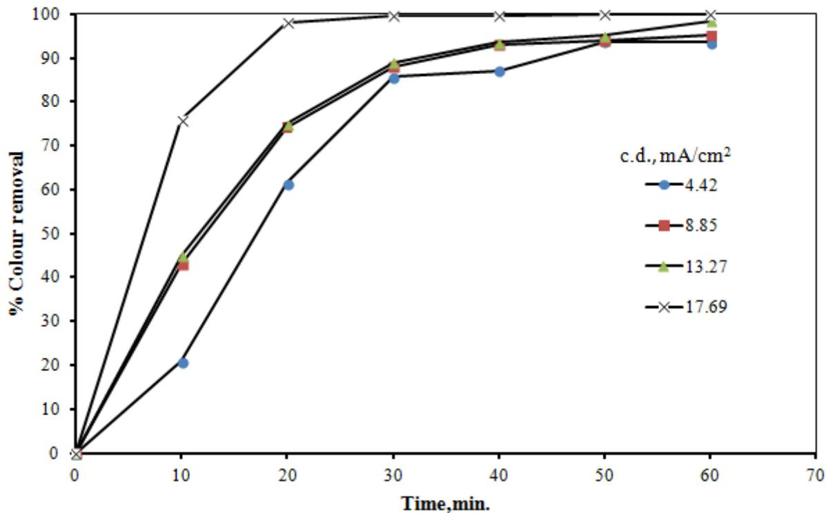
**Figure 2.** Effect of current density on % Colour removal
