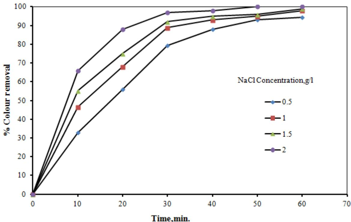
**Figure 4.** Effect of NaCl concentration on % Colour removal ( $C_0=50\text{mg/L}$   $\text{pH}=7$ ,  $c.d = 13.27\text{mA/cm}^2$ , Temperature =  $23\pm 2$  °C, Flow rate =  $285\text{ml/min}$ )
