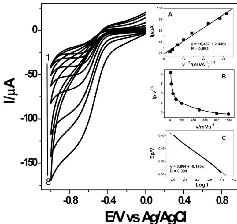
**Figure 9.** Electroreduction of S(IV) using TFcPH<sub>2</sub>/GC modified electrode at pH = 2, at different scan rate (10, 20, 50, 100, 200, 500, 800, 1000 mVs<sup>-1</sup>). Insets: A) I<sub>p</sub> vs v<sup>1/2</sup>; B) normalized current (I<sub>p</sub>v<sup>1/2</sup>) vs v; C) E<sub>p</sub> vs log I.
