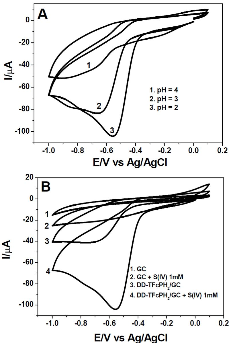
**Figure 8.** Electroreduction of sulfite using drying-drop TFcPH<sub>2</sub>/GC modified electrode: A) different pHs; B) best pH = 2.0.
