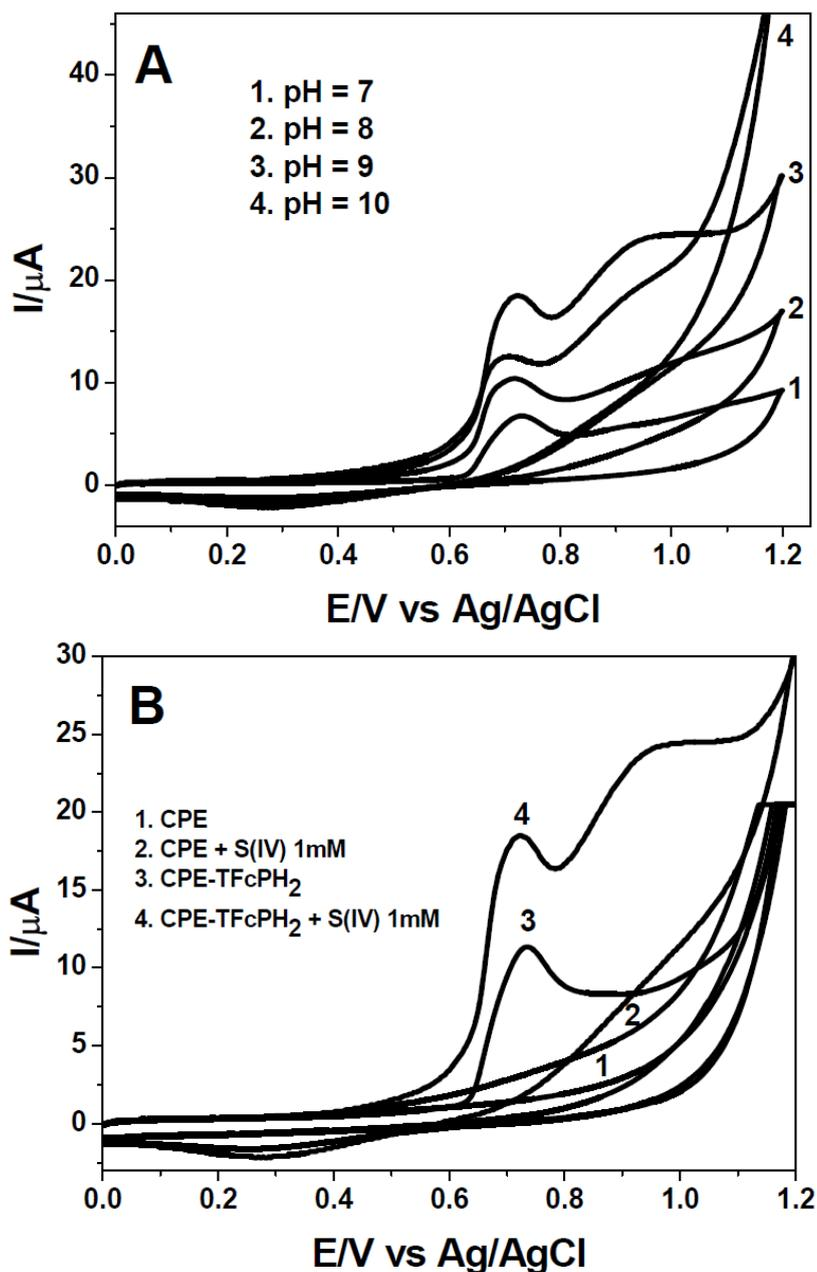
**Figure 7.** Electrocatalytic response of carbon paste/TFcPH<sub>2</sub> modified electrode as redox mediator for sulfite oxidation: A) pH (7,8,9,10); B) best pH = 9.
