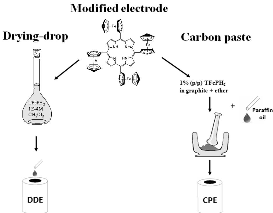
**Figure 2.** Preparation of the modified electrodes.
