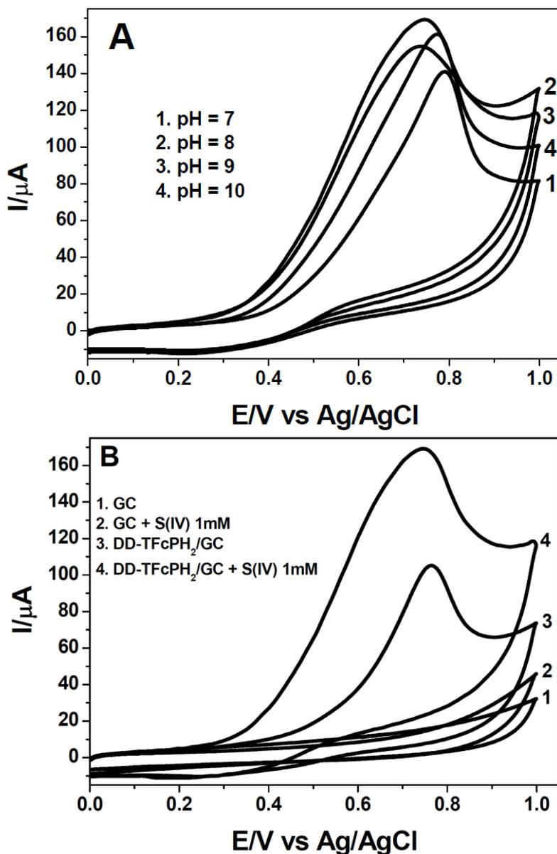
**Figure 6.** Electro-oxidation of sulfite using drying-drop TFcPH<sub>2</sub>/GC modified electrode: A) different pHs (7,8,9,10); B) best pH = 9.
