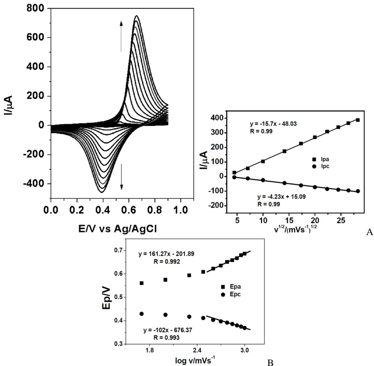
**Figure 4.** Voltammetric response of the drying-drop modified electrode TFCpPH<sub>2</sub>/GC A)  $I_p$  vs  $v^{1/2}$ ; B)  $E_p$  vs  $\log v$ .
