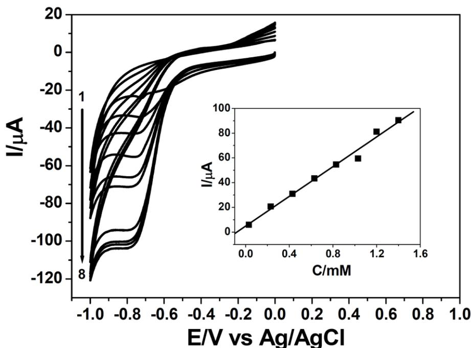
**Figure 10.** Electroreduction of S(IV) using TFcPH<sub>2</sub>/GC modified electrode at pH = 2, at different concentration (0.03, 0.2, 0.4, 0.6, 0.8, 1.0, 12, 1.4 mM). Inset: Calibration plot illustrating the linear response to S(IV) (I<sub>p</sub>/ μA vs C/mM).
