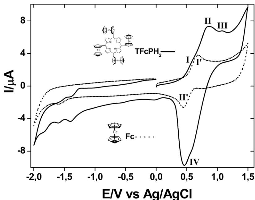
**Figure 3.** Cyclic voltammetry for TFcPH<sub>2</sub> (continuous line) and Ferrocene (dashed line) in CH<sub>2</sub>Cl<sub>2</sub> solution containing tetrabutyl ammonium perchlorate (TBAP) under nitrogen. Scan rate 100 mVs<sup>-1</sup>
