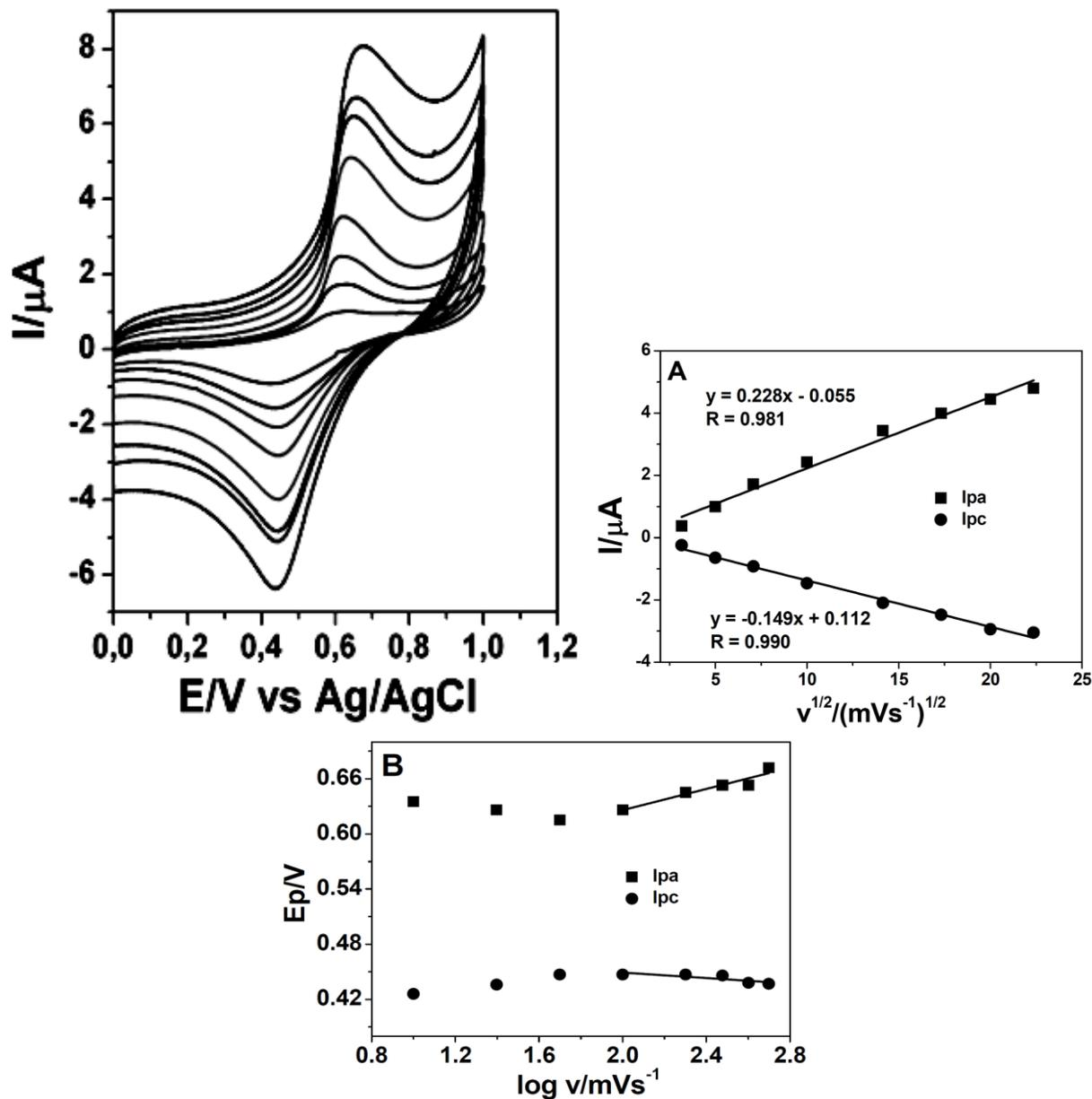
**Figure 5.** Voltammetric response of the carbon paste /TFcPH<sub>2</sub> modified electrode. A)  $I_p$  vs  $v^{1/2}$ ; B)  $E_p$  vs  $\log v$ .
