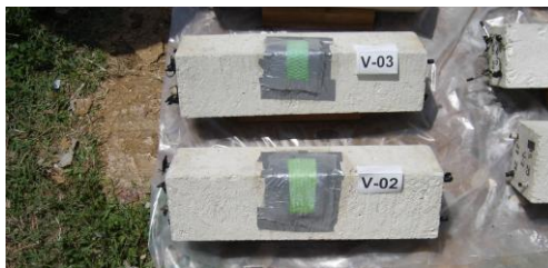
Figure 4. Sketch (a) and photo (b) of beams during wet and dry cycles
