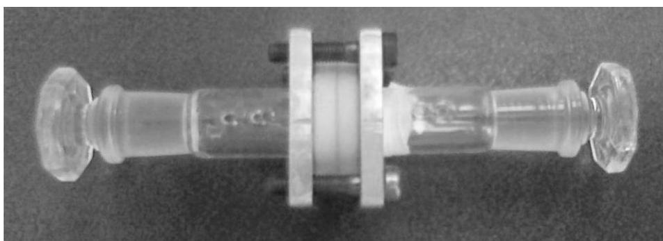
**Figure 1.** Electrochemical “Glass” cell, “Compartment 1” on the right.
