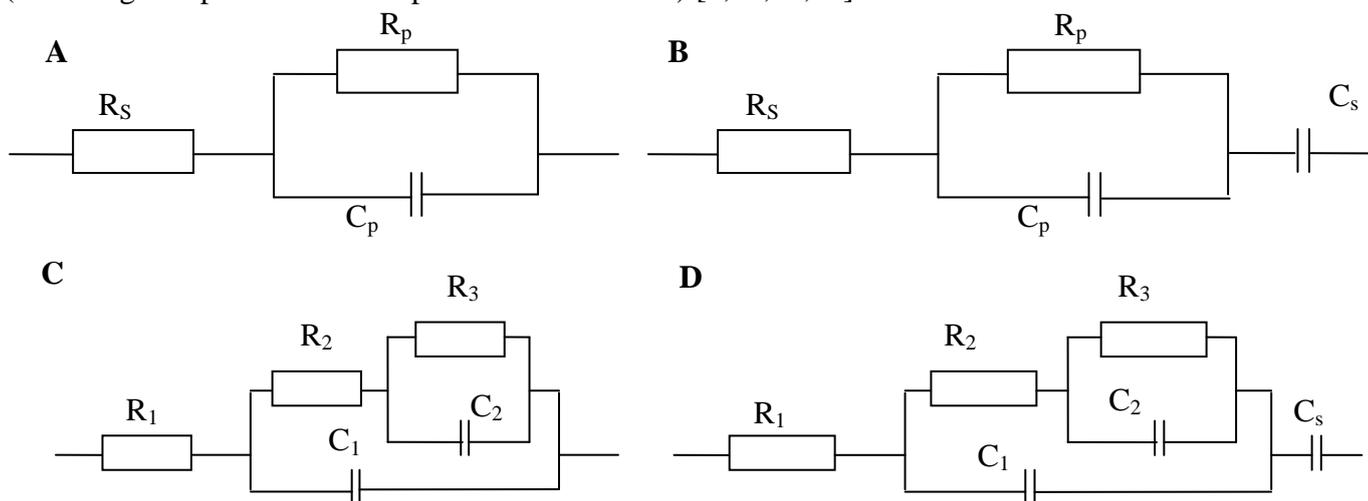
**Figure 2.** Electrical equivalent circuits used for characterization of SPL membranes formed on polymer surfaces.
