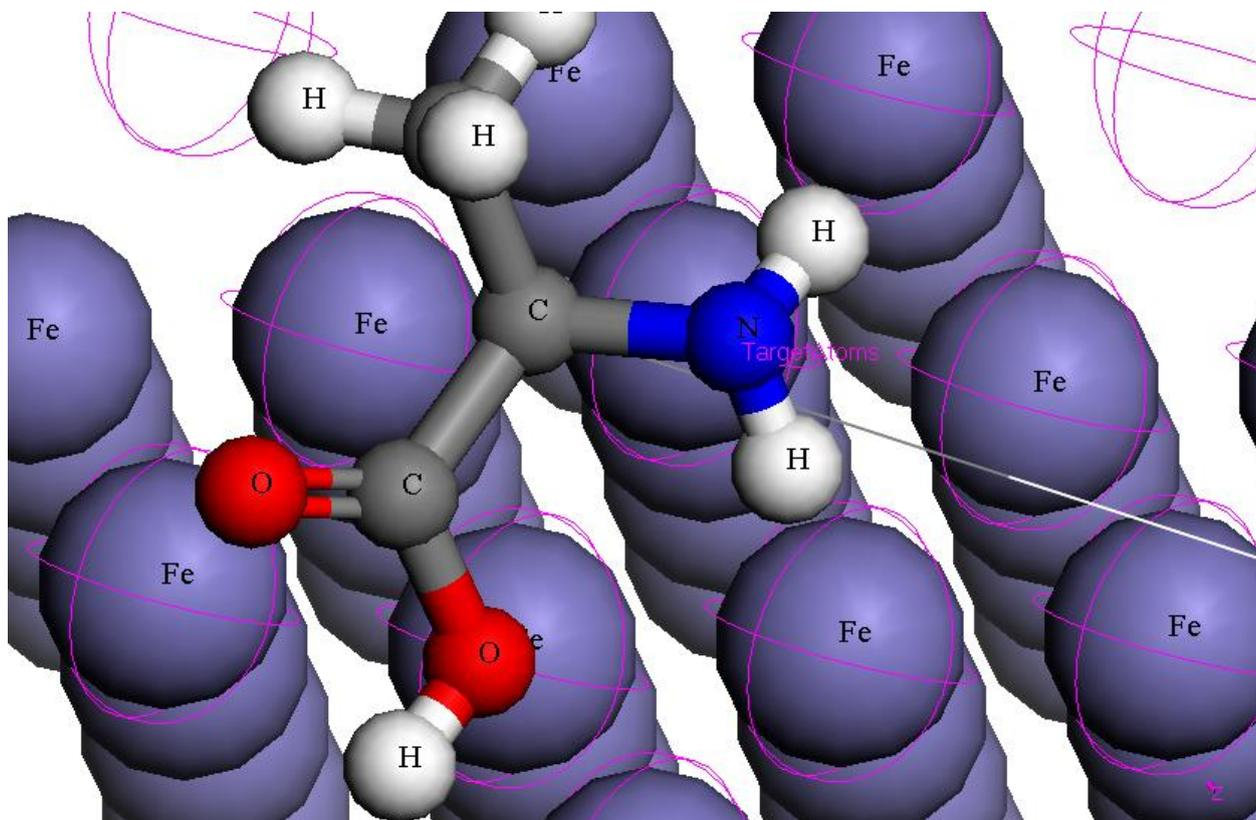
**Figure 2.** Most suitable configuration for adsorption of alanine on Fe(111) substrate obtained by adsorption locator module[22, 28, 29]
