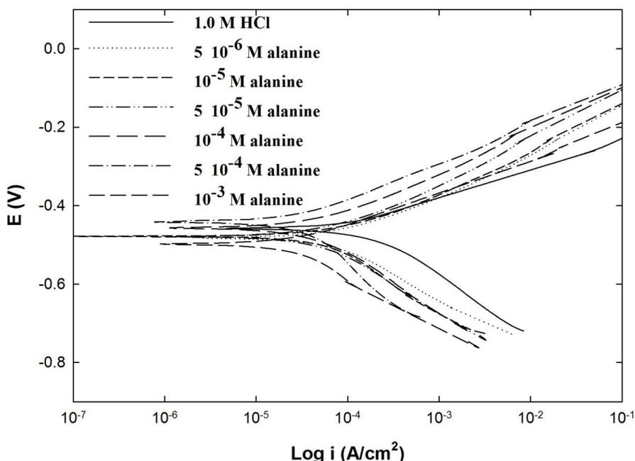
**Figure 6.** Anodic and cathodic polarization curves for iron in 1.0 M HCl solutions in the absence and presence of various concentrations of alanine at 25 ± 1 °C.
