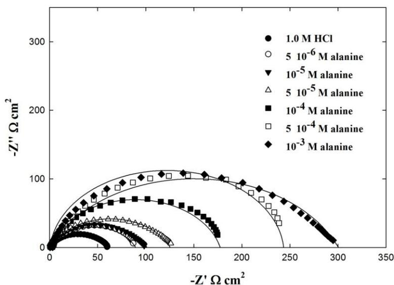
**Figure 7.** Nyquist plots for iron in 1.0 M HCl solutions in the absence and presence of various concentrations of alanine at  $25 \pm 1 \text{ }^\circ\text{C}$ , solid line represent fitted data obtained by equivalent circuit in Fig. 8.
