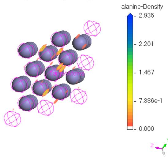
**Figure 3.** Adsorption density field of alanine on the Fe (1 1 1) substrate.
