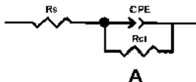
**Figure 8.** Equivalent circuit model for iron /1.0 M HCl interface.
