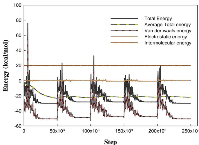
Figure 4. Total energy distribution of adsorbate (alanine)- adsorbent (iron) system.
