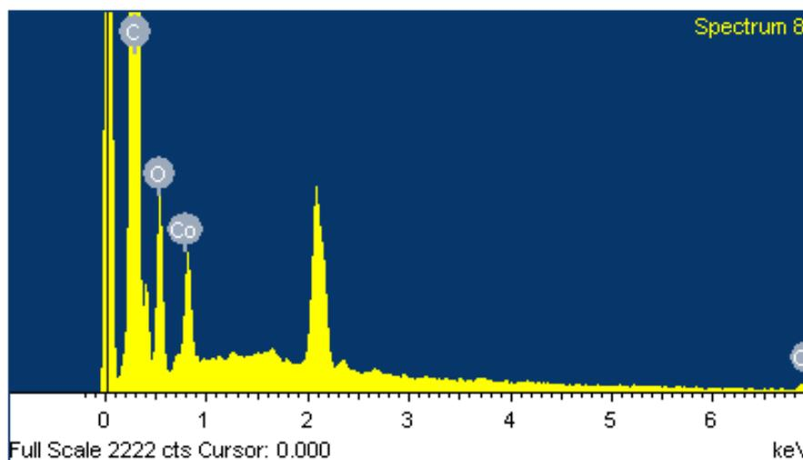
**Figure 3.** EDX spectra of Cobalt oxide/CNF nanocomposite.
