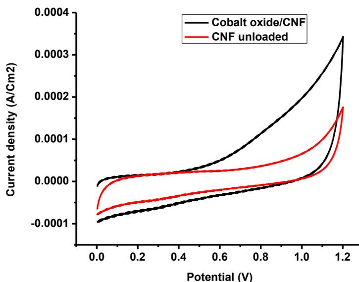
**Figure 7.** Cyclic voltammograms of Cobalt oxide/CNF and unloaded CNF electrocatalysts prepared by in (0.6 M MeOH + 0.5 M H<sub>2</sub>SO<sub>4</sub>) solution The potential range is from 0 to +1.2 V at 100 mV s<sup>-1</sup>.
