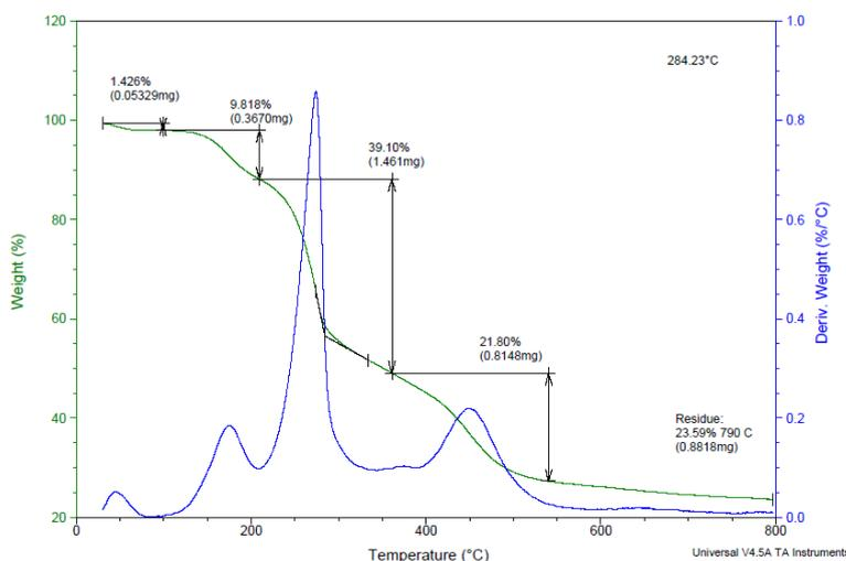
**Figure 1.** The TGA-thermogram in nitrogen atmosphere for PVA electrospun nanofibers
