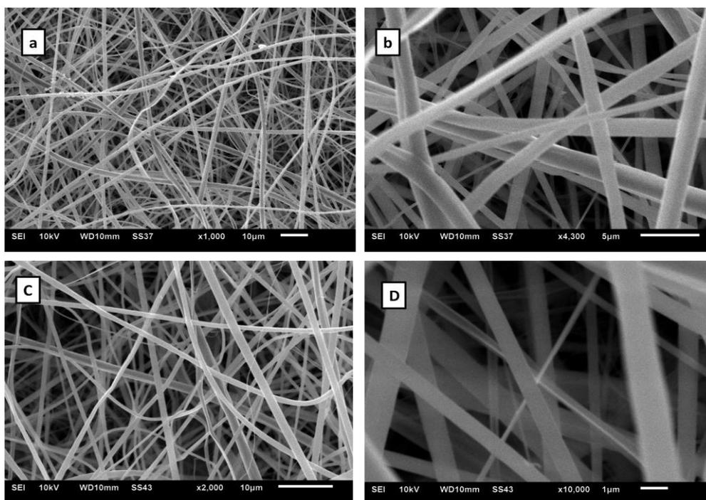
**Figure 2.** SEM images of PVA nanofibers before carbonization (a,b) and after carbonization(c,d)
