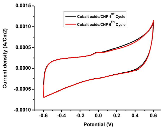
**Figure 6.** Repeated CVs of Cobalt oxide/CNF in a solution of  $1 \text{ M KOH}$  at a scan rate of  $100 \text{ mV s}^{-1}$ .
