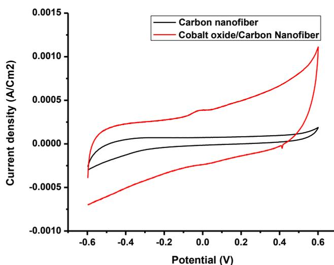
**Figure 5.** CV curves of (a) pure carbon nanofibers and Cobalt oxide/CNF electrodes at sweep rate of  $50 \text{ mV s}^{-1}$
