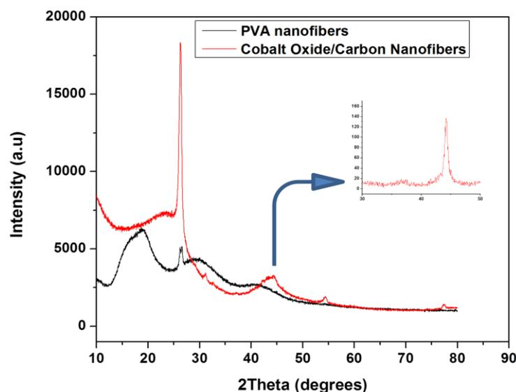
**Figure 4.** XRD pattern of PVA nanofibers and Cobalt Oxide/CNF nanocomposite .
