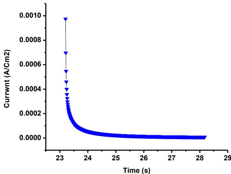
**Figure 8.** Chronoamperograms of Cobalt oxide/CNF at potential values of 0.3 V in (0.6 M MeOH + 0.5 M H<sub>2</sub>SO<sub>4</sub>) solution.
