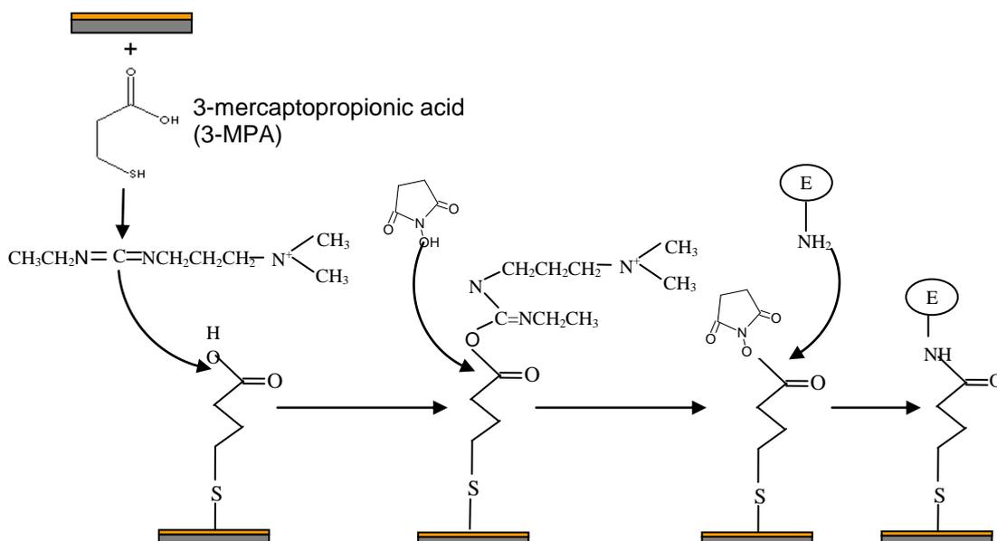
**Figure 2.** The immobilization sequences of the 3-MPA, EDC, NHS and lipase.
