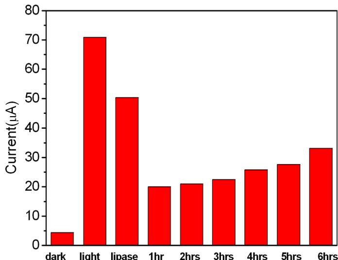
**Figure 7.** PN diode current characteristics plot of dark, light, lipase immobilized and transesterification react from 1 to 6 hours.
