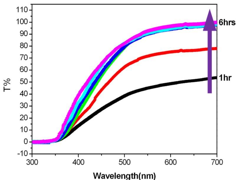
**Figure 4.** Transmittance characteristics of each reaction time (1 to 6 hours).
