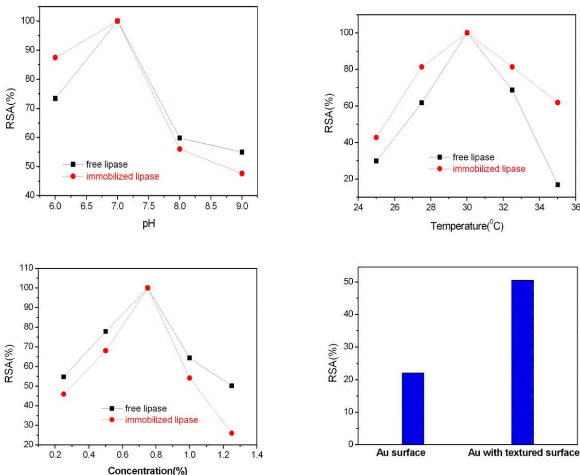
**Figure 5.** Relative specific activity (RSA) of comparison characteristics of free and immobilized lipase (a) with different pH values, (b) with different temperatures, (c) with different lipase concentrations, and (d) different substrates.
