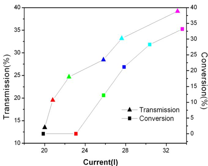
**Figure 8.** The relationship of the transesterification reaction compared with the current by PN diode, transmission by UV-Vis and conversion yield by NMR. The curves with (▲) and (■) represent the relationship with transmission v.s. current and conversion yield v.s. current respectively. The symbols represent transesterification react from 1 to 6 hours.
