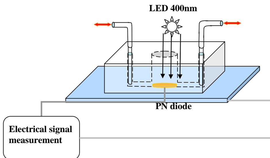
**Figure 1.** Concept of photoelectrical approach of on chip transesterification reaction detection technique.
