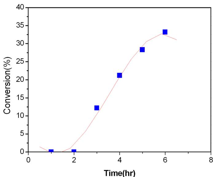
**Figure 6.** Conversion yield–time characteristics of  $^1\text{H-NMR}$  measurement with transesterification react from 1 to 6 hours.
