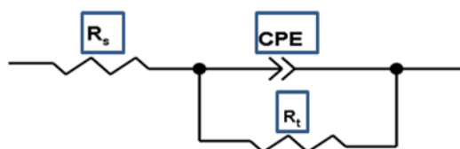
Figure 6. Equivalent electrical circuit used to fit impedance data
