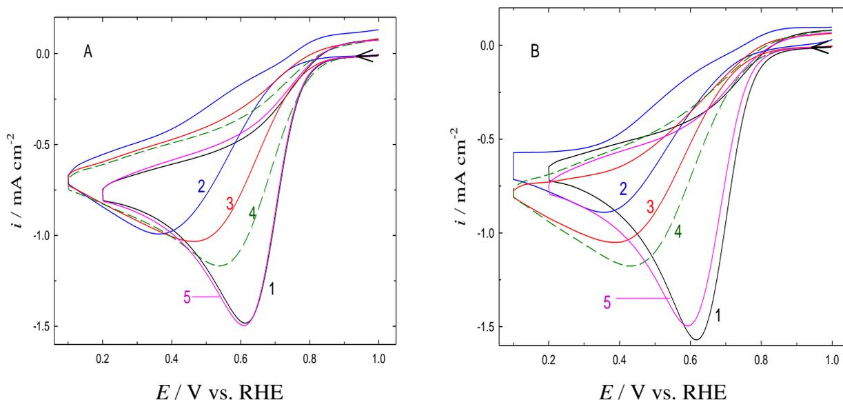
**Figure 5.** ORR in  $\text{SO}_2$ -free 0.1 M  $\text{H}_2\text{SO}_4$  on the GC/nano-Pt electrode. (1) fresh electrode, (2) poisoned (3) and (4) after the 5<sup>th</sup> and the 10<sup>th</sup> cycles of the short-range recovery, respectively and (5) after the long-range recovery. Average Pt particles size: (A) 40 and (B) 90 nm.
