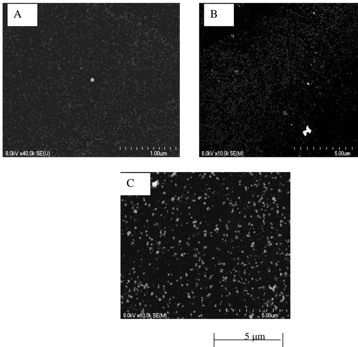
**Figure 1.** SEM images of GC/nano-Pt electrodes. Average Pt particles sizes: (A) 20, (B) 40 and (C) 90 nm.
