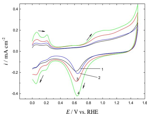
**Figure 2.** CVs obtained at the GC/nano-Pt electrodes with different sizes of the Pt particles in  $\text{N}_2$ -saturated  $0.1 \text{ M H}_2\text{SO}_4$ . Average particle sizes: (1) 40, (2) 90, (3) 190 and (4) 480 nm. Potential scan rate :  $0.1 \text{ V s}^{-1}$ .
