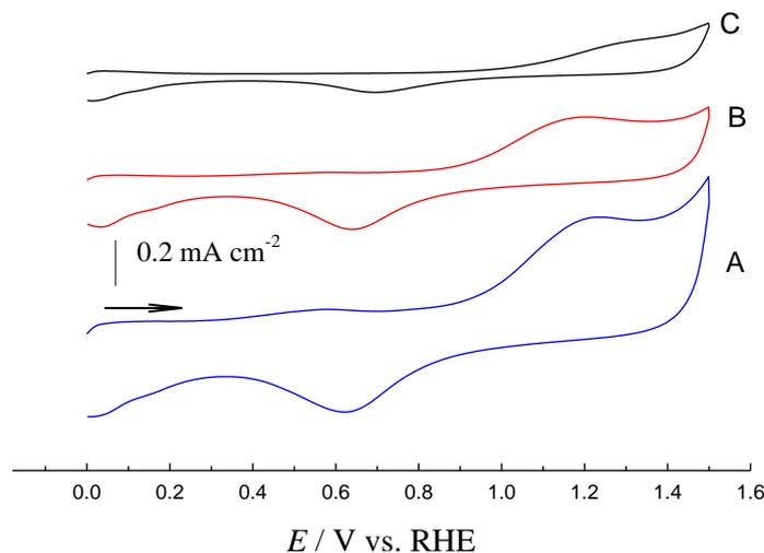
**Figure 10.** CVs obtained at the poisoned GC/nano-Pt electrodes with average Pt particle sizes of (A) 40 and (B) 90 nm and (C) at the poly-Pt electrode in  $N_2$ -saturated 0.1 M  $H_2SO_4$ . Potential scan rate:  $0.1 \text{ V s}^{-1}$ .
