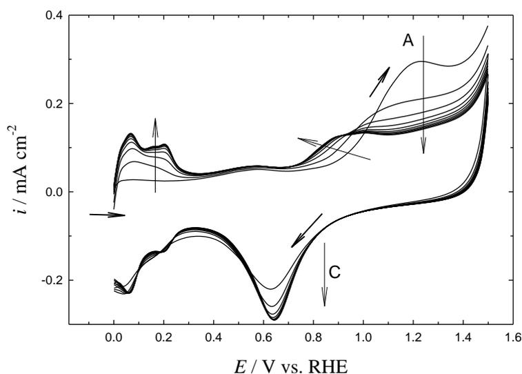
**Figure 4.** Sequence of CVs obtained at the poisoned GC/nano-Pt electrode with average particle size of 190 nm in  $N_2$ -saturated 0.1 M  $H_2SO_4$ . Potential scan rate :  $0.1 \text{ V s}^{-1}$ .
