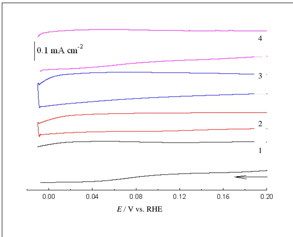
**Figure 9.** CVs of the  $H_{\text{ads/des}}$  on the GC/nano-Pt (average Pt particle size: 40 nm) in  $N_2$ -saturated 0.1 M  $H_2SO_4$ : (1) fresh electrode, (2) poisoned electrode, (3) after short-range recovery and (4) after long-range recovery.
