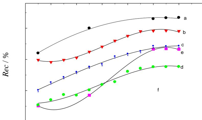
**Figure 6.** Percentage current recovery change of the ORR peak current with the number of potential cycles in the short-range recovery (1.0 to 0.1 V) obtained at GC/nano-Pt electrodes with different platinum nanoparticles sizes: (a) 20, (b) 40, (c) 90 and (d) 480 nm. (e) was obtained at poly-Pt electrode.
