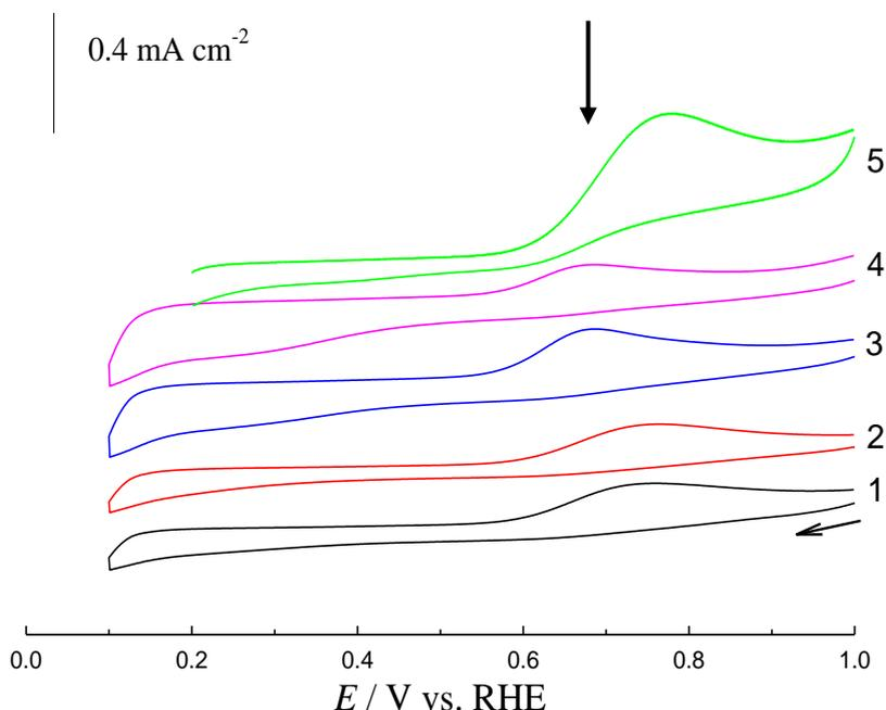
**Figure 3.** CVs obtained at GC/nano-Pt electrodes in  $\text{N}_2$ -saturated 0.1 M  $\text{H}_2\text{SO}_4$  containing  $5 \times 10^{-4}$  M  $\text{SO}_2$ . Average particle sizes: (1) 40, (2) 90, (3) 190 and (4) 480 nm. Curve 5 is the results obtained at poly-Pt electrode. Potential scan rate :  $0.1 \text{ V s}^{-1}$ .
