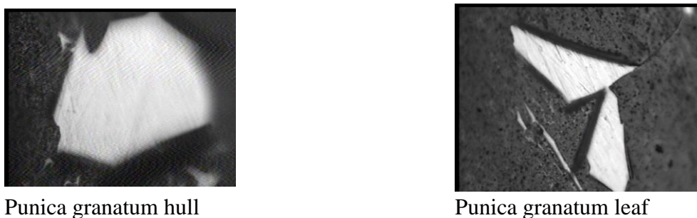
Figure 4. Optical micrograph photo (40X) for cathodically polarized steel in \text{CaCl}_2 brine solution in the presence of 100 ppm of extracts after 21 hours at 40^\circ\text{C} with film scratching.
