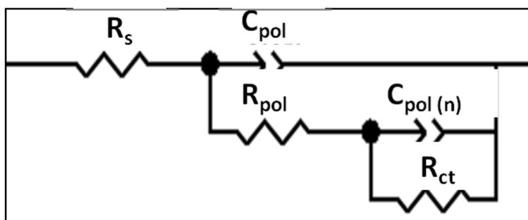
**Figure 5.** Equivalent circuit used in the analysis of electrochemical impedance data.  $R_s$  (strength solution) and  $C_{pol}$ ,  $C_{pol}(n)$  (polymer solution interface and electrode solution interface, respectively) and  $R_{ct}$ ,  $R_{pol}$  (resistance of the charge transfer of the polymer and of the double layer, respectively).
