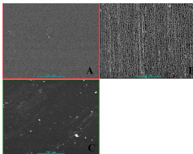
**Figure 6.** SEM images of Au electrode / polyCoTAPP (A), PoPD (B) and copolymer (C), magnification 500X.
