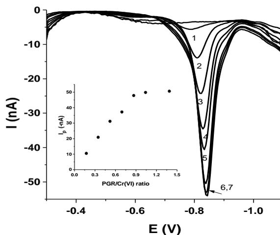
**Figure 1.** Adsorptive voltammograms of Cr(VI) solutions in the presence of aliquots of PGR, and plot of  $I_{\text{peak}}$  vs. Cr:PGR ratio. Conditions:  $pH = 4.5$  ( $4 \text{ mmol L}^{-1}$  acetic buffer);  $C_{\text{Cr(VI)}} = 0.19 \mu\text{mol L}^{-1}$ ;  $C_{\text{PGR}} = 0.0$  to  $0.28 \mu\text{mol L}^{-1}$ ;  $E_{ads} = -0.68$  V;  $t_{ads} = 60$  s; voltage step = 5 mV; amplitude = 10 mV; frequency = 25 Hz and scan rate  $126 \text{ mV s}^{-1}$  (mode SWV)
