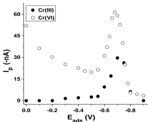
**Figure 6.** Effect of adsorptive potential ( $E_{ads}$ ) on the peak current of the Cr<sup>III</sup>–PGR complex. (●)  $C_{Cr(III)} = 9.8 \mu\text{g L}^{-1}$ . (○)  $C_{Cr(VI)} = 9.8 \mu\text{g L}^{-1}$ . Conditions:  $pH=4.5$ ;  $C_{PGR} = 0.25 \mu\text{mol L}^{-1}$ ;  $t_{ads} = 60$  s.
