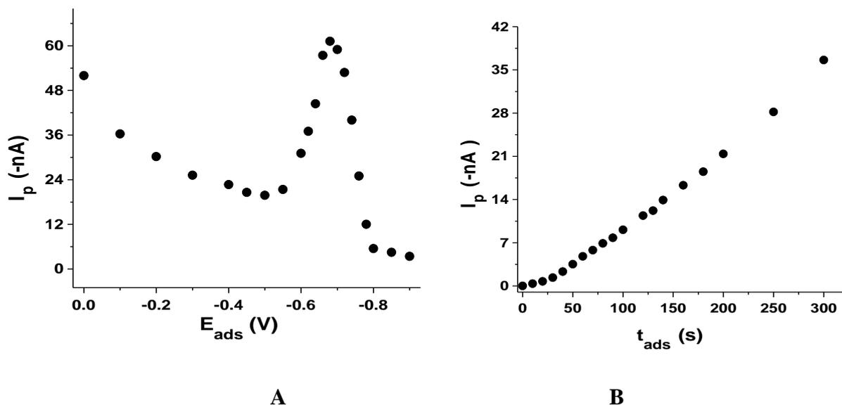
**Figure 4.** Effect of adsorptive potential ( $E_{ads}$ ) (A) and time ( $t_{ads}$ ) (B) on the peak current of the  $\text{Cr}^{\text{III}}$ -PGR complex. Conditions:  $\text{pH} = 4.5$  (acetic buffer);  $C_{\text{Cr(VI)}} = 9.8 \mu\text{gL}^{-1}$ ;  $C_{\text{PGR}} = 0.25 \mu\text{mol L}^{-1}$ ; (A)  $t_{ads} = 60$  s; (B)  $E_{ads} = -0.68$  V.
