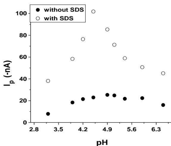
**Figure 2.** Effect of pH on the peak current of the  $\text{Cr}^{\text{III}}$ –PGR complex in the absence (●) and presence (○) of SDS ( $9.8 \mu\text{mol L}^{-1}$ ). Conditions:  $C_{\text{Cr(VI)}}=9.8 \mu\text{g L}^{-1}$ ;  $C_{\text{PGR}}=0.32 \mu\text{mol L}^{-1}$ ;  $E_{\text{ads}}=-0.40 \text{ V}$ ;  $t_{\text{ads}}=60 \text{ s}$ .
