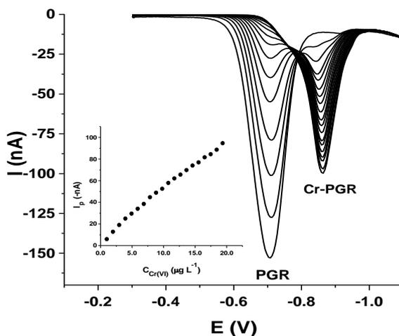
**Figure 5.** Adsorptive voltammograms and calibration curves for the  $\text{Cr}^{\text{III}}$ -PGR complex. Conditions:  $\text{pH} = 4.5$  (acetic buffer);  $C_{\text{PGR}} = 2.7 \mu\text{mol L}^{-1}$ ;  $E_{ads} = -0.68$  V;  $t_{ads} = 60$  s. Other conditions as in Fig. 1.
