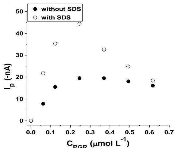
**Figure 3.** Effect of ligand concentration on the peak current of the Cr<sup>III</sup>-PGR complex in the absence (●) and presence (○) of SDS. Conditions:  $pH = 4.5$  (acetic buffer);  $C_{Cr(VI)} = 9.8 \mu\text{g L}^{-1}$ ;  $C_{SDS} = 2.0 \mu\text{g L}^{-1}$ ;  $t_{ads} = 60 \text{ s}$ ;  $E_{ads} = -0.40 \text{ V}$ .
