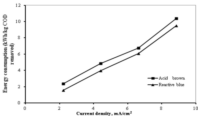
**Figure 7.** Effect of current density on energy consumption (NaCl = 15 g/l, flow rate = 765 cm<sup>3</sup>/min, Time = 80 min., C<sub>0</sub> = 100 mg/l, pH = 7, Temp. = 25 °C)
