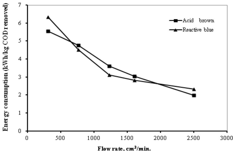
**Figure 9.** Effect of solution flow rate on energy consumption (c.d = 6.63 mA/cm<sup>2</sup>, NaCl = 15 g/l, Time = 80 min., C<sub>0</sub>= 100 mg/l, pH = 7, Temp. =25 °C)
