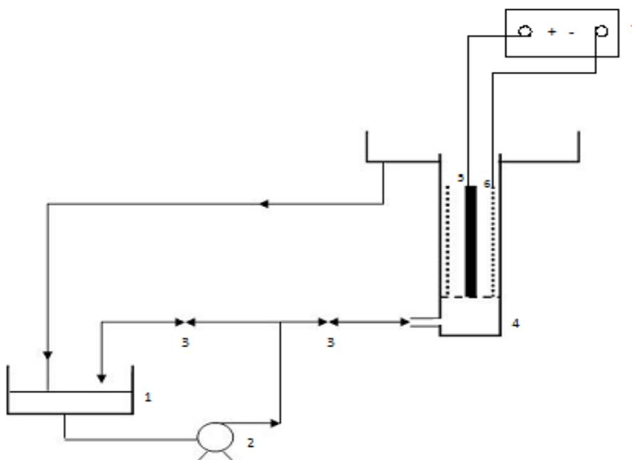
**Figure 1.** Electrochemical oxidation cell 1. Storage tank 2. Centrifugal pump 3. Valve 4. Cylindrical plexi glass column 5. Graphite rod anode 6. Stainless steel cathode 7. D.C.power supply
