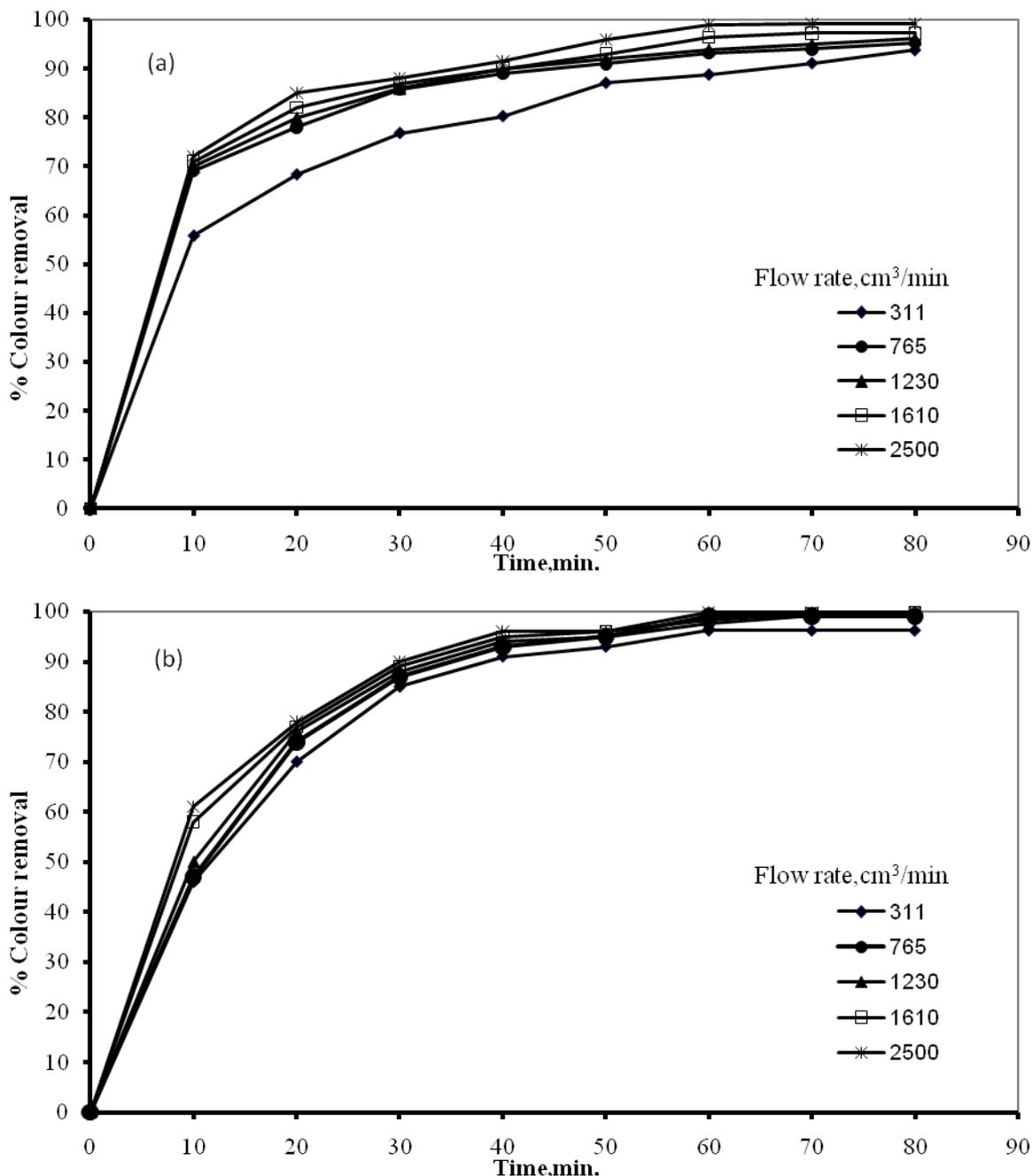
**Figure 6.** Effect of solution flow rate on efficiency of colour removal (NaCl = 15 g/l, c.d = 6.63 mA/cm<sup>2</sup>, C<sub>0</sub>= 100 mg/l, pH = 7, Temp. =25 °C) a. Acid brown b. Reactive blue
