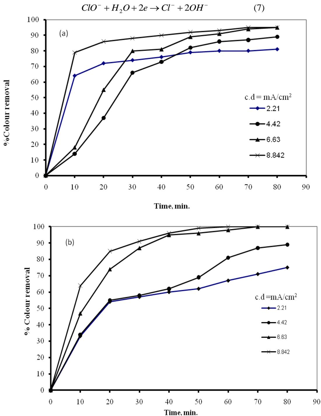
**Figure 2.** Effect of current density on efficiency of colour removal ( $C_0=100$  mg/l, NaCl=15g/l, pH=7, flow rate=  $765$  cm<sup>3</sup>/min, Temp. =25 °C) a. Acid brown b. Reactive blue
