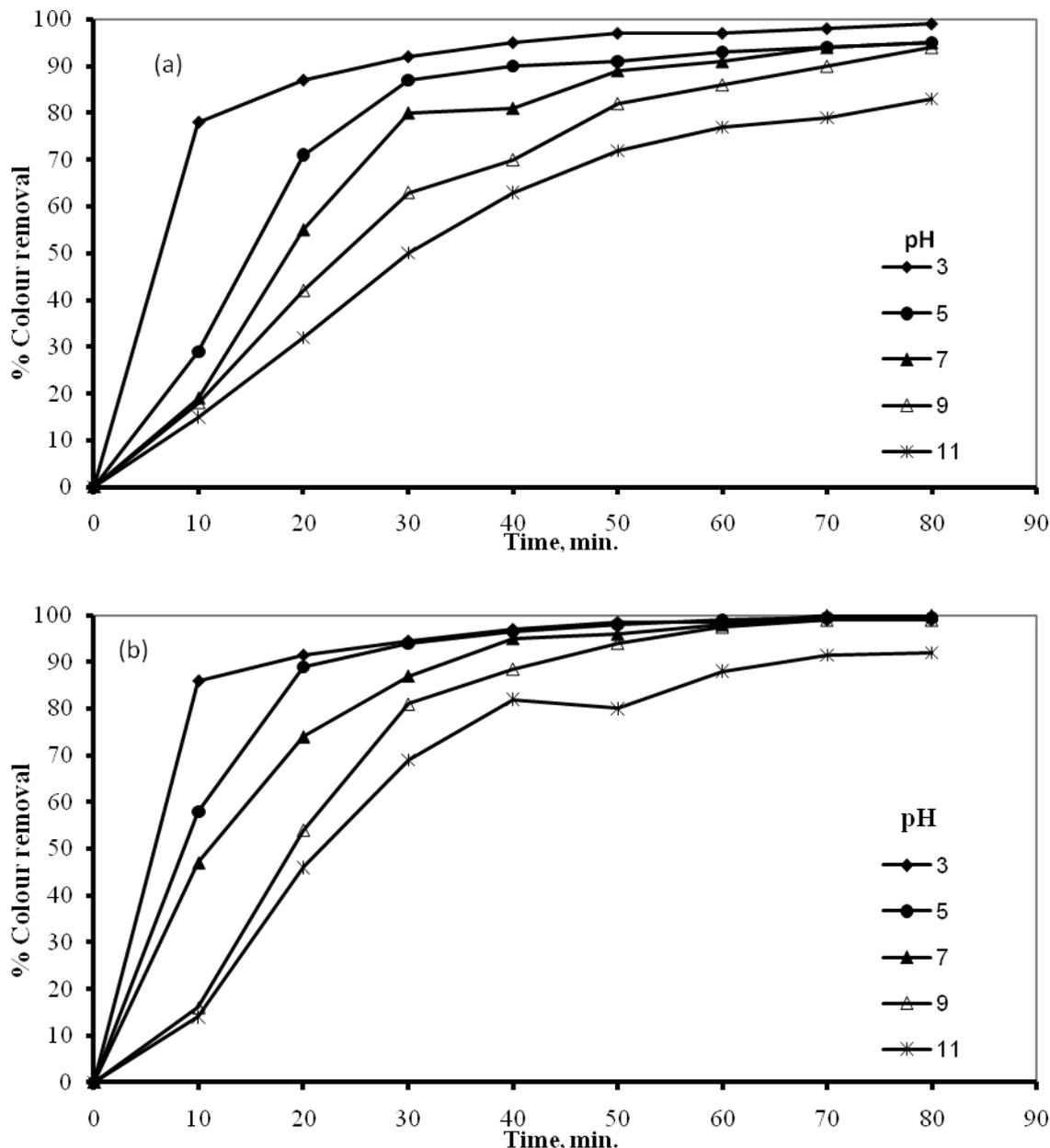
**Figure 5.** Effect of initial pH on efficiency of colour removal (NaCl = 15 g/l, c.d = 6.63 mA/cm<sup>2</sup>, C<sub>0</sub>= 100 mg/l, flow rate= 765 cm<sup>3</sup>/min, Temp. =25 °C) a. Acid brown b. Reactive blue
