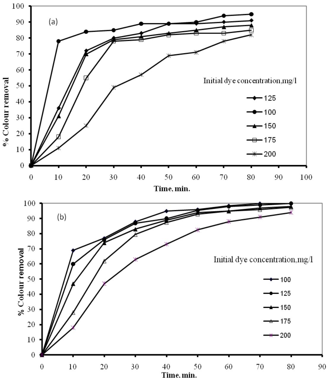
**Figure 4.** Effect of initial dye concentration on efficiency of colour removal (NaCl = 15 g/l, c.d = 6.63 mA/cm<sup>2</sup>, pH=7, flow rate= 765 cm<sup>3</sup>/min, Temp. =25 °C) a. Acid brown b. Reactive blue
