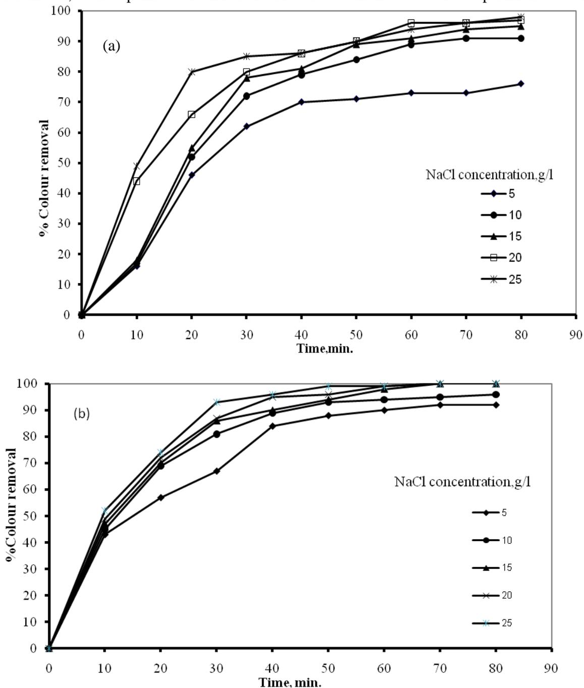
**Figure 3.** Effect of NaCl concentration on efficiency of colour removal ( $C_0=100 \text{ mg/l}$ ,  $c.d = 6.63 \text{ mA/cm}^2$ ,  $\text{pH}=7$ , flow rate=  $765 \text{ cm}^3/\text{min}$ , Temp. =  $25 \text{ }^\circ\text{C}$ ) a. Acid brown b. Reactive blue
