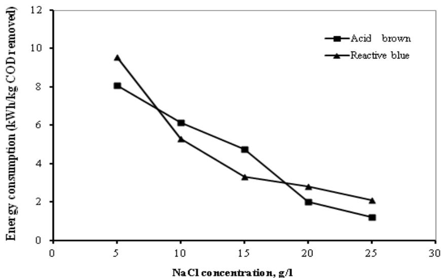
**Figure 8.** Effect of NaCl concentration on energy consumption (c.d = 6.63 mA/cm<sup>2</sup>, flow rate = 765 cm<sup>3</sup>/min, Time = 80 min., C<sub>0</sub>= 100 mg/l, pH = 7, Temp. =25 °C)
