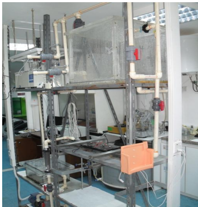
Figure 1. Single compartment electrochemical reactor connected to the flow system used in conducting the experiments .
