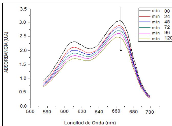
**Figure 4.** Variation of absorption spectrum of methylene blue depends on the illumination time.
