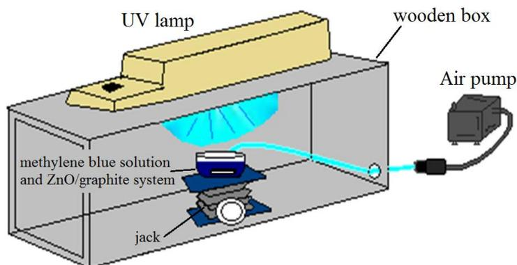
**Figure 1.** Schematic diagram of the system used for the methylene blue degradation.
