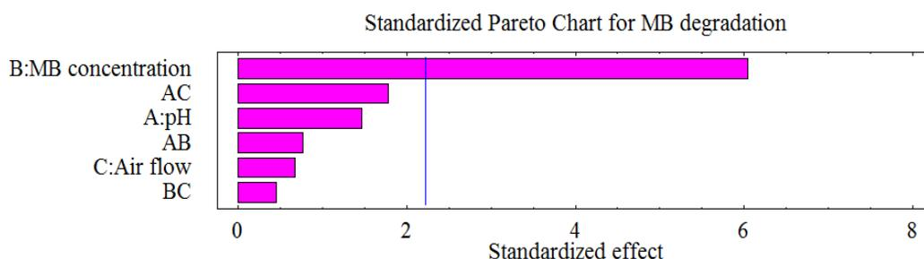
**Figure 5.** Standardized Pareto chart for the response variable (MB degradation) of the experimental design.
