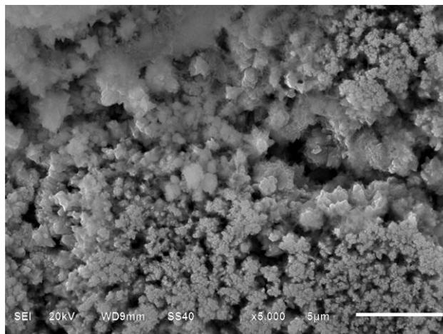
**Figure 3.** Micrograph of the ZnO/graphite system obtained by SEM.
