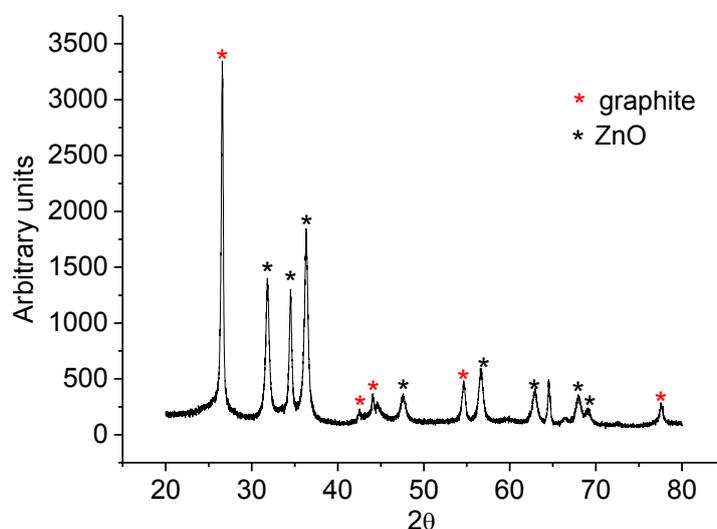
**Figure 2.** Diffractogram of the ZnO/graphite system.
