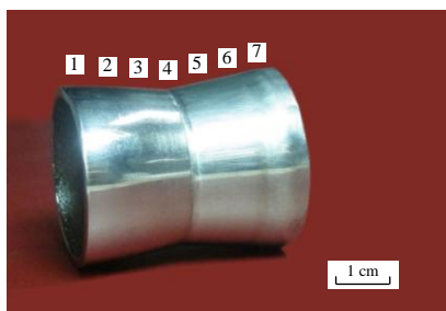
Figure 8. Photo of the nickel thin-walled part prepared by PJED.
