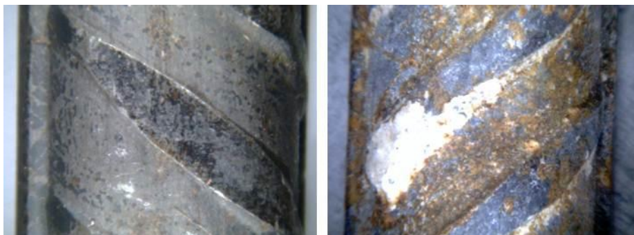
Figure 7. Surface appearance of the carbon steel at the beginning of the experiment and after 49 days.
