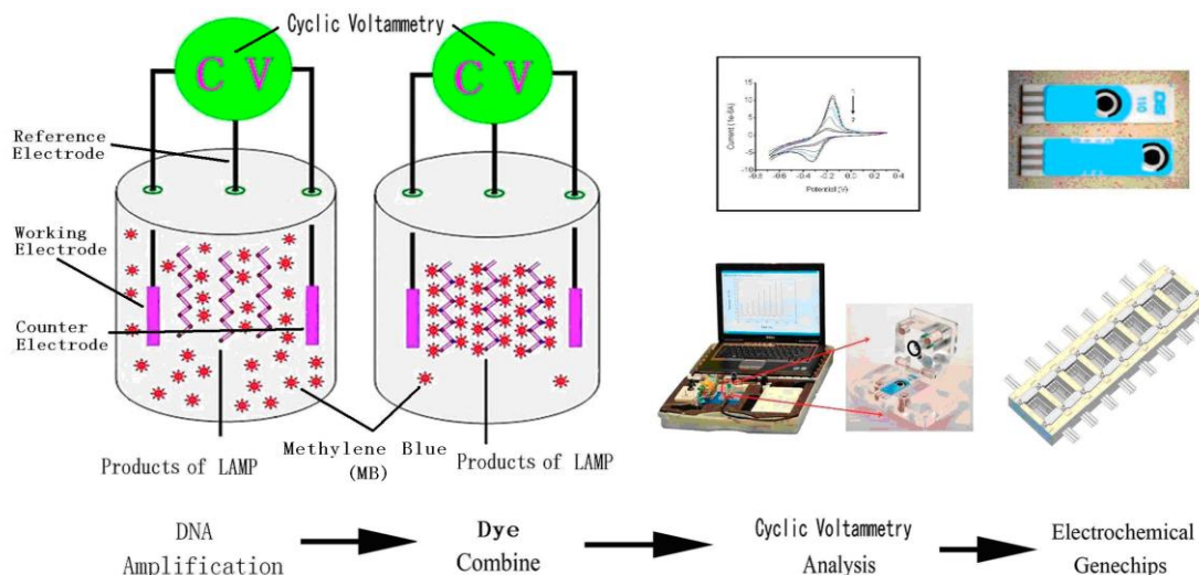
Figure 1. The scheme of the DNA electrochemical detection on the microfluidic gene chip
