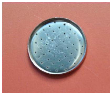
b. positive pan with small holes
