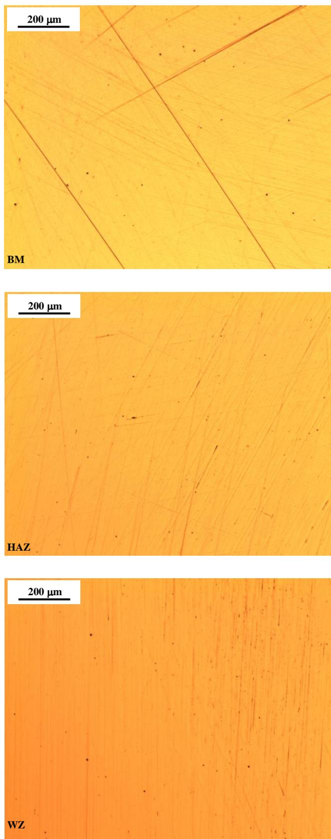
**Figure 2.** Surfaces of BZ, HAZ and WZ of Alloy 59 after OCP tests in polluted phosphoric acid at 80 °C.
