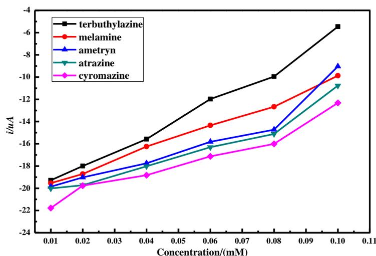
**Figure 8.** Response current of DPV with the MIP modified sensor for structural analogues different compounds. Each value represents the average of three independent measurements.
