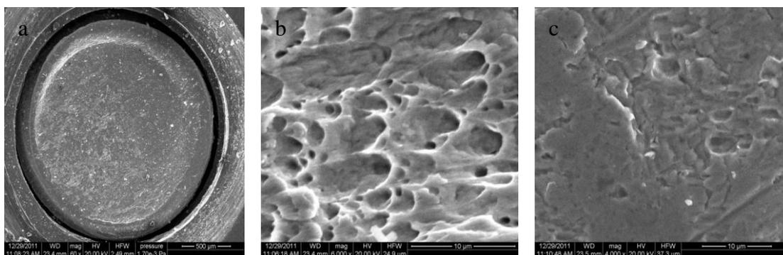
**Figure 5.** SEM images of (a) molecularly imprinted gold electrode surface (magnification 60 $\times$ ), (b) MIP electrode (magnification 6000 $\times$ ), (c) NIP electrode (magnification 4000 $\times$ ).
