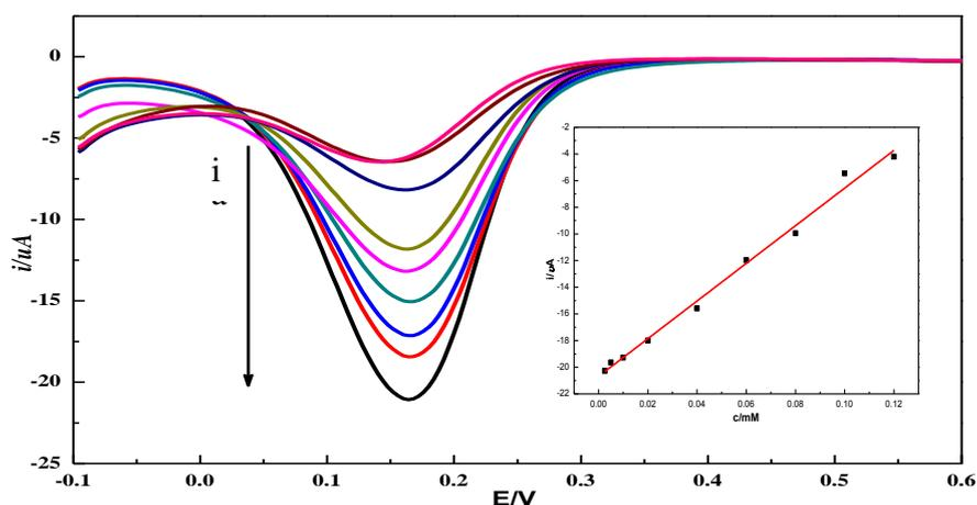
**Figure 9.** DPV graph of TBA at a concentration range of  $2.50 \times 10^{-4}$  mmol/L~0.12 mmol/L (a-i) on the surface of the MIP-modified electrode. Inset figure is a calibration curve.
