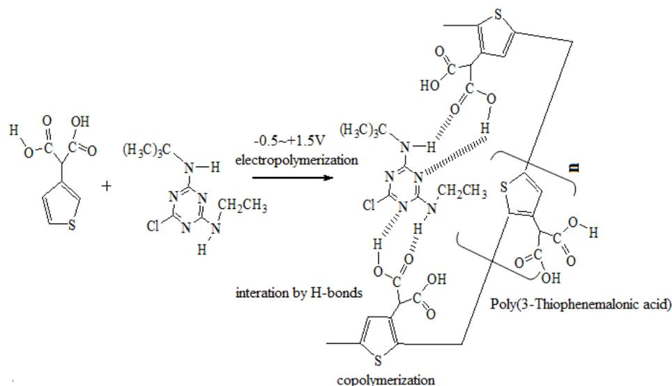
**Figure 1.** Schematic representation of poly (3-TMA) copolymerization after the establishment of H-bonds between TBA and 3-TMA in a prepolymerization complex.
