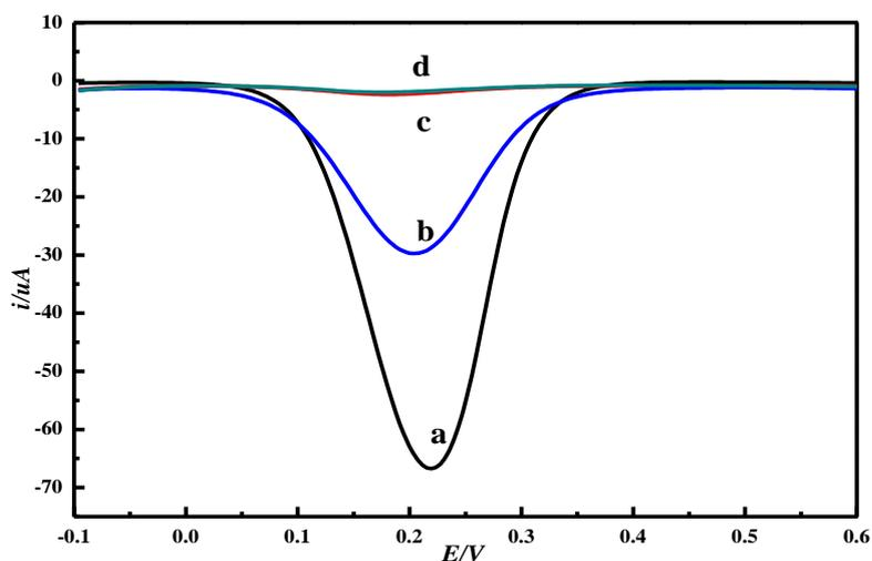
**Figure 4.** DPV graph of four kinds of gold electrodes. a) bare gold electrode, b) MIP-modified gold electrode after removal of the imprinted molecules of TBA, c) MIP modified gold electrode before the removal of the imprinted molecules of TBA, d) NIP modified gold electrode. Instrumental parameters: init E (V)=-0.1, final E (V)=0.6, amplitude (V)=0.05, Pulse Width (s)=0.2, Pulse Period (s)=0.5.
