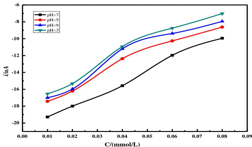
**Figure 6.** The effect of different PH value on oxidation peak current
